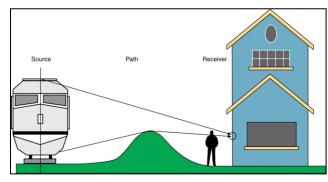
Noise impact assessments are based on applicable FTA and Federal Railroad Administration (FRA) models, and are assessed using the source-pathreceiver framework. Some of the key components of a noise impact assessment include:
