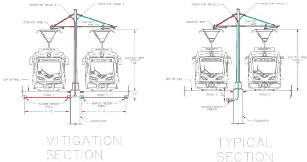
**Figure 1 Layout of Power Supply Wires in the Mitigation Section**
