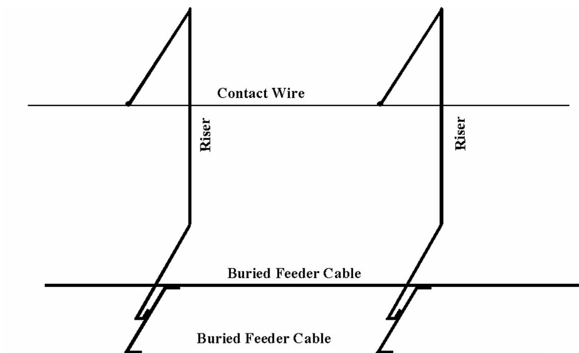
**Figure 2 Connections between Buried Cables and Contact Wire**
