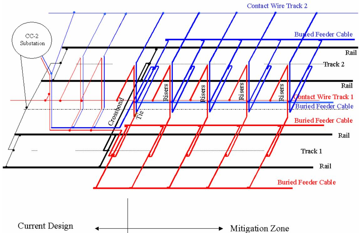
**Figure 3 Layout of Electrical Wires**
