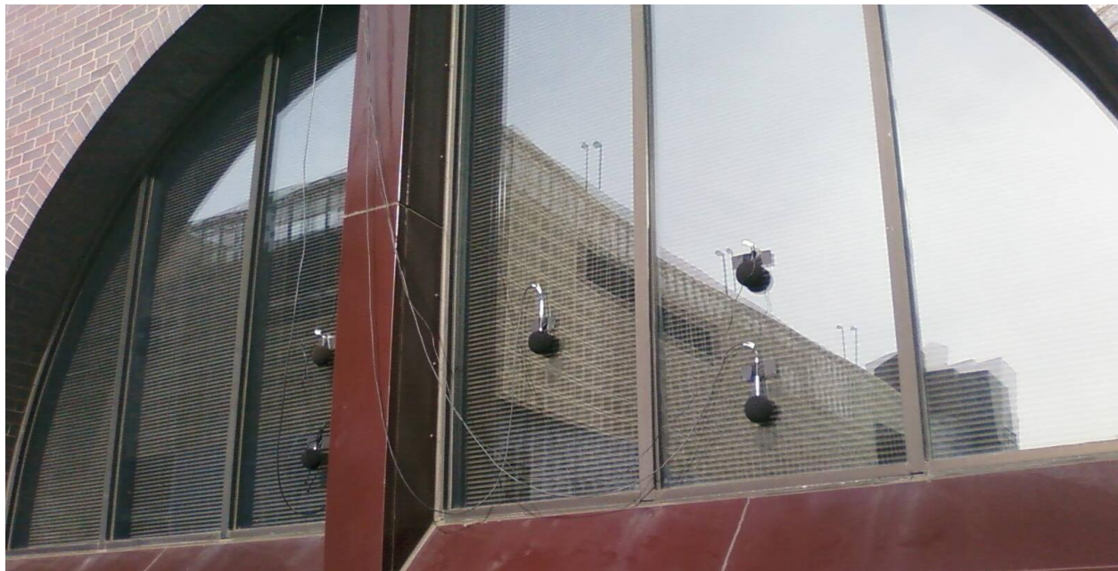
Figure 1 – Studio MMW exterior microphone locations
