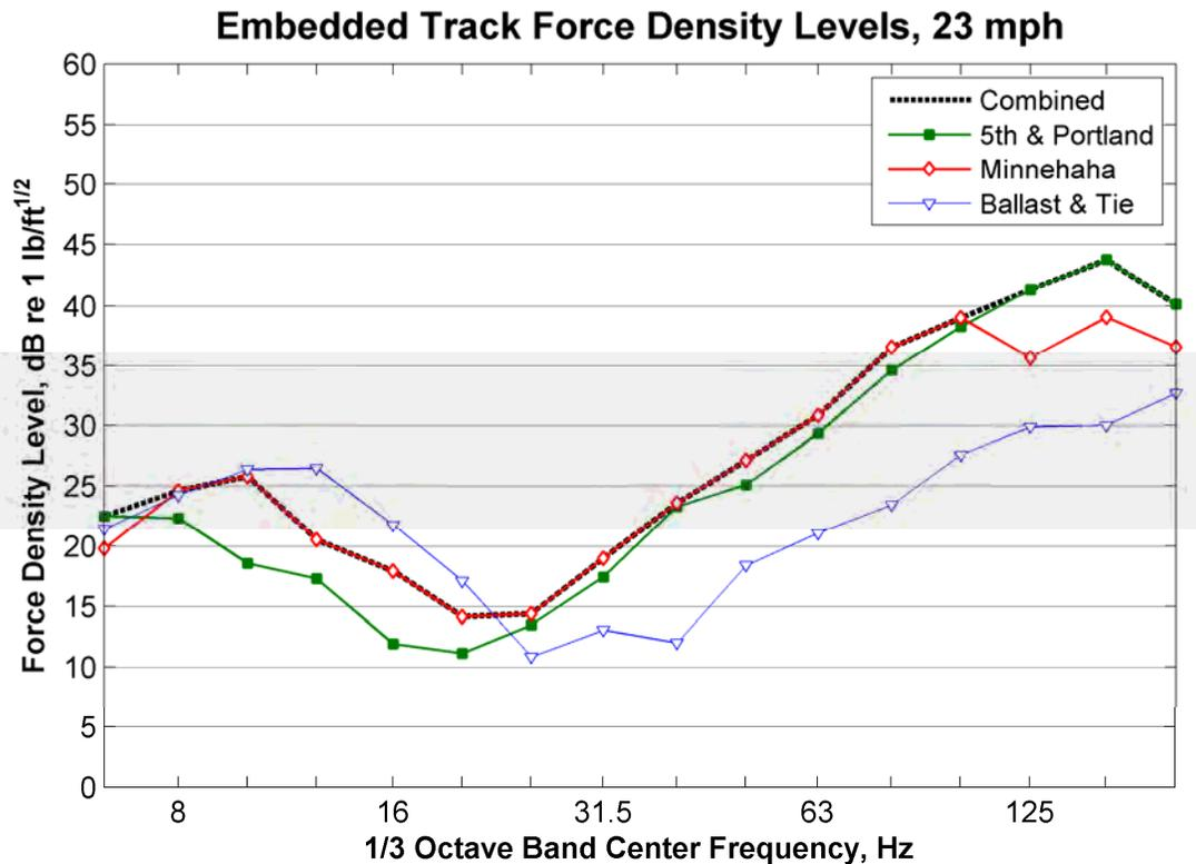
**Figure 35: Measured and Composite FDL at 23 mph, Embedded Track**
