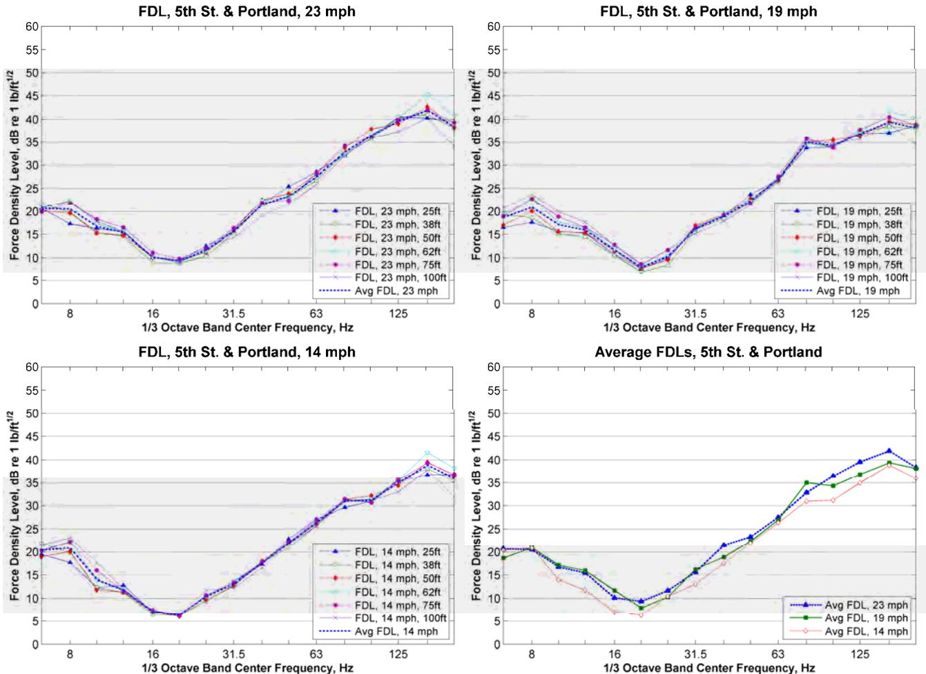
**Figure 25: Force Density Levels, 5<sup>th</sup> Street and Portland Avenue Embedded Track**
