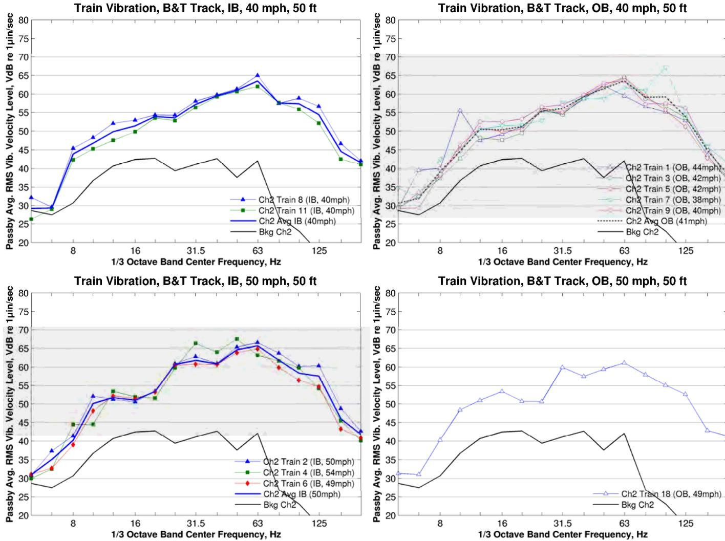
**Figure 182: Vibration Spectra, Ballast & Tie Track, 50 ft, 40 and 50 mph**
