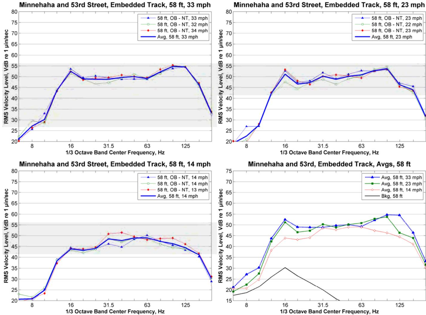
**Figure 198: Train Vibration, Minnehaha and 53<sup>rd</sup> Street, 58 ft from Track Centerline**
