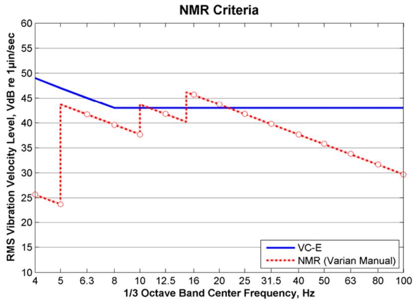
**Figure 3: NMR Criteria Compared to VC-E Curve**
