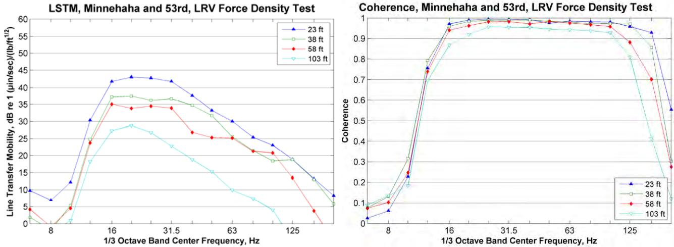
Figure 27: Line-Source Transfer Mobility, LRV FDL Test, Minnehaha & 53<sup>rd</sup> Street
