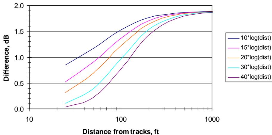
**Figure 40: Expected Vibration Difference for a 3-Car Train Compared to a 2-Car Train**
