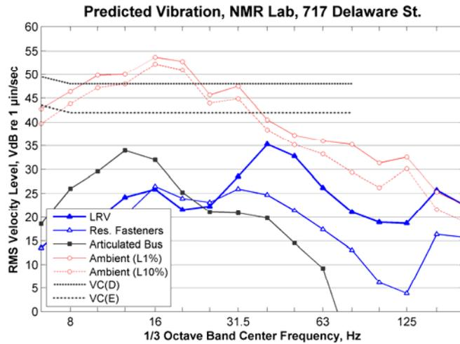
**Figure 82: Predicted Vibration in NMR Lab, 717 Delaware Street**
