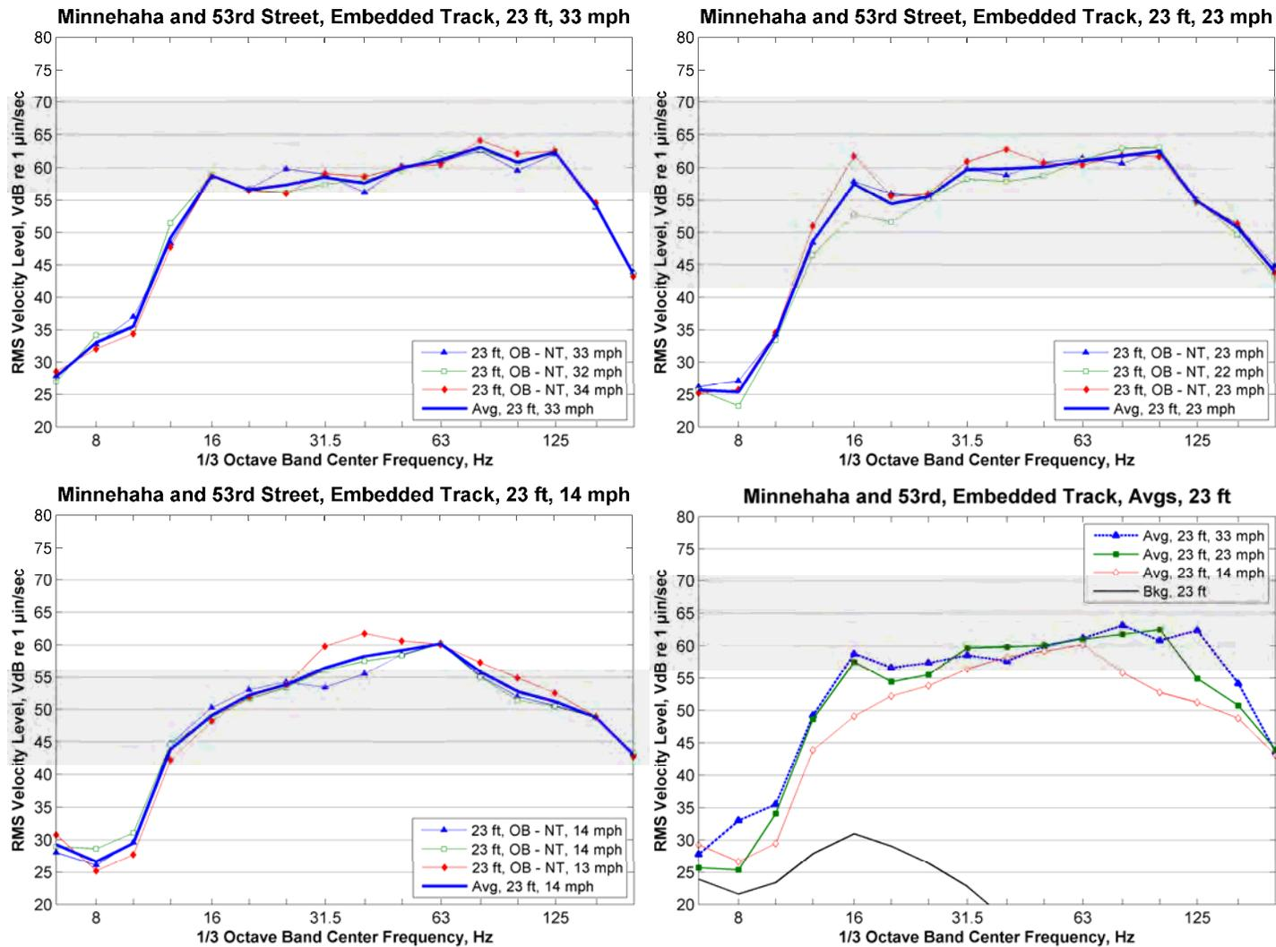
Figure 196: Train Vibration, Minnehaha and 53<sup>rd</sup> Street, 23 ft from Track Centerline
