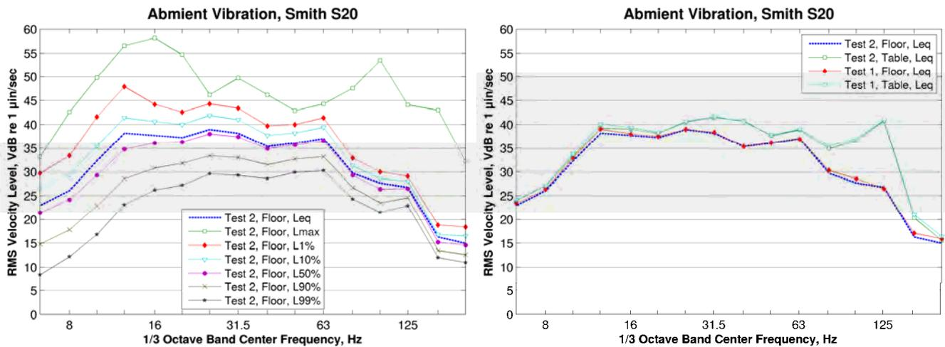
**Figure 77: Vibration Spectra of Ambient Vibration, Room Smith S20**
