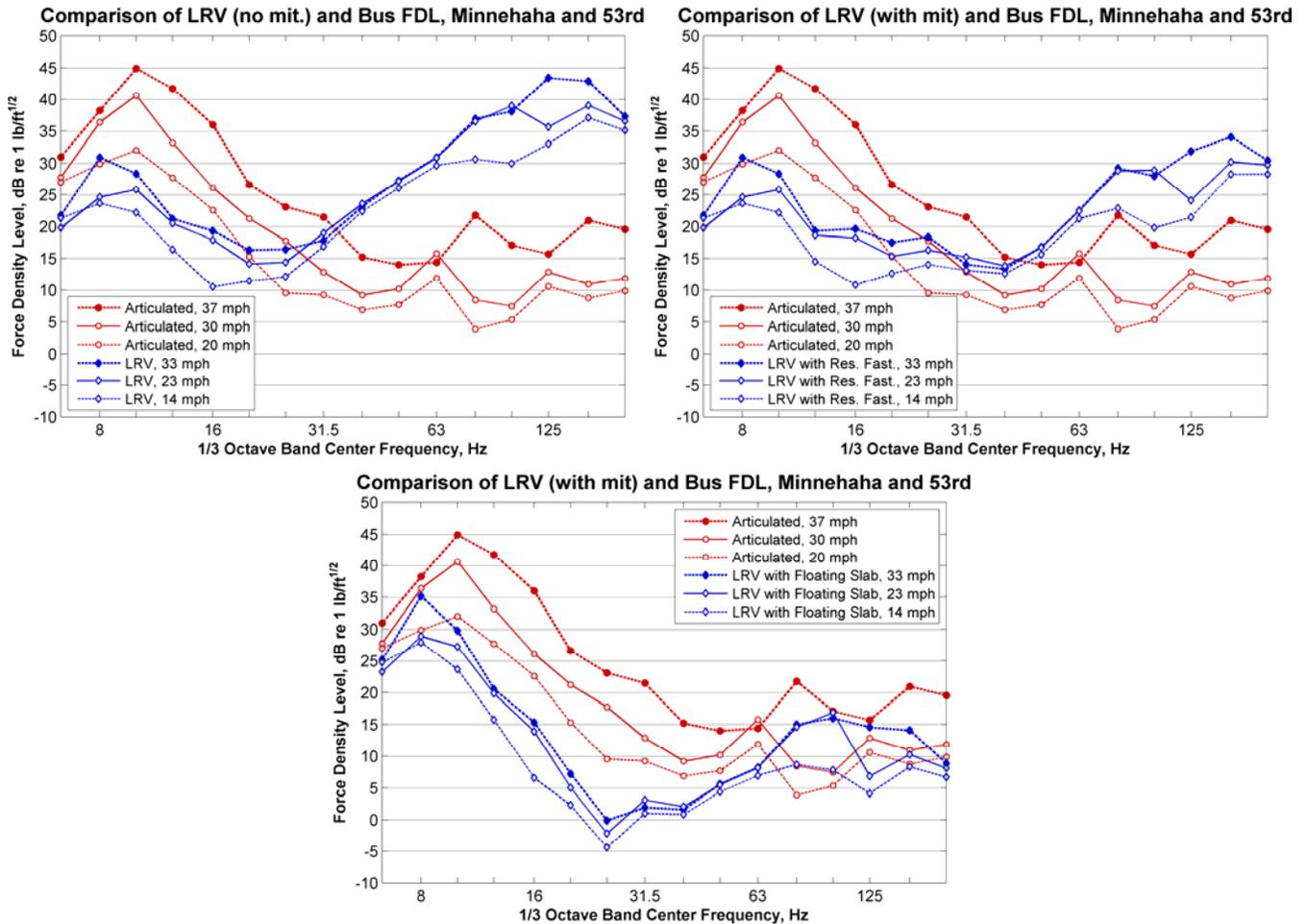
**Figure 39: Comparison of Bus and LRV Force Density Curves, Minnehaha and 53<sup>rd</sup>**
