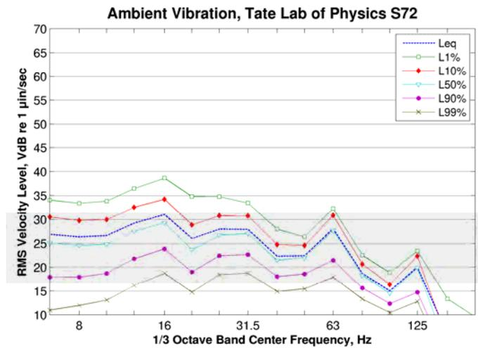
**Figure 138: Ambient Vibration Spectrum inside the Tate Lab of Physics**
