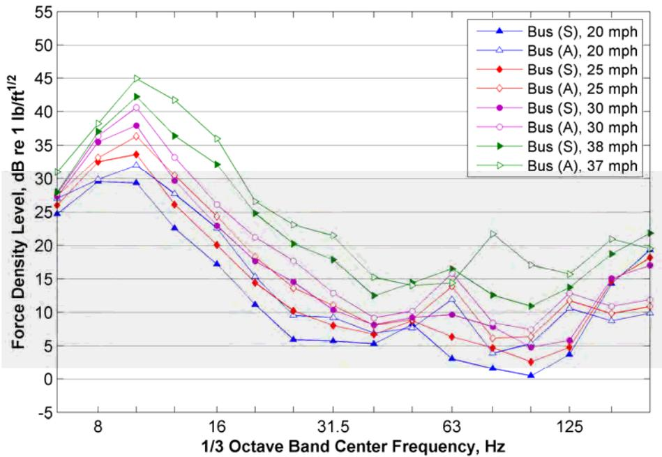
Figure 37: Bus FDL Curves Levels for Predicting L<sub>max</sub>
