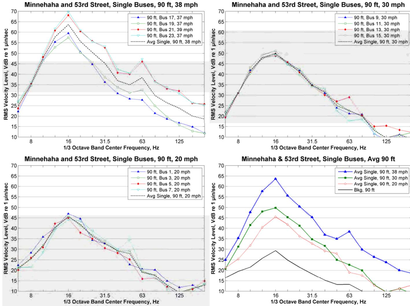
**Figure 206: Single Bus Vibration, Minnehaha and 53<sup>rd</sup> Street, 90 ft from Roadway Centerline**
