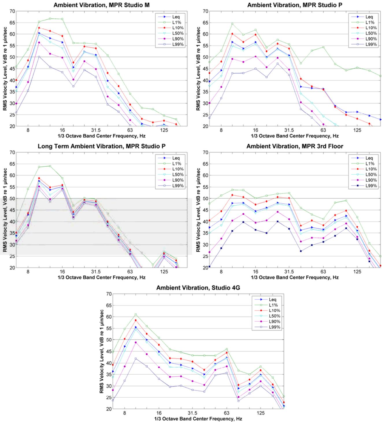
**Figure 170: Ambient Vibration Measurements in Original MPR Building**
