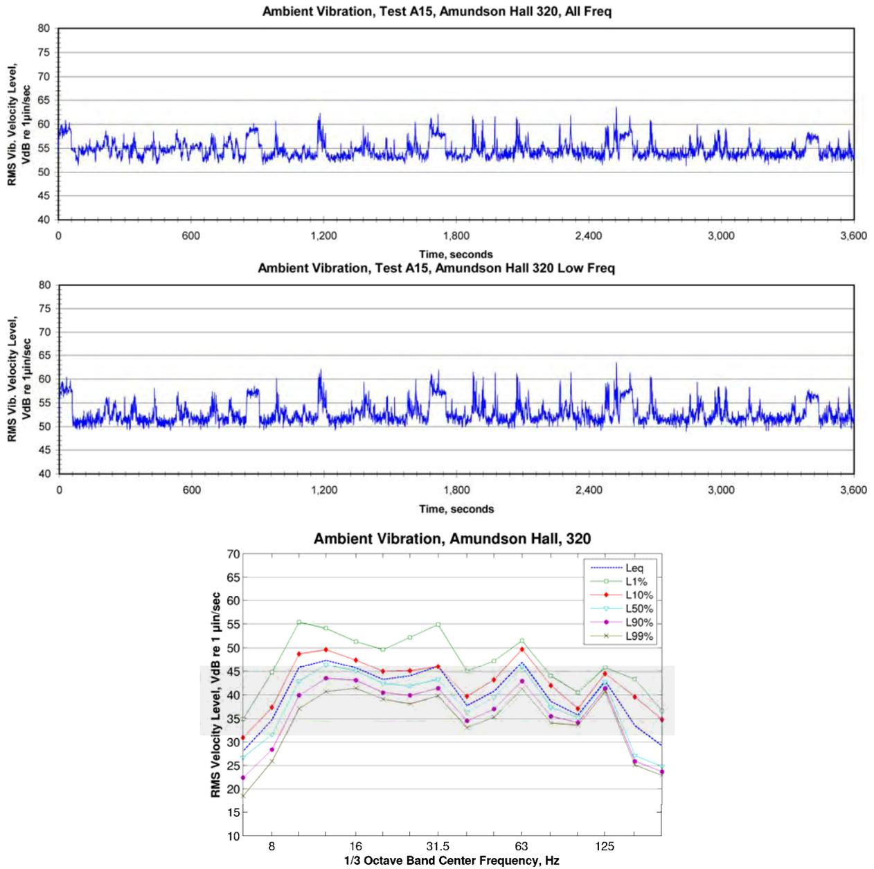
**Figure 131: Ambient Vibration Spectrum inside Room 320 at Amundson Hall**
