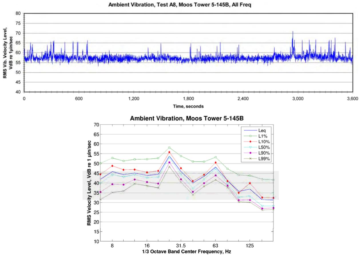
**Figure 103: Ambient Vibration inside Room 5-145B at Moos Tower**
