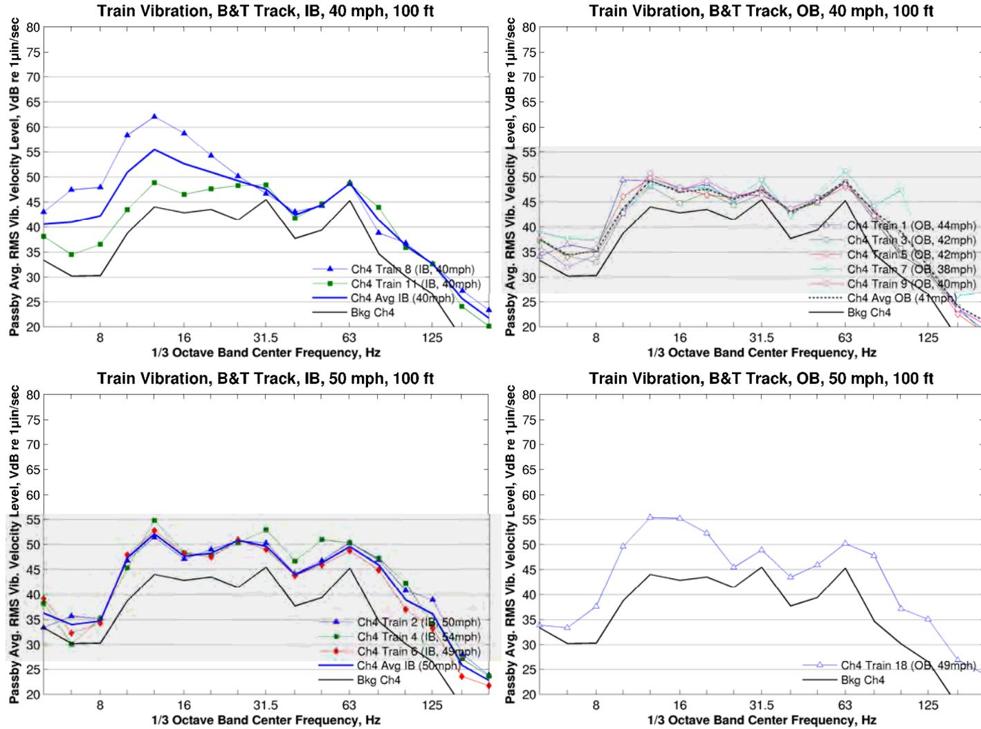
**Figure 186: Vibration Spectra, Ballast & Tie Track, 100 ft, 40 and 50 mph**
