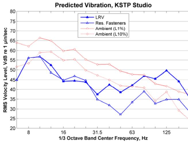
**Figure 154: Predicted Train Vibration inside KSTP Studio**
