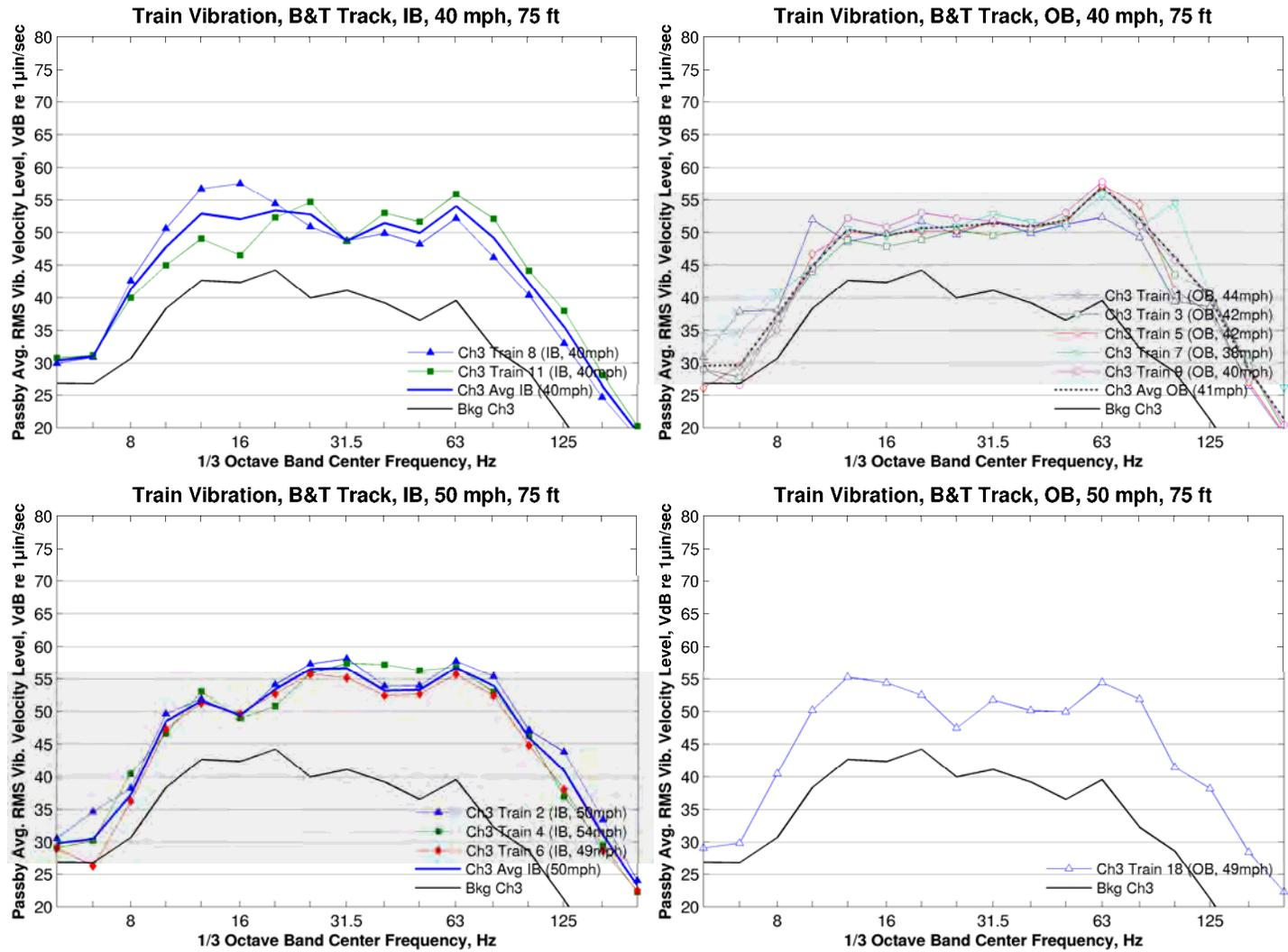
Figure 184: Vibration Spectra, Ballast & Tie Track, 75 ft, 40 and 50 mph
