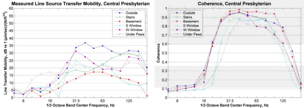
**Figure 161: Measured Line Source Transfer Mobility, Central Presbyterian Church**
