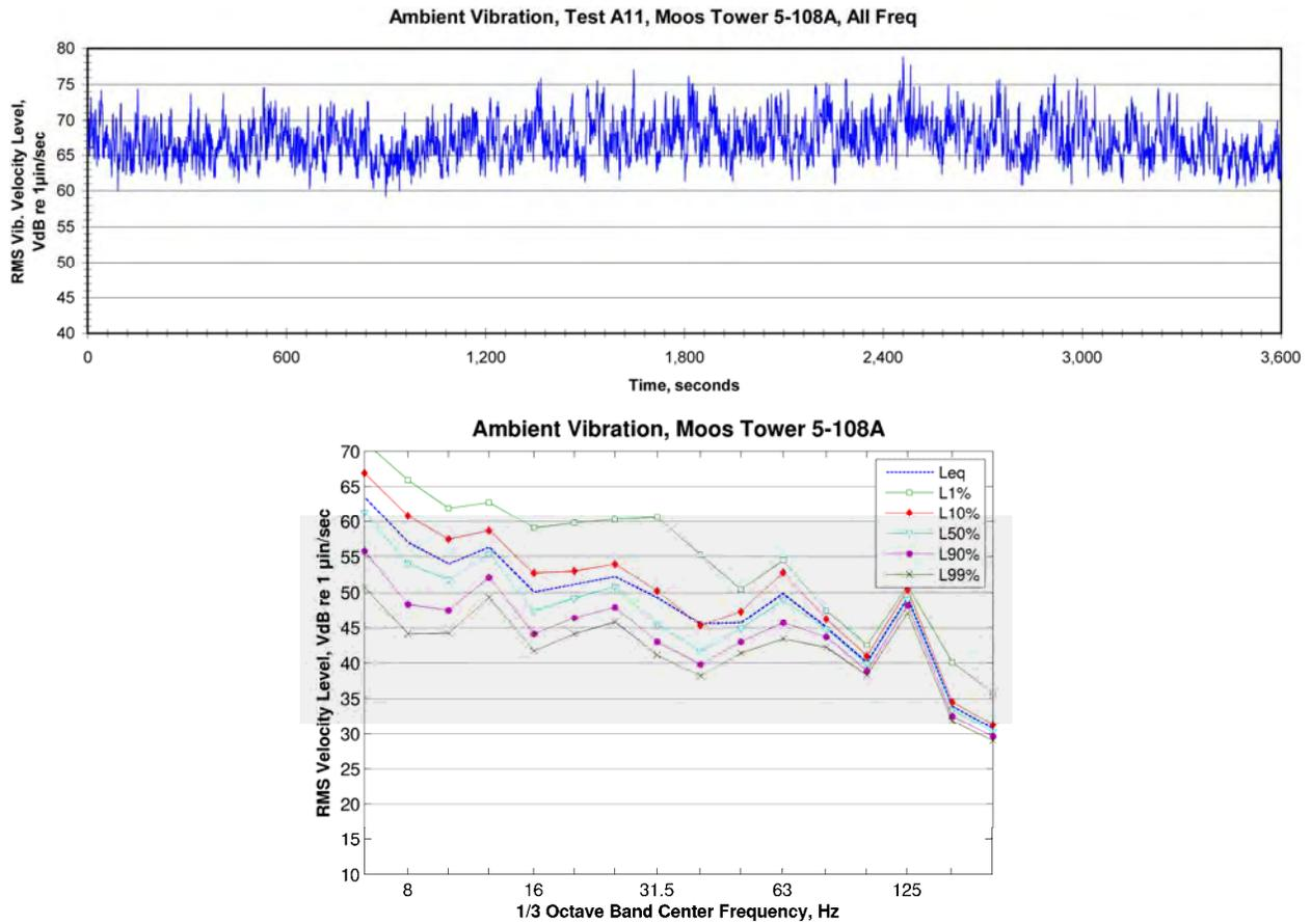
**Figure 114: Ambient Vibration inside Room 5-108A at Moos Tower**
