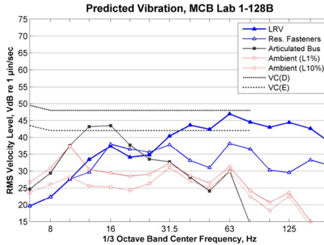
**Figure 112: Predicted Vibration inside Room 1-128B at the Molecular and Cellular Biology Building**
