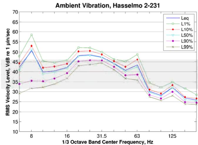
**Figure 88: Ambient Vibration inside Room 2-231 at Nils Hasselmo**
