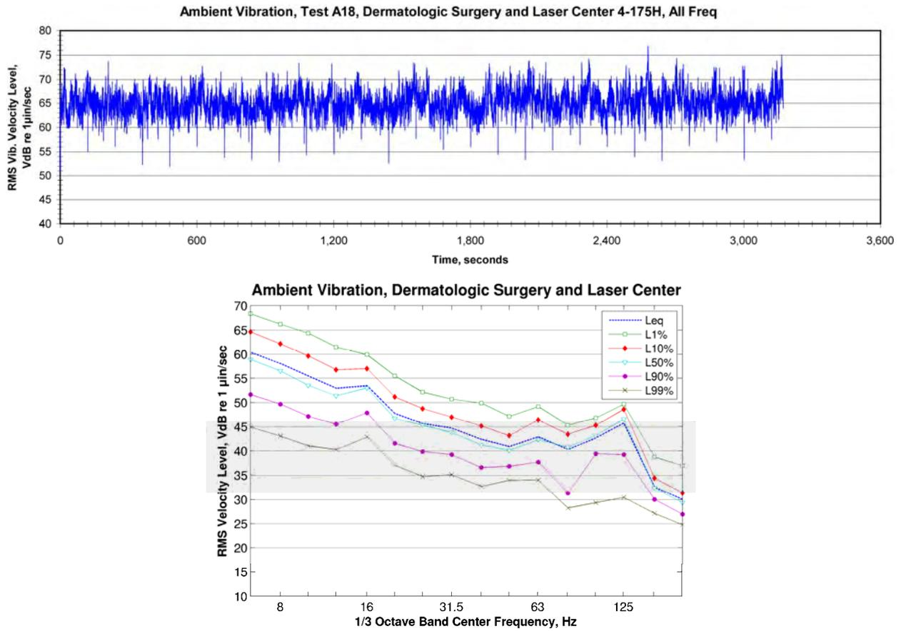
Figure 141: Ambient Vibration Spectrum inside the Dermatology Surgery and Laser Center
