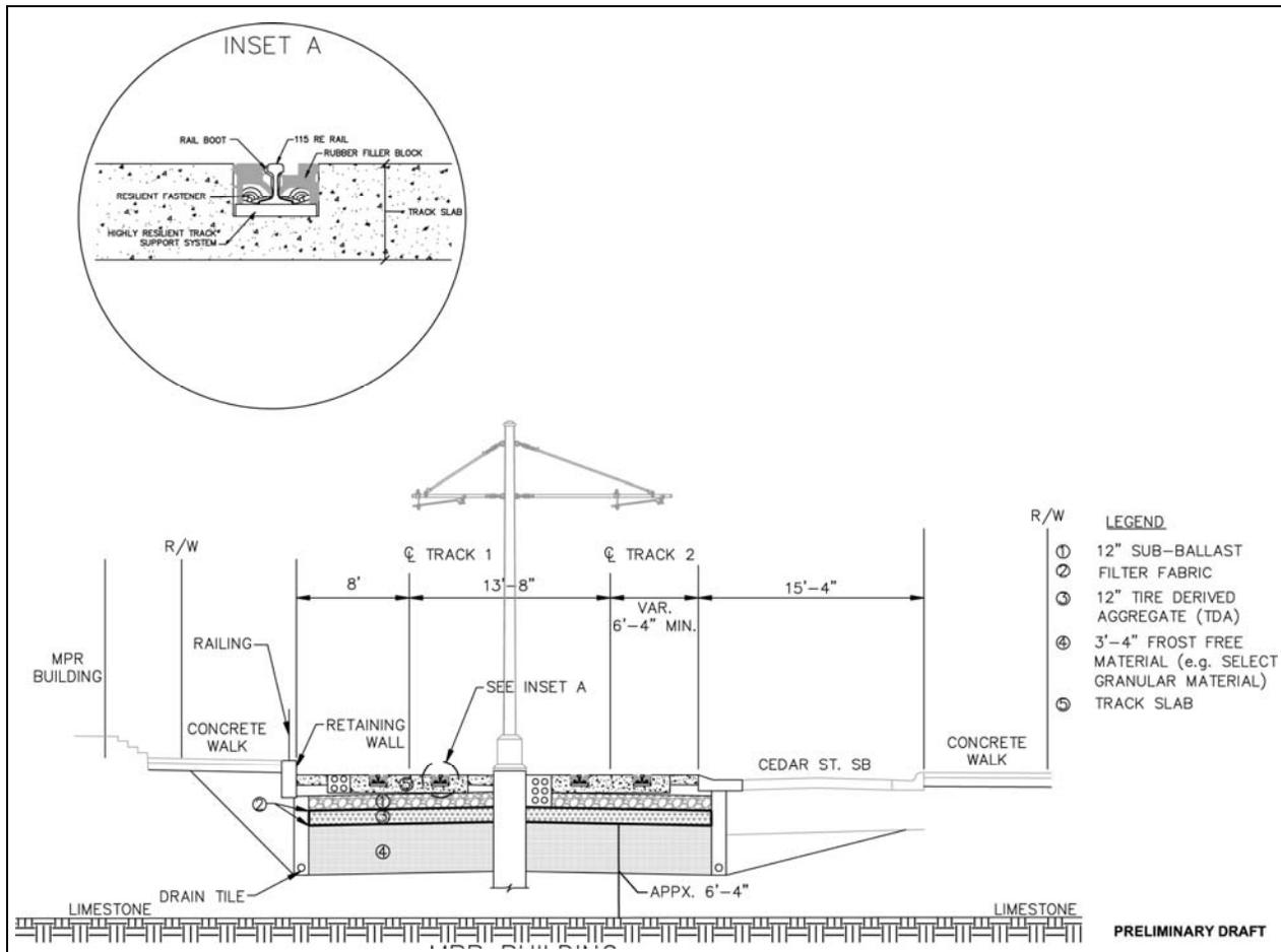
**Figure 5: Concept for Using Tire Derived Aggregate for Vibration Isolation of Embedded Track**
