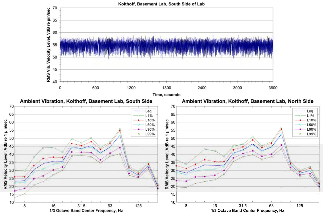
**Figure 70: Ambient Vibration Measured in Kolthoff Basement Lab**
