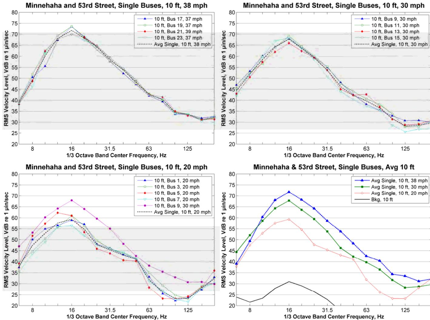
Figure 200: Single Bus Vibration, Minnehaha and 53<sup>rd</sup> Street, 10 ft from Roadway Centerline
