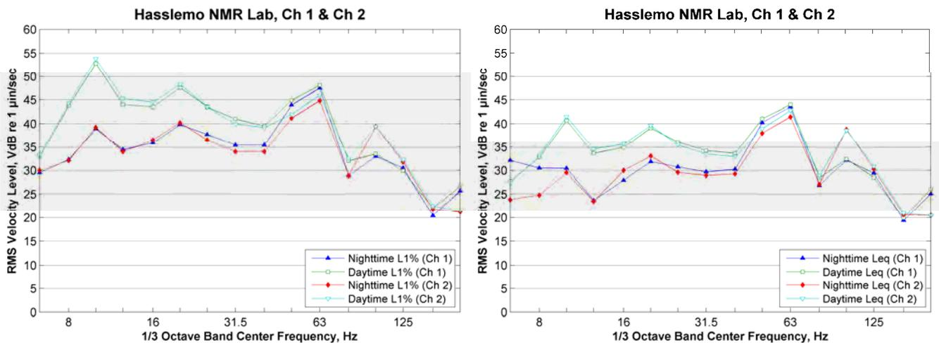
**Figure 48: Comparison of Channel 1 and Channel 2 Ambient Vibration, Hasselmo NMR Lab**
