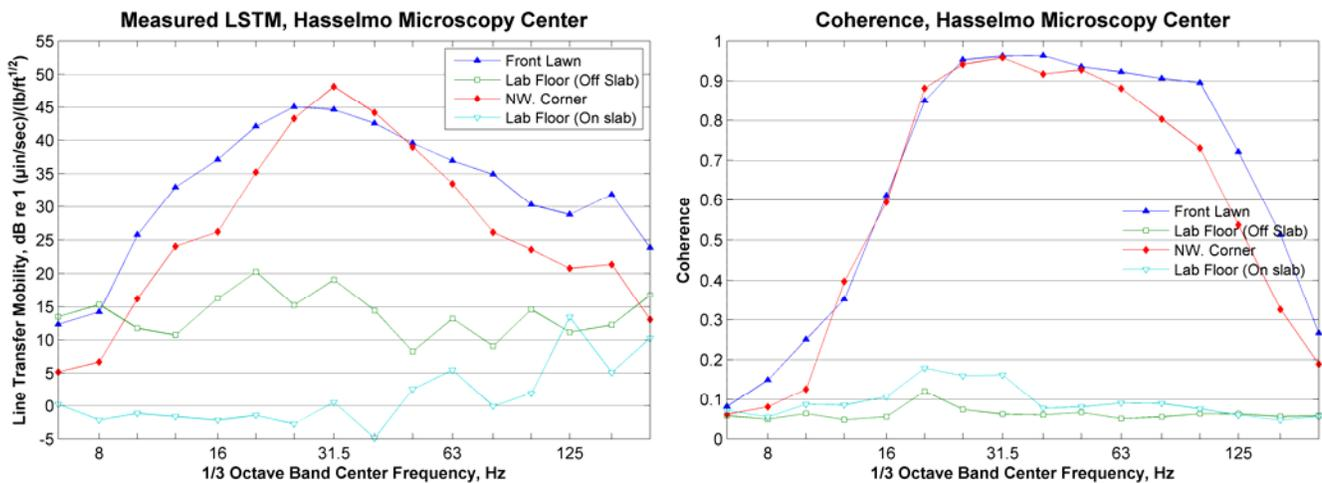
**Figure 56: Measured Line Source Transfer Mobility, Hasselmo Microscopy Center**
