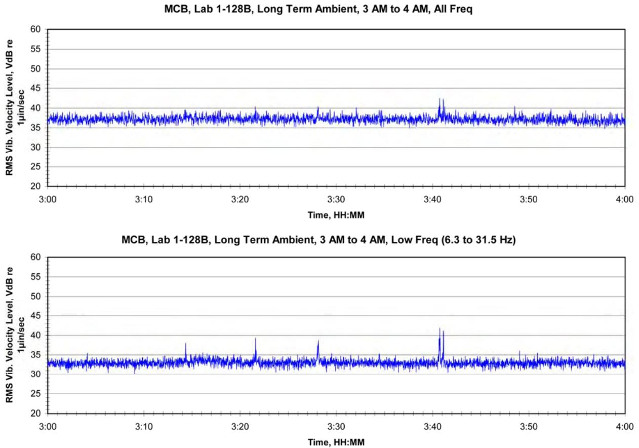
**Figure 110: Time History of Vibration inside Room 1-128B at MCB, Typical Night Time**
