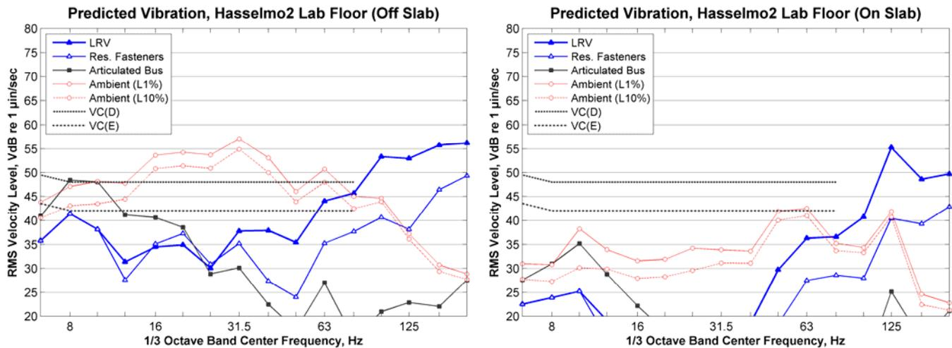
**Figure 57: Predicted Train Vibration inside Hasselmo Microscopy Center**
