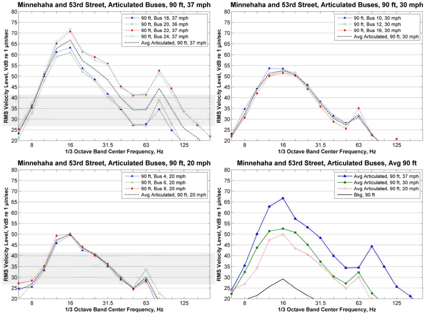
**Figure 207: Articulated Bus Vibration, Minnehaha and 53<sup>rd</sup> Street, 90 ft from Roadway Centerline**
