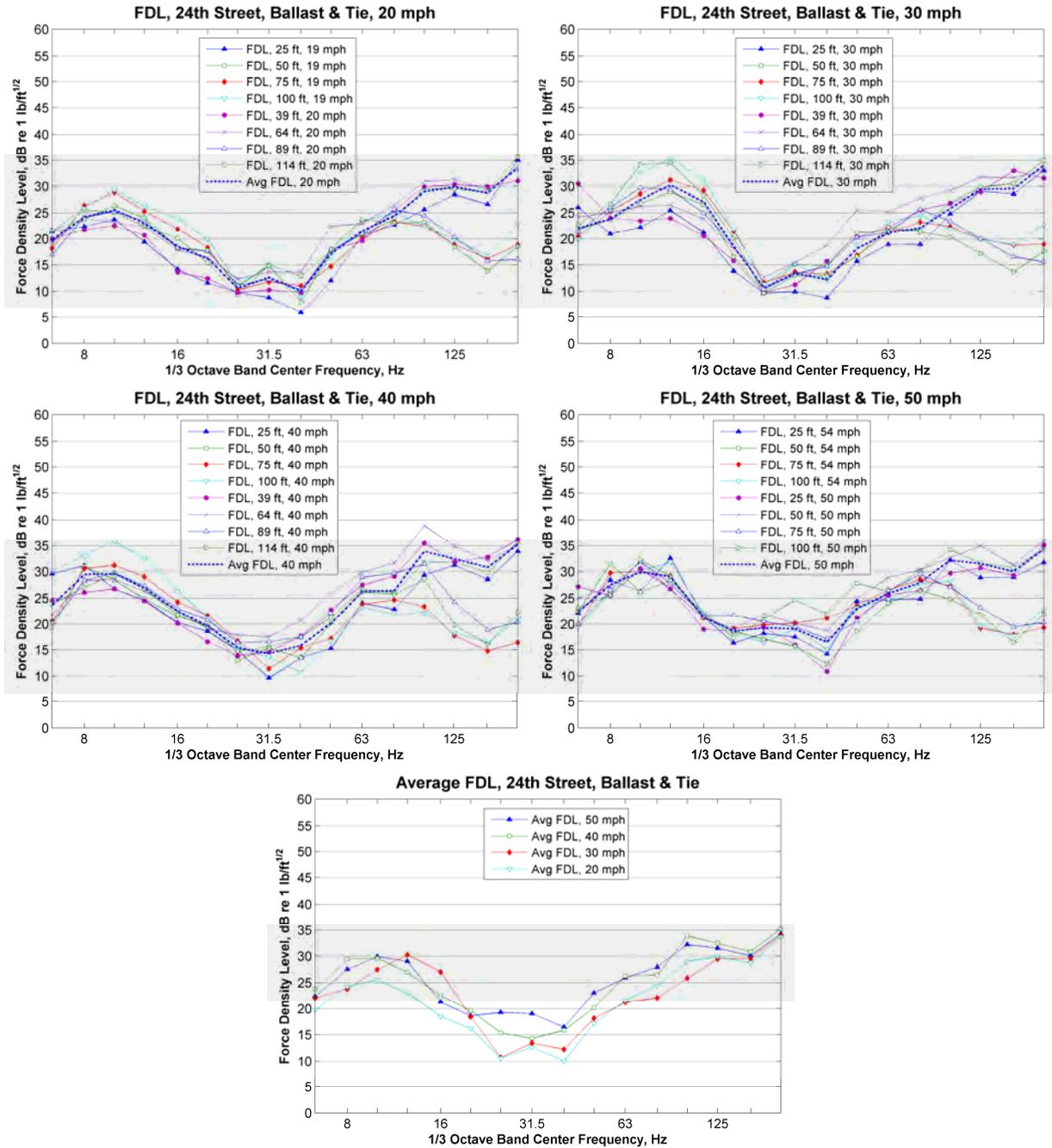
**Figure 13: Force Density Levels, 24<sup>th</sup> FDL Test Site (Ballast and Tie Track)**
