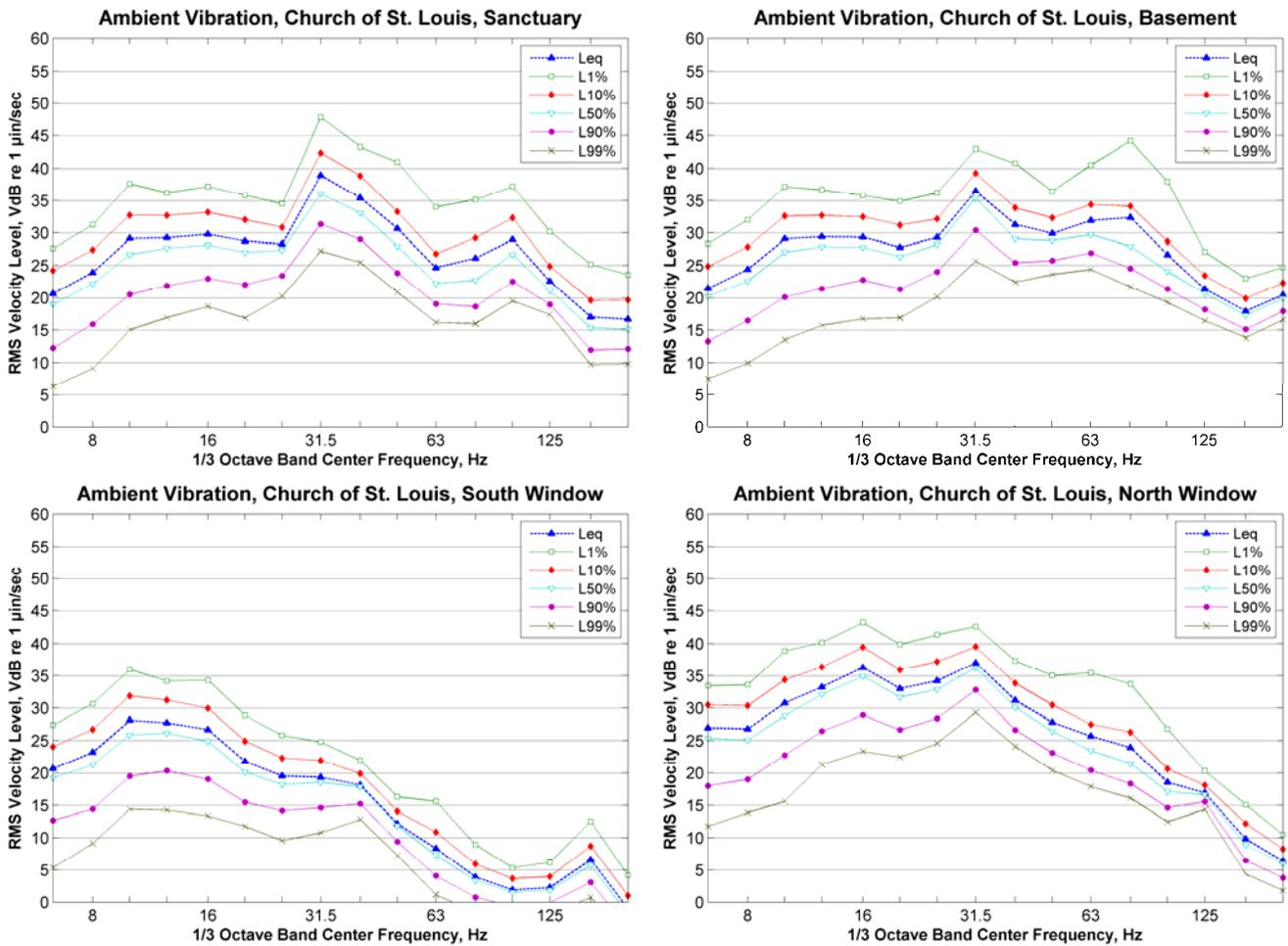
Figure 159: Ambient Vibration at Indoor LSTM Measurement Positions, Church of St. Louis
