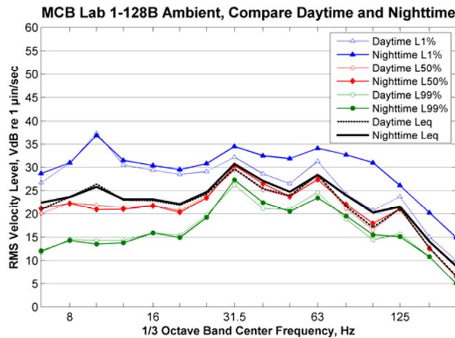
**Figure 111: Ambient Vibration Spectrum inside Room 1-128B at MCB**
