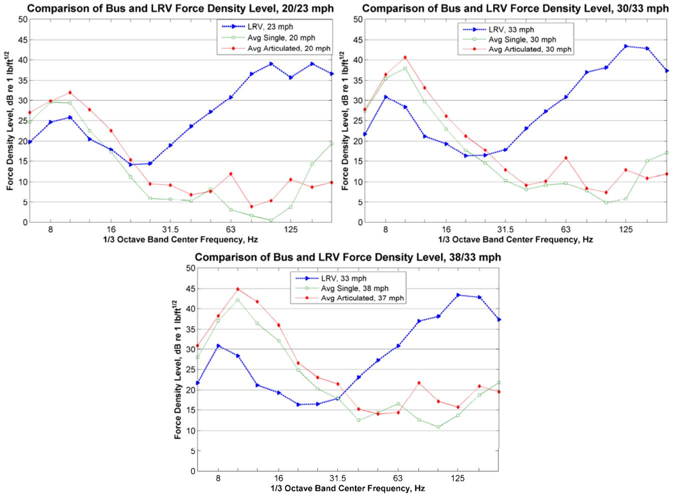
**Figure 38: Comparison of Bus and LRV FDL Curves**
