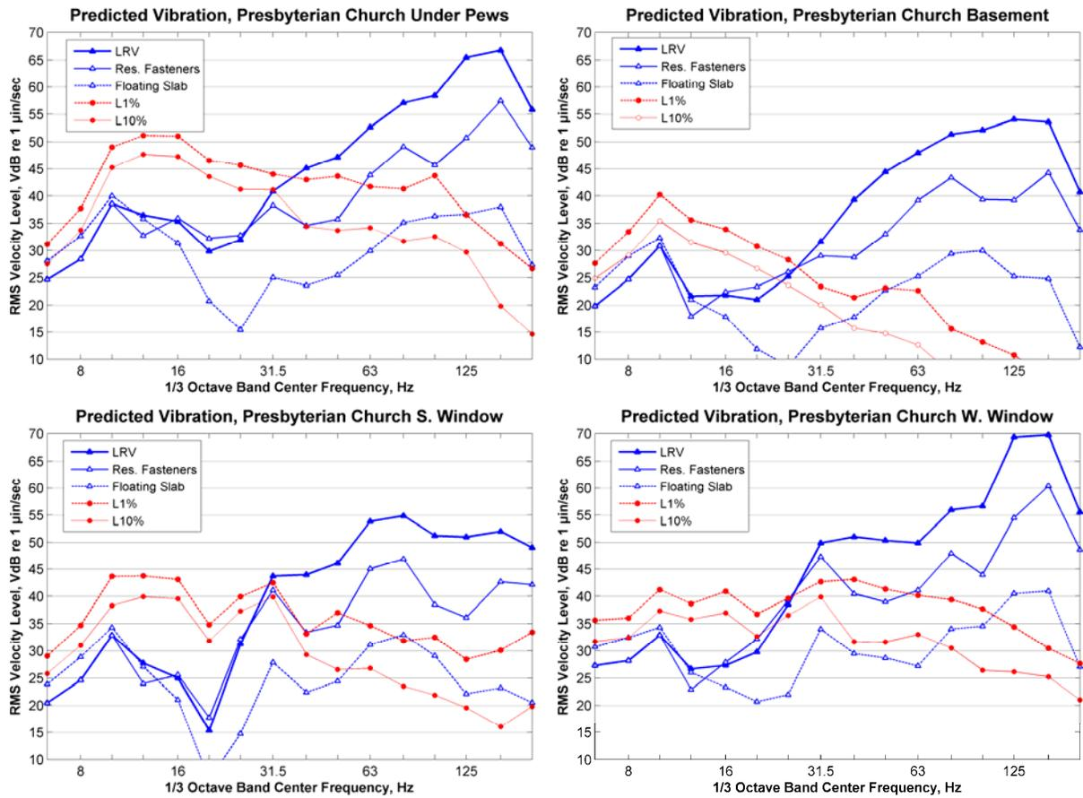
**Figure 163: Predicted LRT Vibration, Central Presbyterian Church**
