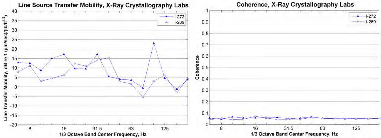
**Figure 53: Measured Line Source Transfer Mobility, Hasselmo Rooms 1-272 and 1-269**
