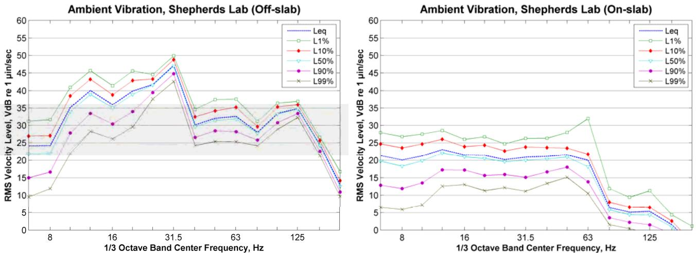
**Figure 60: Ambient Vibration in Shepherd Labs Microscopy Center**
