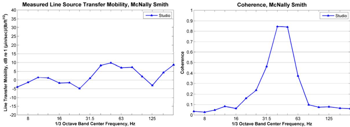
**Figure 165: Measured LSTM & Coherence at McNally Smith Performance Center**
