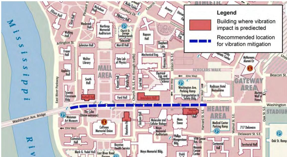
Figure 44: Predicted Vibration Impact on U of M Campus and Location of Vibration Mitigation
