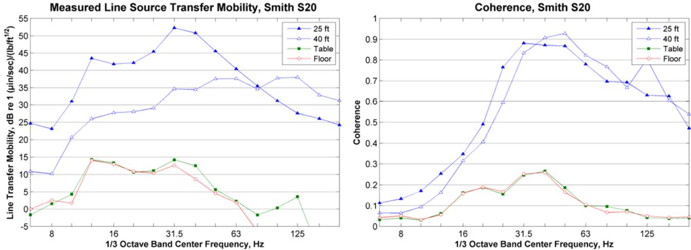
**Figure 78: Measured Line Source Transfer Mobility, Smith S20**
