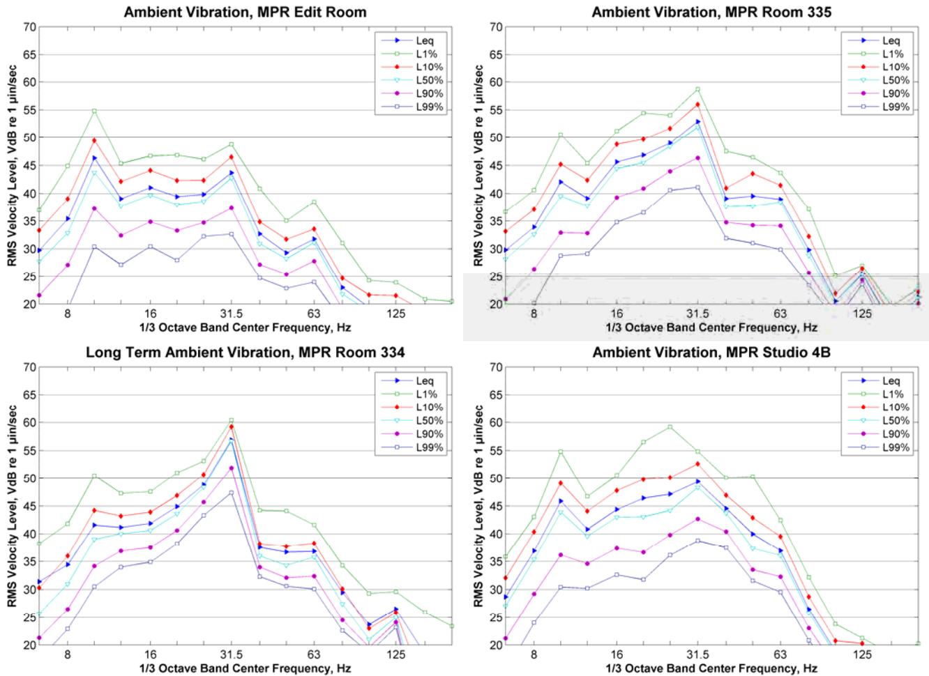
**Figure 171: Ambient Vibration Measurements in New MPR Building**
