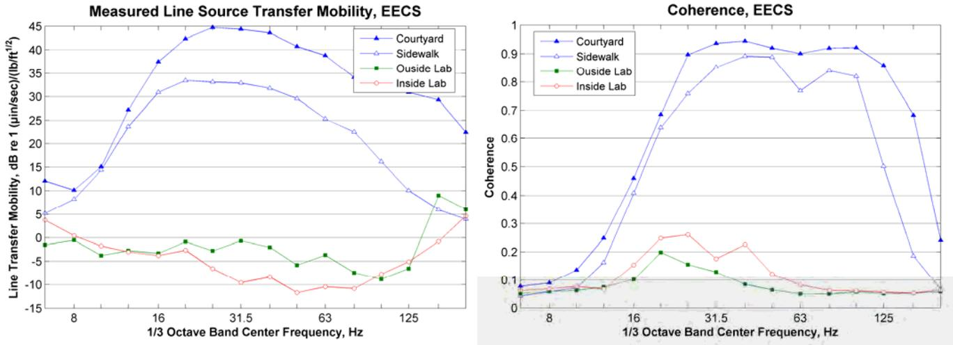
**Figure 63: Measured Line Source Transfer Mobility, EECS**
