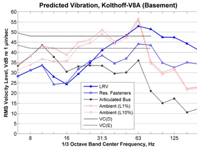
**Figure 72: Predicted Vibration and Mitigation for Prof. Blank’s Lab inside Kolthoff Hall**
