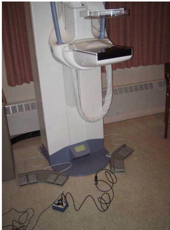
**Figure 143: Ambient Vibration Measurement on the Floor of Room M 164 at the Cancer Center**
