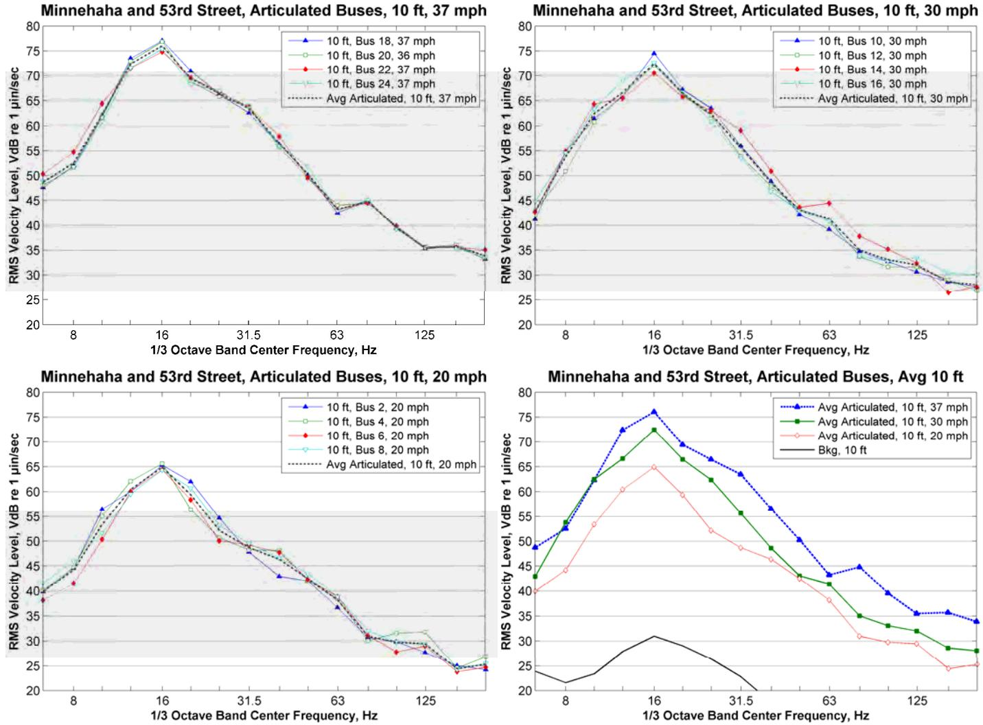
**Figure 201: Articulated Bus Vibration, Minnehaha and 53<sup>rd</sup> Street, 10 ft from Roadway Centerline**
