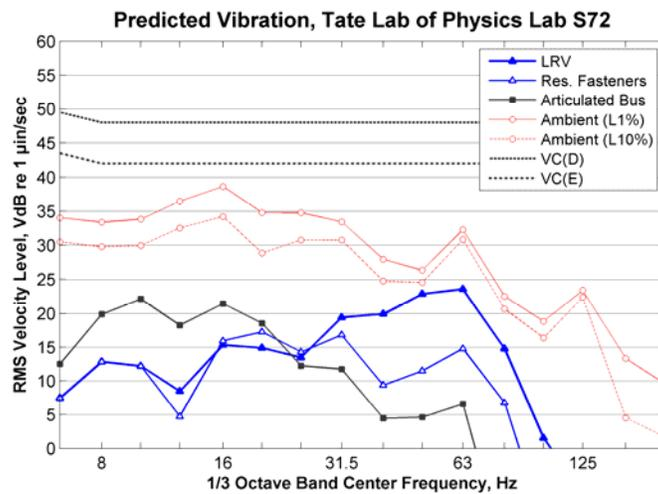
**Figure 139: Predicted Vibration inside Room S72 at the Tate Lab of Physics**
