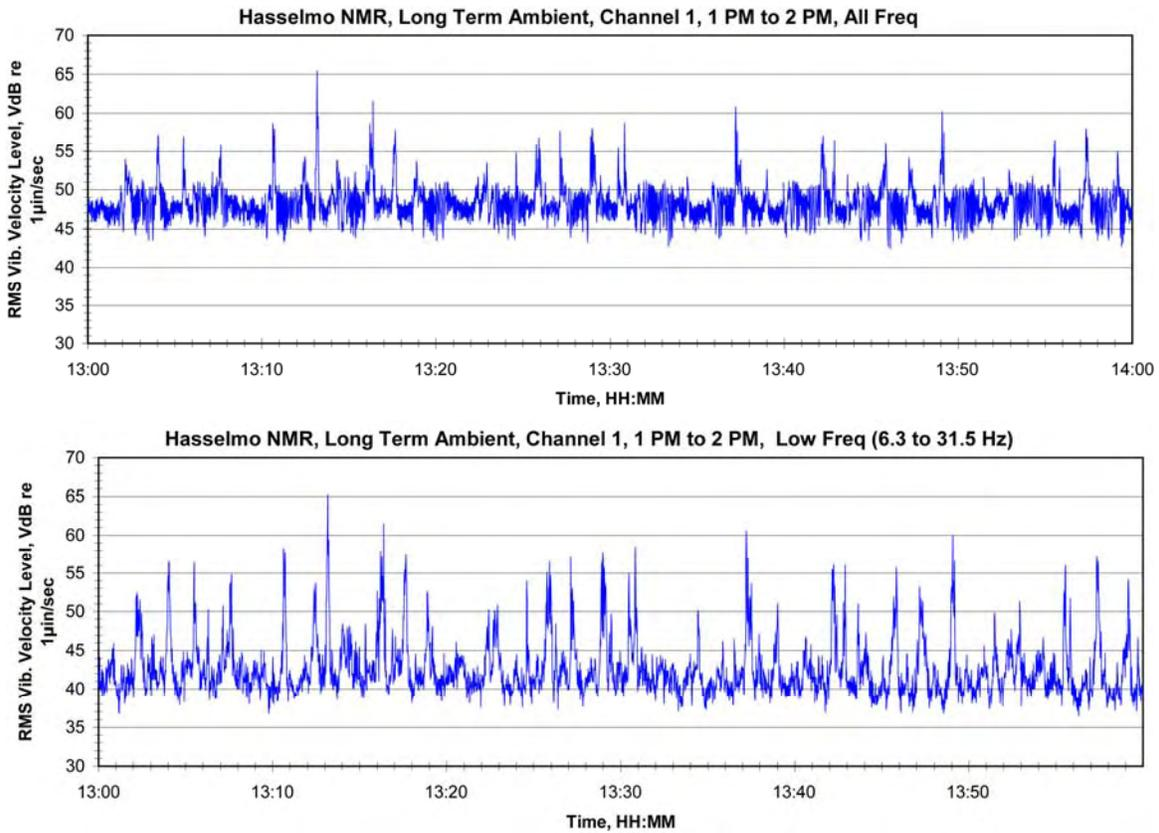
**Figure 47: Ambient Vibration in Hasselmo NMR Lab, Typical Daytime Hour**
