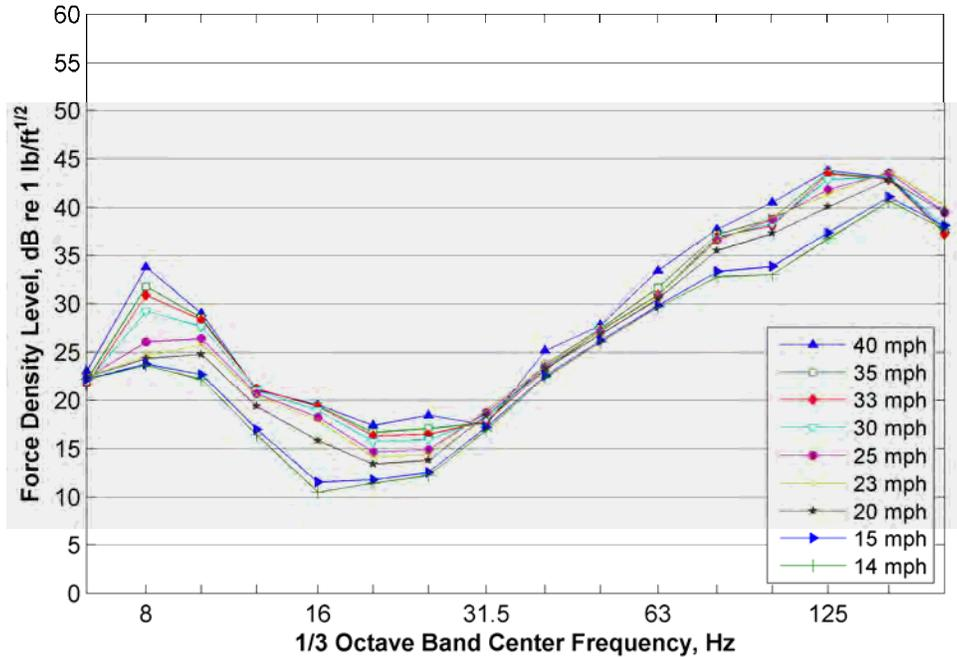
Figure 36: LRV FDL Curves Used for Predictions L<sub>max</sub>, Embedded Track
