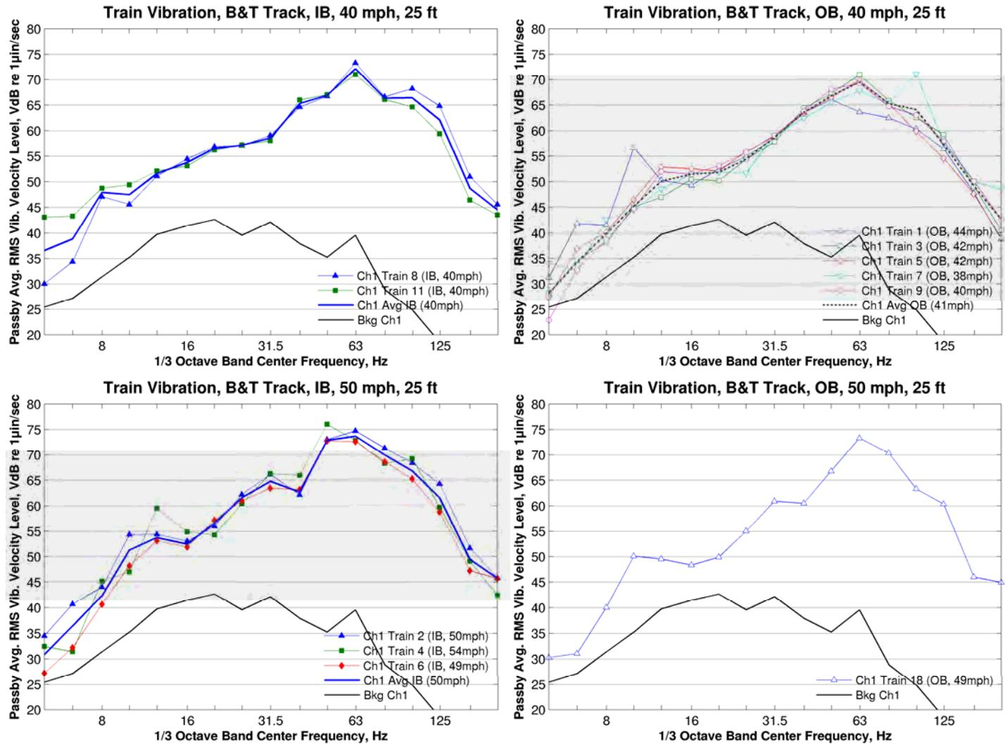
**Figure 180: Vibration Spectra, Ballast & Tie Track, 25 ft, 40 and 50 mph**
