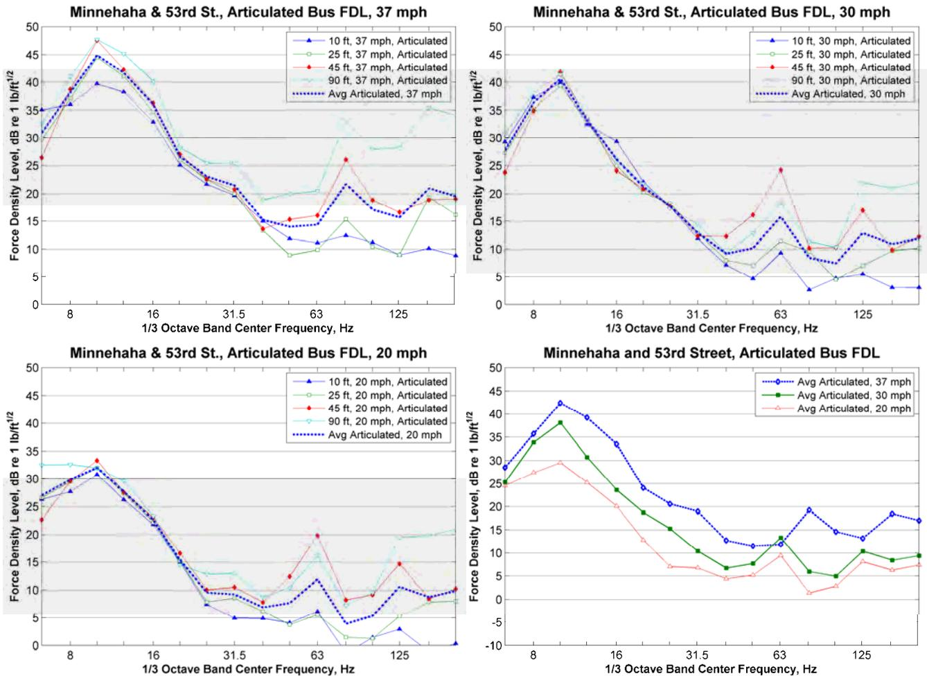
**Figure 34: Articulated Bus Force Density Levels, Minnehaha and 53<sup>rd</sup> Street**
