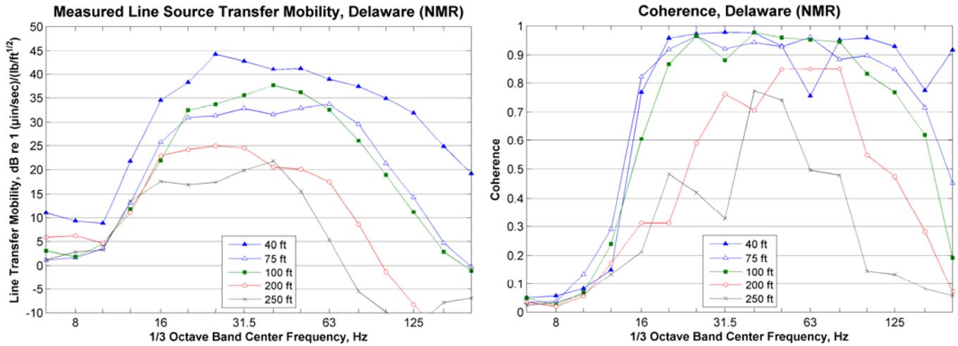
**Figure 81: Measured Line Source Transfer Mobility, Delaware (Outdoors)**
