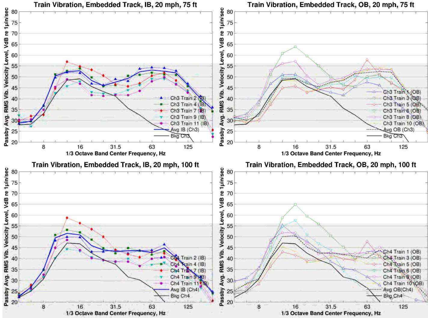
Figure 189: Vibration Spectra, 5<sup>th</sup> Street and 5<sup>th</sup> Avenue Embedded Track, 75 and 100 ft, 20 mph
