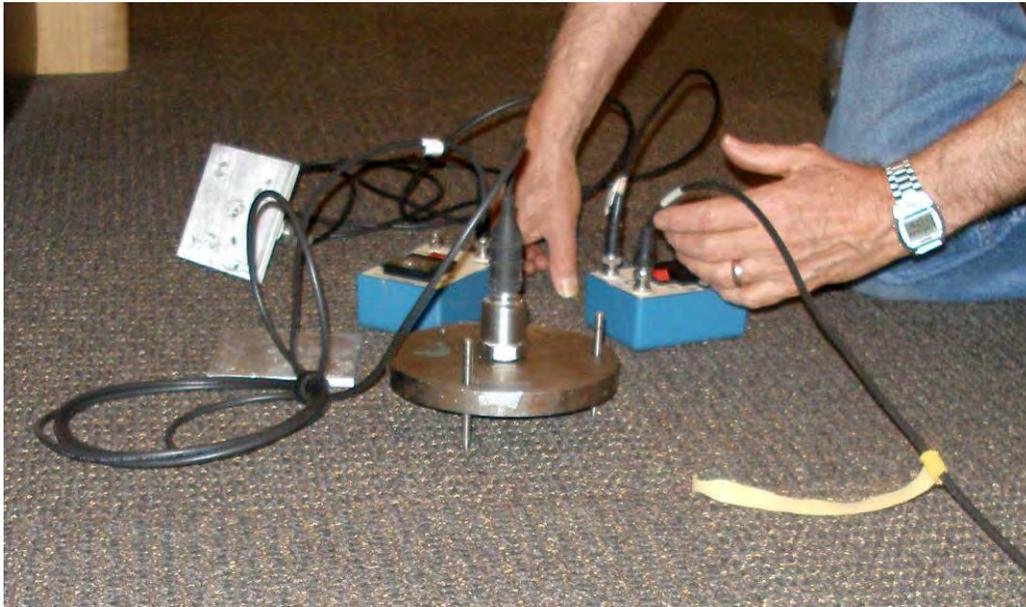
**Figure 167: Installation of Accelerometer on Carpeted Floor**
