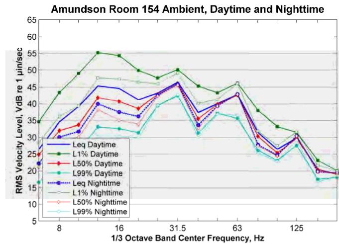
**Figure 128: Ambient Vibration Spectrum inside Room 54 at Amundson Hall**
