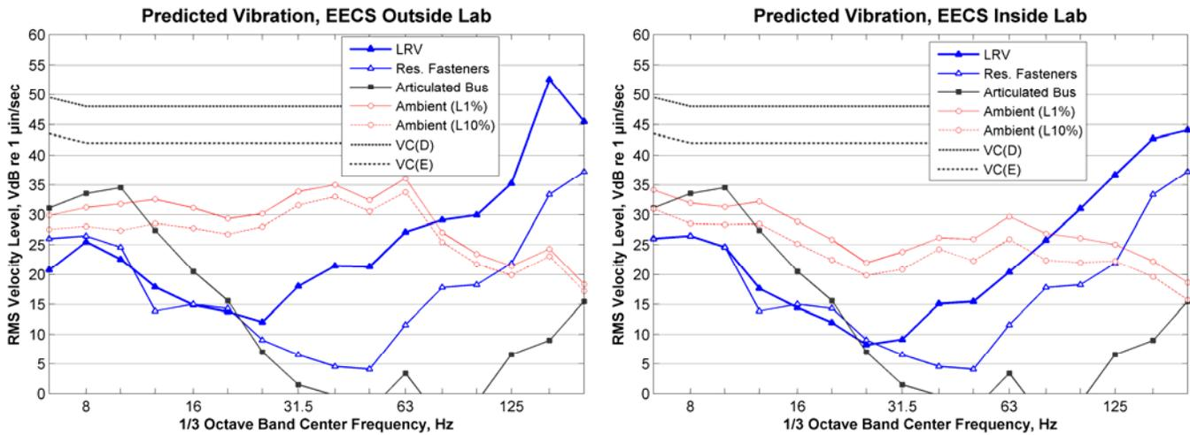
**Figure 64: Predicted Train Vibration, EECS Microscopy Lab**
