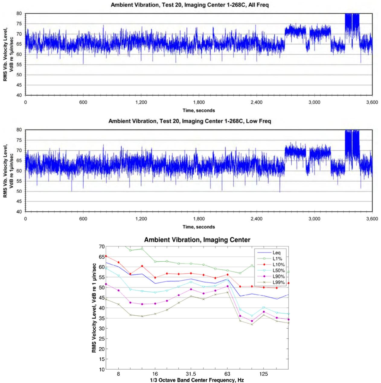
**Figure 147: Ambient Vibration Spectrum inside the Imaging Center at the Philip Wangenstein Building**
