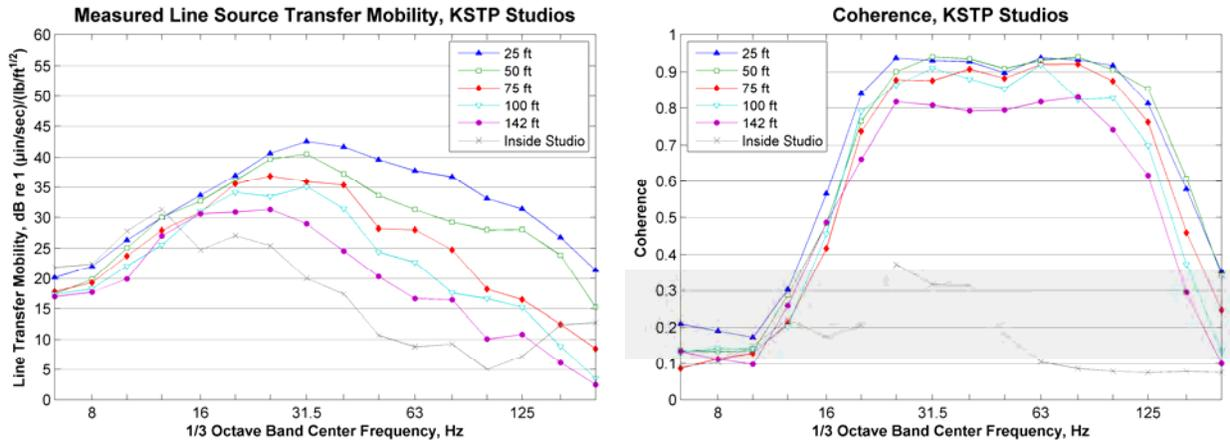
**Figure 153: Measured Line Source Transfer Mobility, KTSP Studio**
