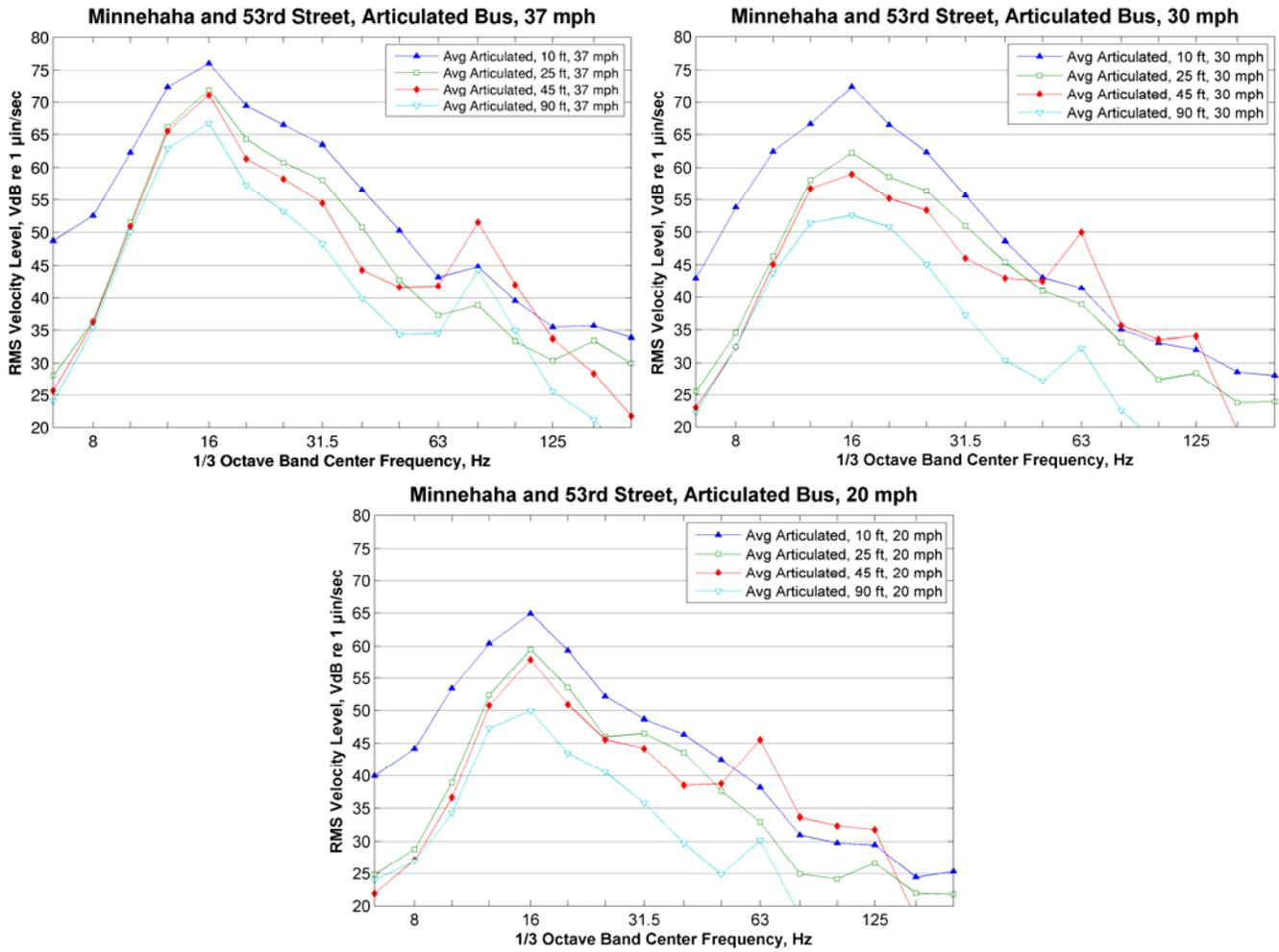
**Figure 31: Average Articulated Bus Vibration Levels, Minnehaha and 53<sup>rd</sup> Street**
