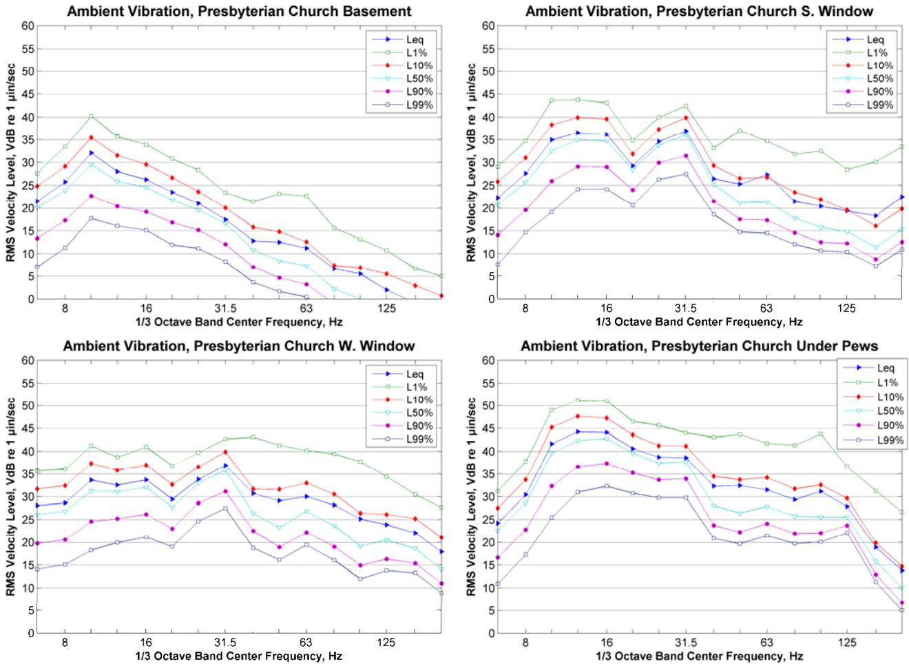
**Figure 158: Ambient Vibration at Indoor LSTM Measurement Positions, Central Presbyterian Church**
