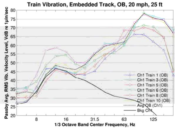
**Figure 19: Train Vibration Levels, 5<sup>th</sup> Street and 5<sup>th</sup> Avenue Embedded Track, 20 mph 25 foot Accelerometer**
