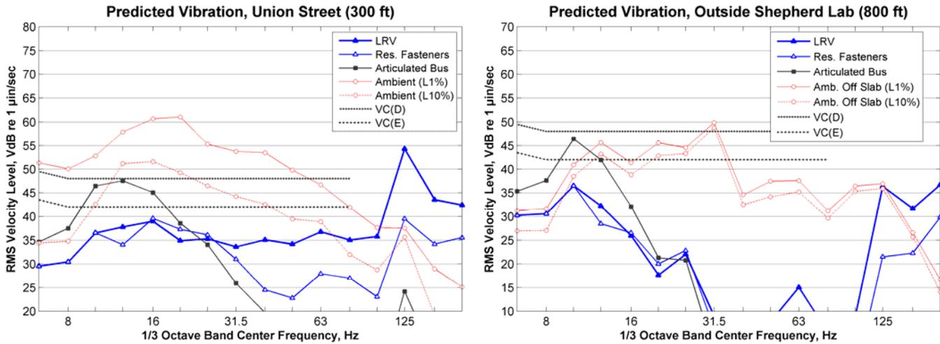
**Figure 62: Predicted Vibration on Union Street and Outside Shepherd Labs**
