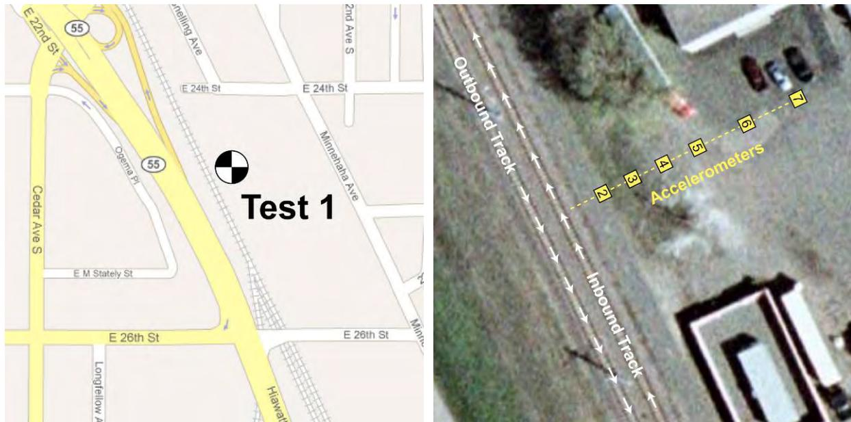
**Figure 10: LRV FDL Measurement Location at 24<sup>th</sup> Street, Ballast and Tie Tracks**
