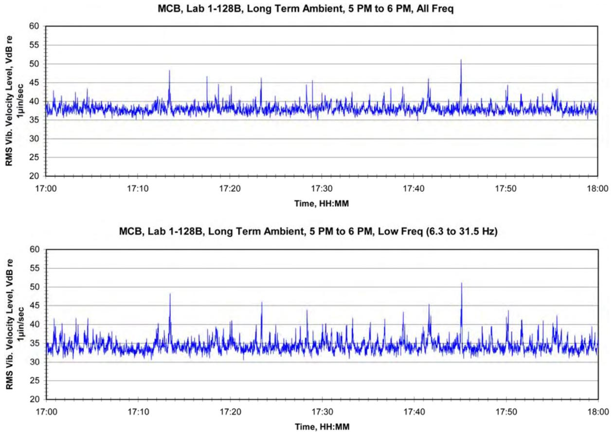
**Figure 109: Time History of Vibration inside Room 1-128B at MCB, Typical Day Time**
