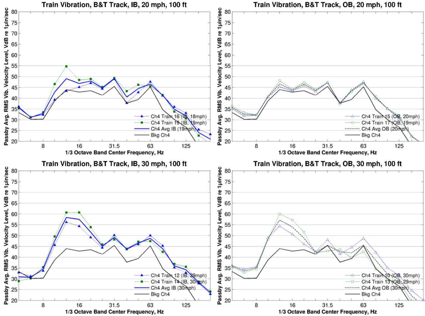
**Figure 185: Vibration Spectra, Ballast & Tie Track, 100 ft, 20 and 30 mph**
