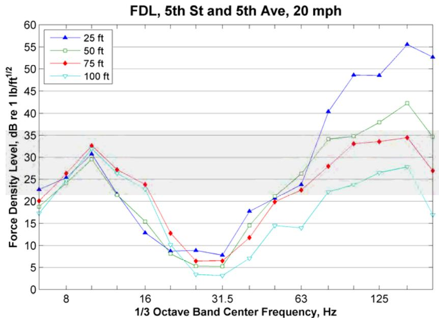
**Figure 21: Measured FDL, Embedded Track, 5th Street and 5th Avenue, 20 mph**
