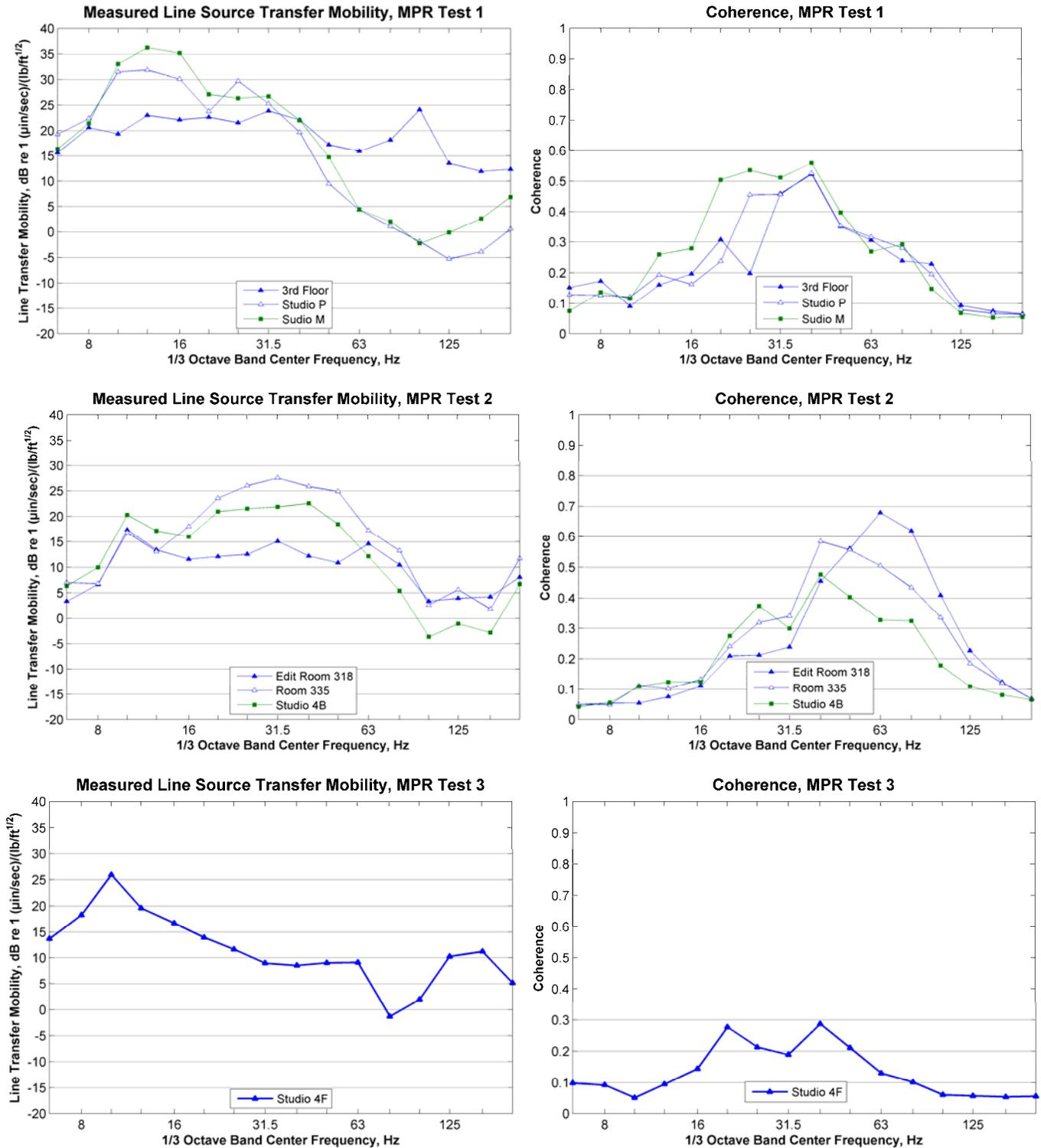
Figure 168: Measured Line Source Transfer Mobility, Tests MPR1, MPR2 and MPR3
