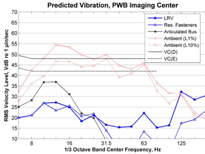
**Figure 148: Predicted Vibration inside the Imaging Center at the Philip Wangenstein Building**
