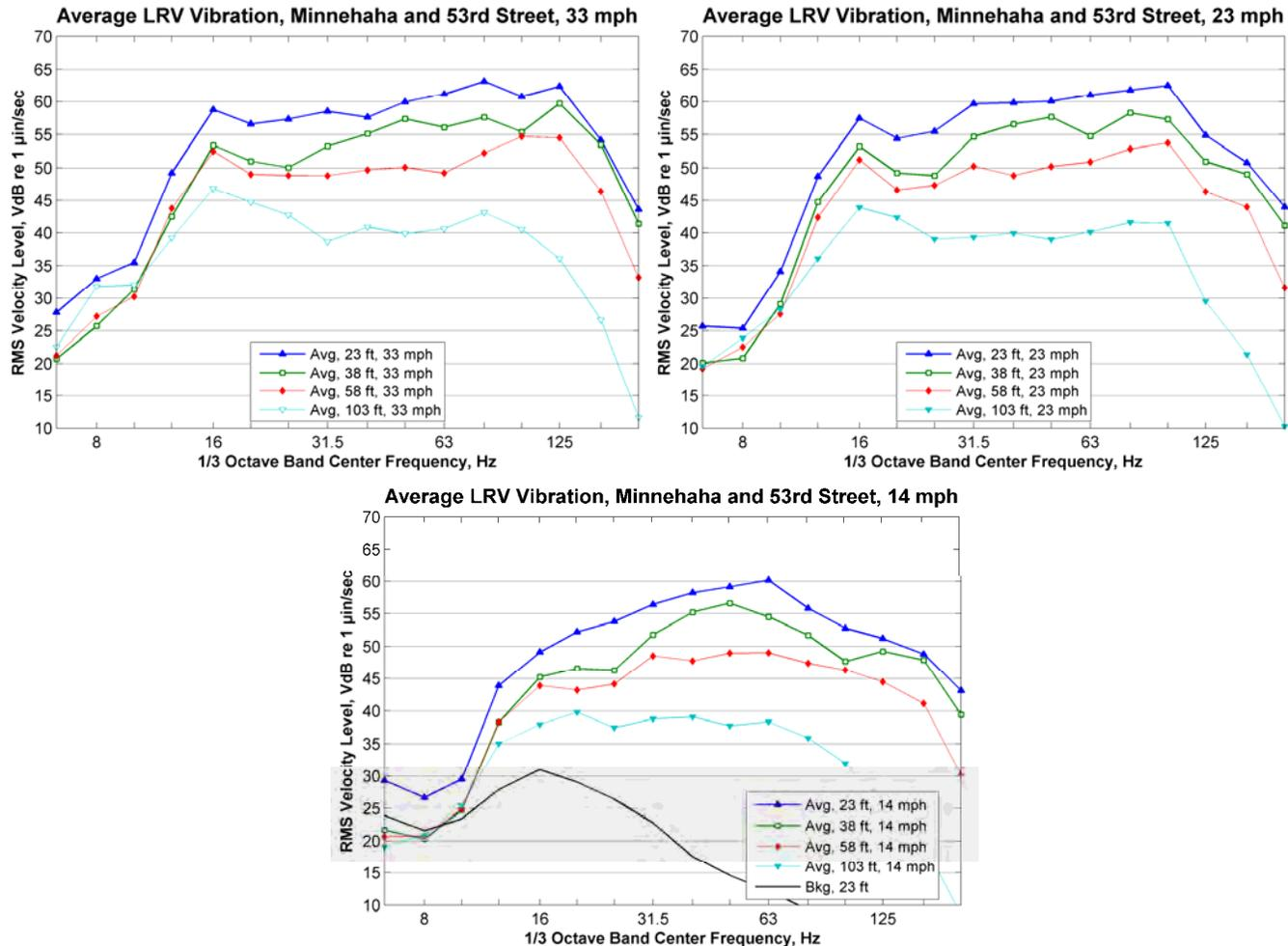
Figure 28: Average Train Vibration Levels, Minnehaha and 53<sup>rd</sup> Street, Embedded Track
