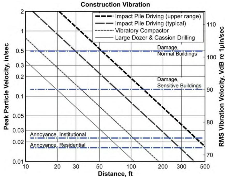
**Figure 177: Typical Vibration Levels from Construction Equipment**
