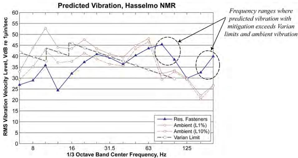
**Figure 52: Predicted Train Vibration with Mitigation inside Hasselmo NMR Lab**
