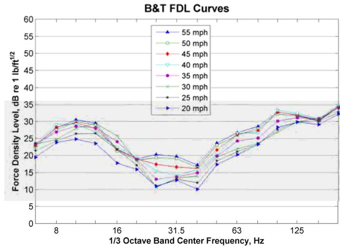
**Figure 14: Derived FDL Curves for Ballast and Tie Track**
