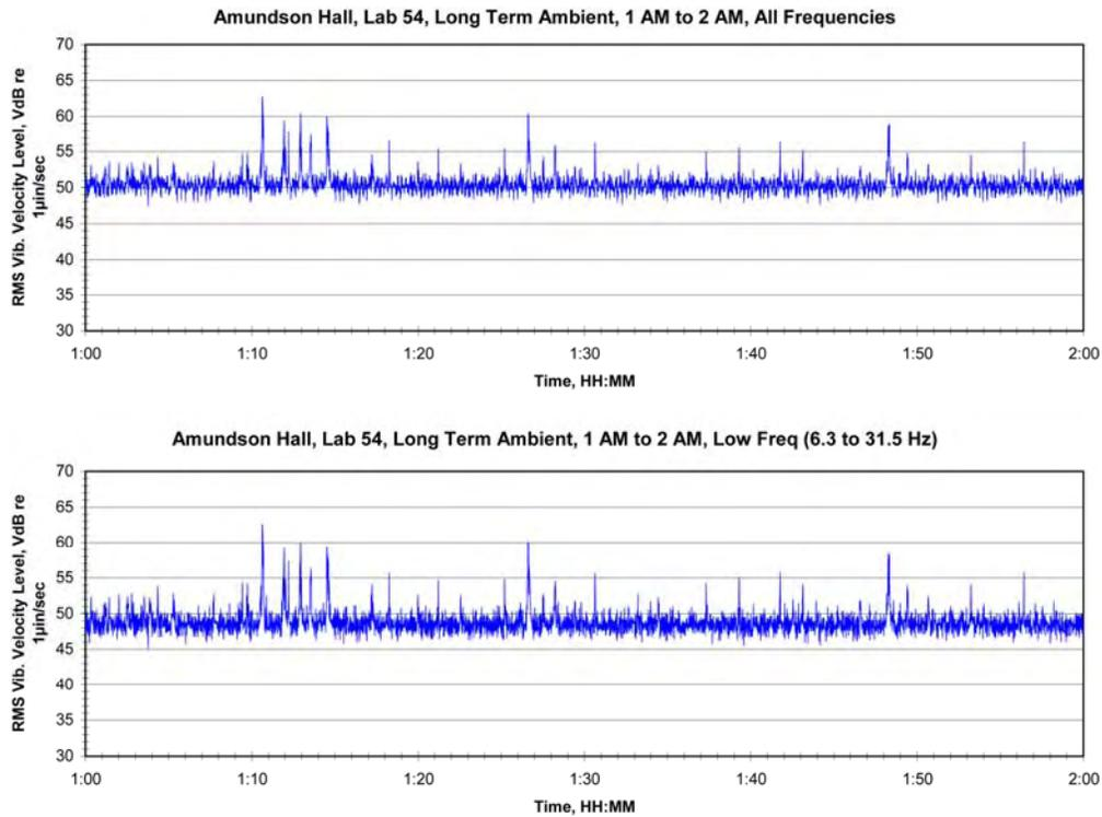
**Figure 126: Ambient Vibration in Amundson Room 54, 1 AM to 2 AM**
