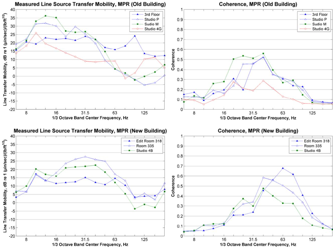
**Figure 169: Comparison of LSTM Curves Measured Studios in Original and New MPR Buildings**
