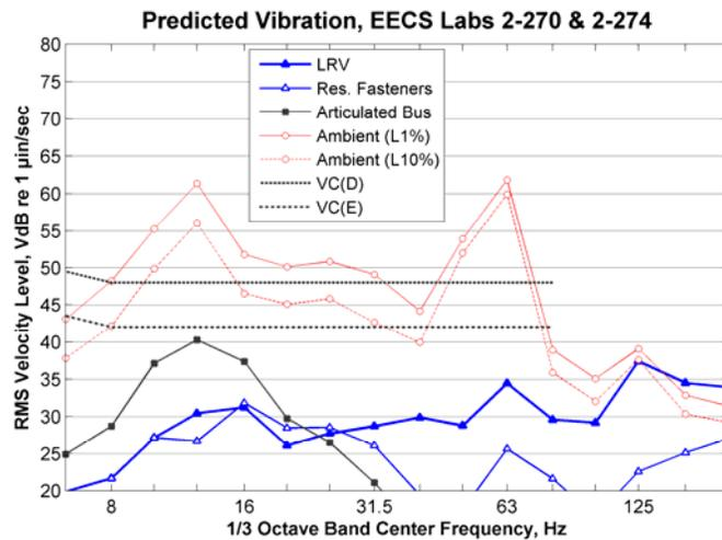
**Figure 123: Predicted Vibration inside Rooms 2-270 and 2-274 at the Electrical Engineering and Computer Science Building**
