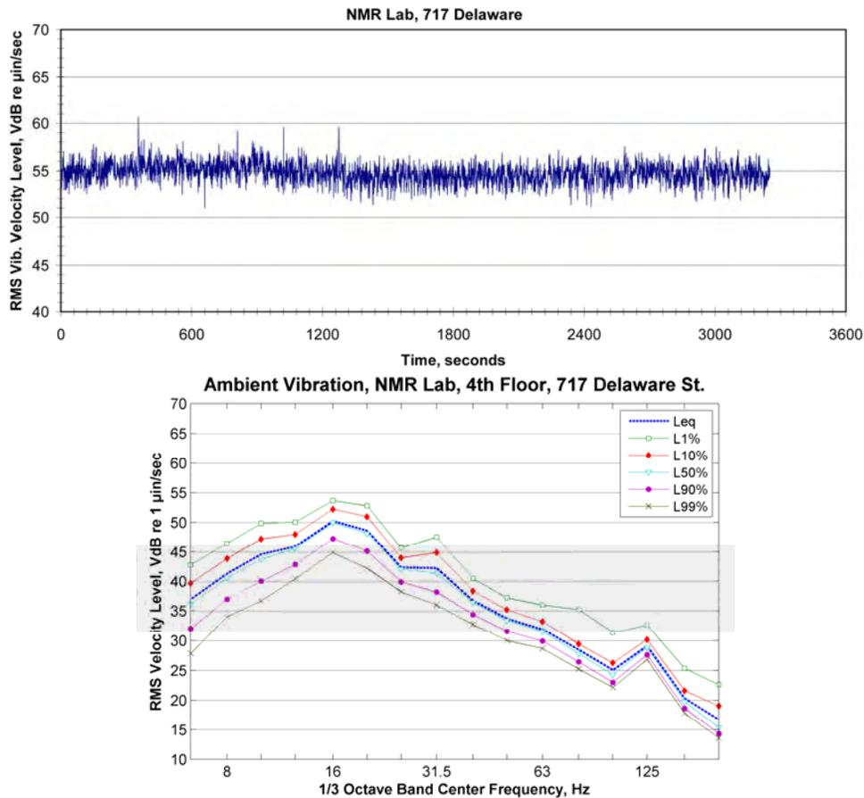
**Figure 80: Ambient Vibration, 717 Delaware Street, NRM Lab on 4<sup>th</sup> Floor**
