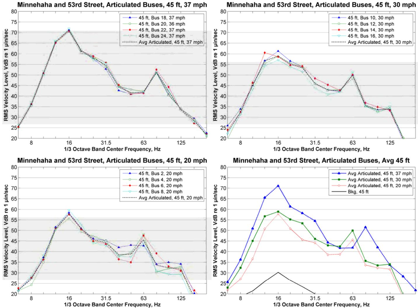
**Figure 205: Articulated Bus Vibration, Minnehaha and 53<sup>rd</sup> Street, 45 ft from Roadway Centerline**
