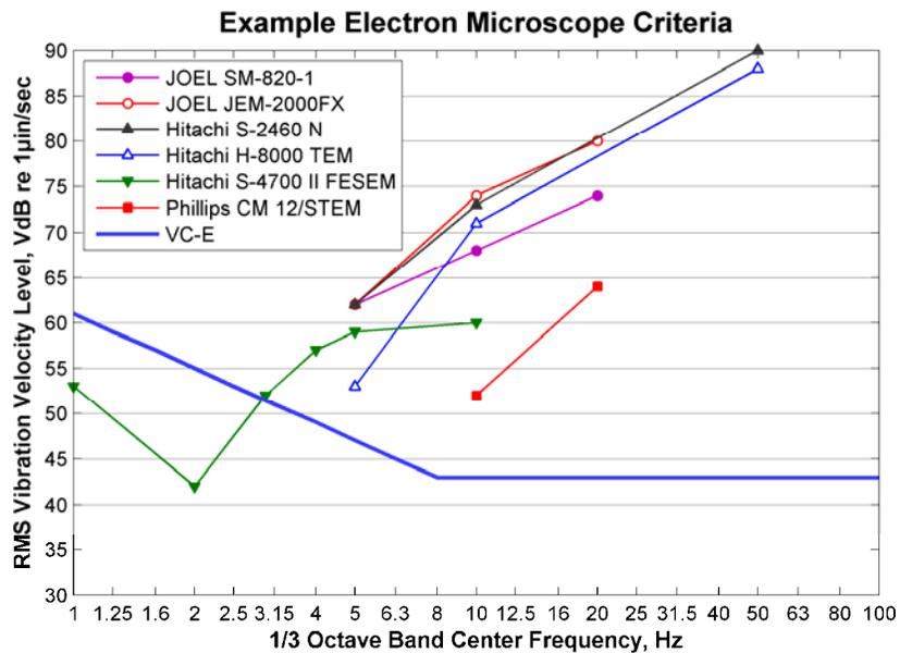
**Figure 4: Example Vibration Criteria for Electron Microscopes**
