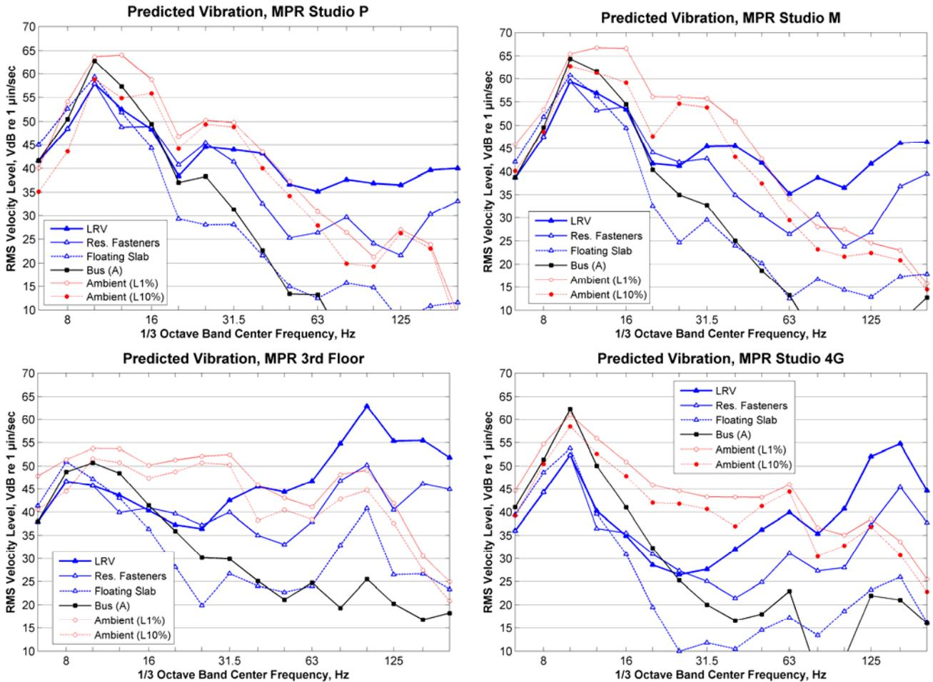
**Figure 175: Predicted Vibration in Studios in Original Building**
