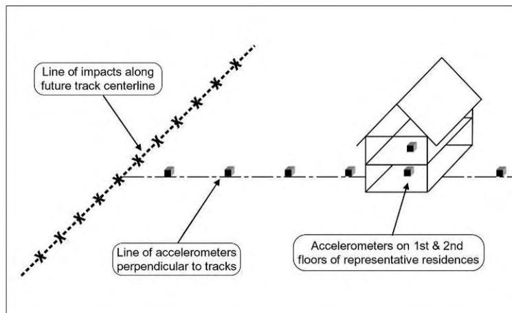
**Figure 1: Schematic of Vibration Test Procedure**
