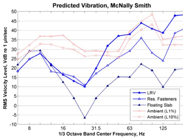
**Figure 166: Predicted Vibration at McNally Smith Performance Center**
