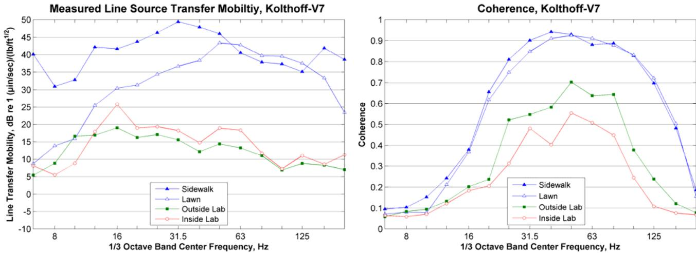
**Figure 68: Measured Line Source Transfer Mobility, Kolthoff Hall Rooms 194/196**
