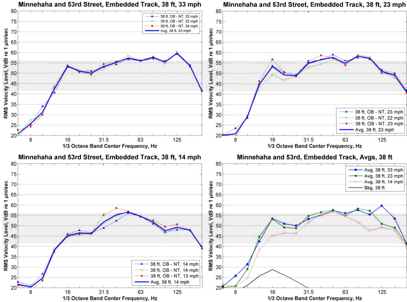
**Figure 197: Train Vibration, Minnehaha and 53<sup>rd</sup> Street, 38 ft from Track Centerline**
