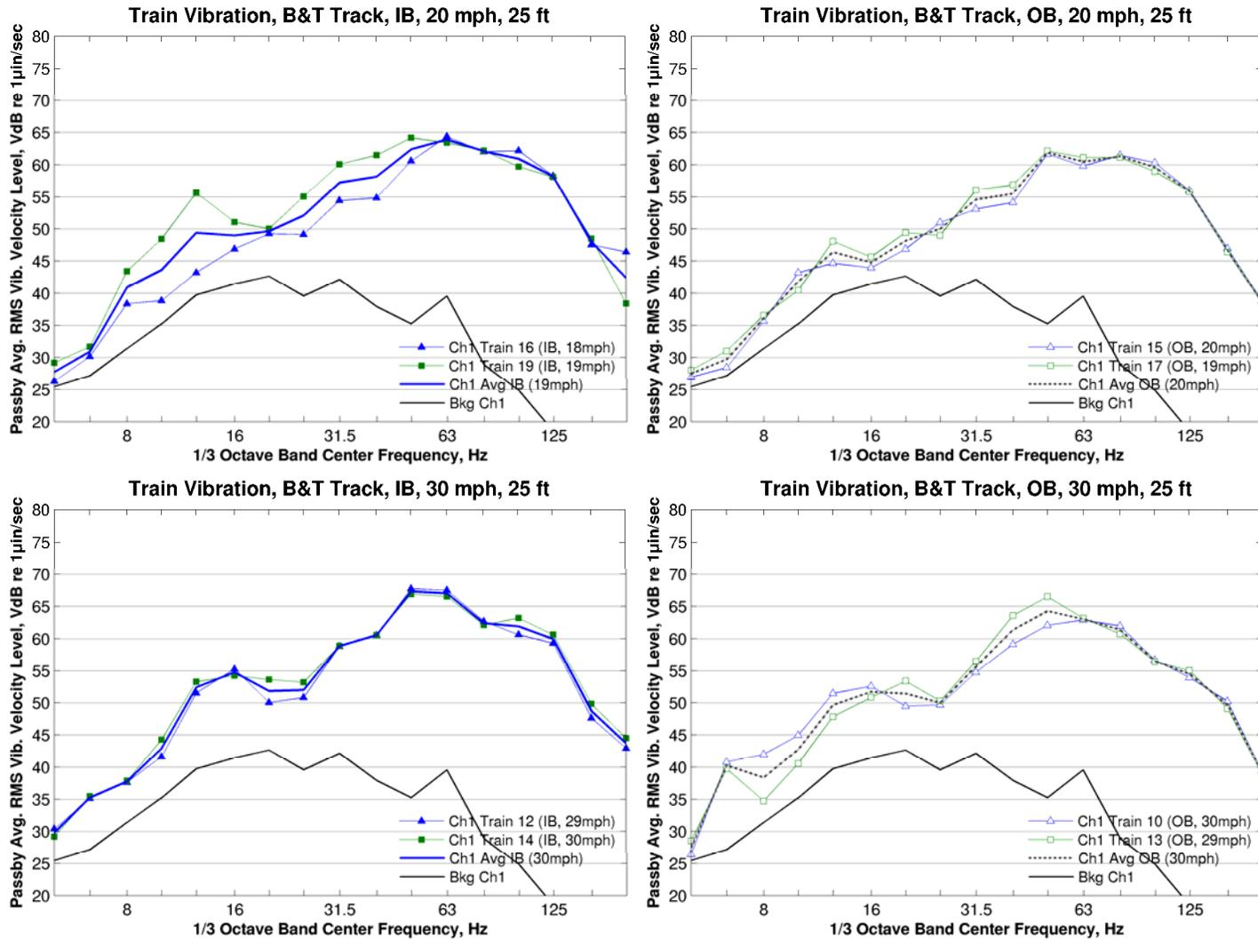
**Figure 179: Vibration Spectra, Ballast & Tie Track, 25 ft, 20 and 30 mph**
