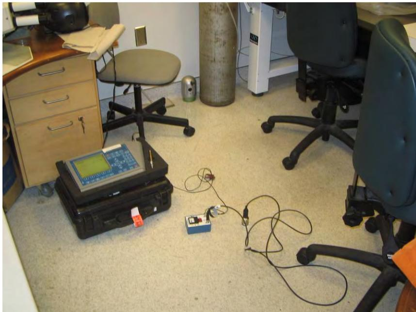
**Figure 113: Vibration Measurement on the Floor of Room 5-108A at Moos Tower**
