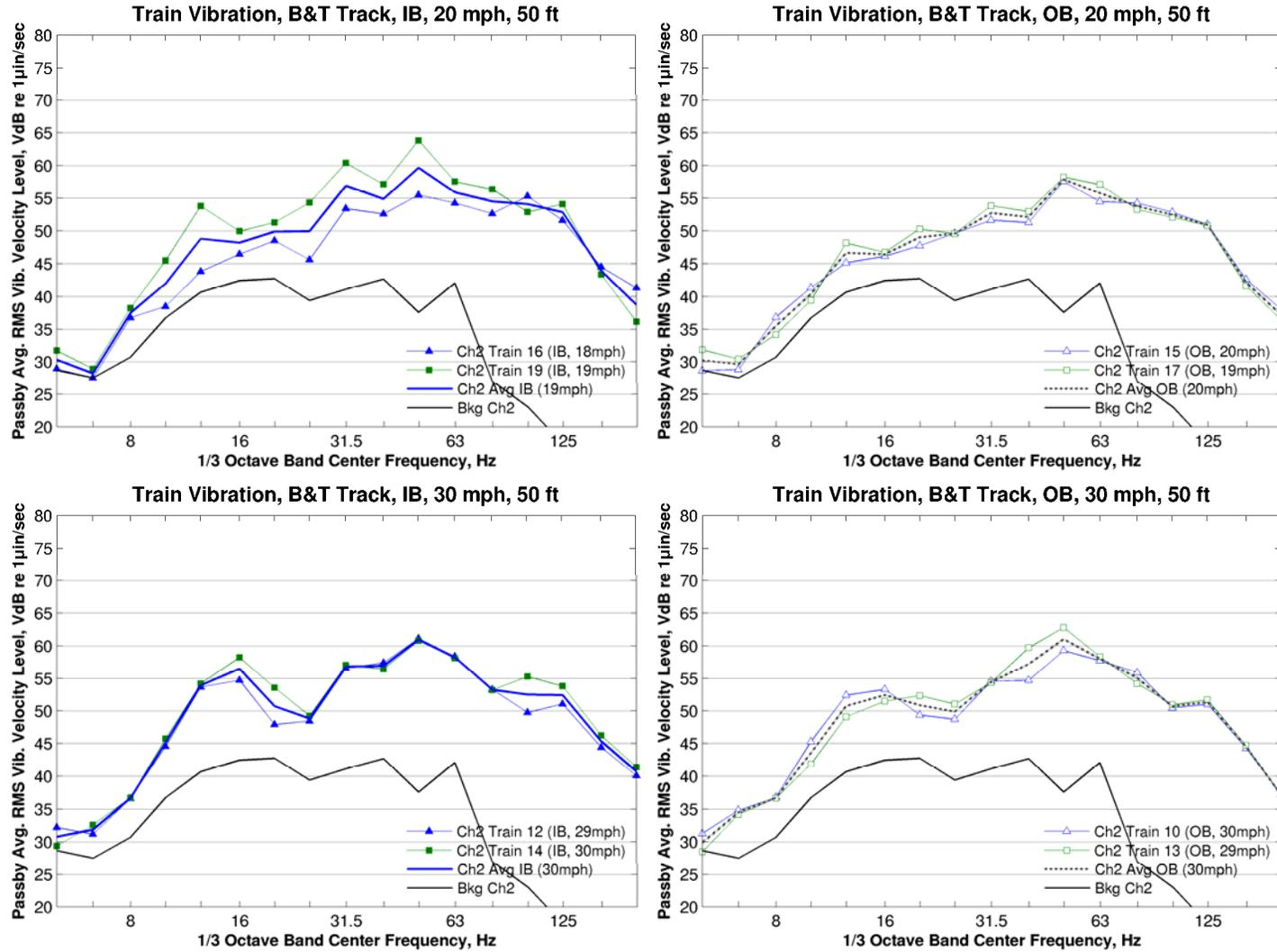
**Figure 181: Vibration Spectra, Ballast & Tie Track, 50 ft, 20 and 30 mph**
