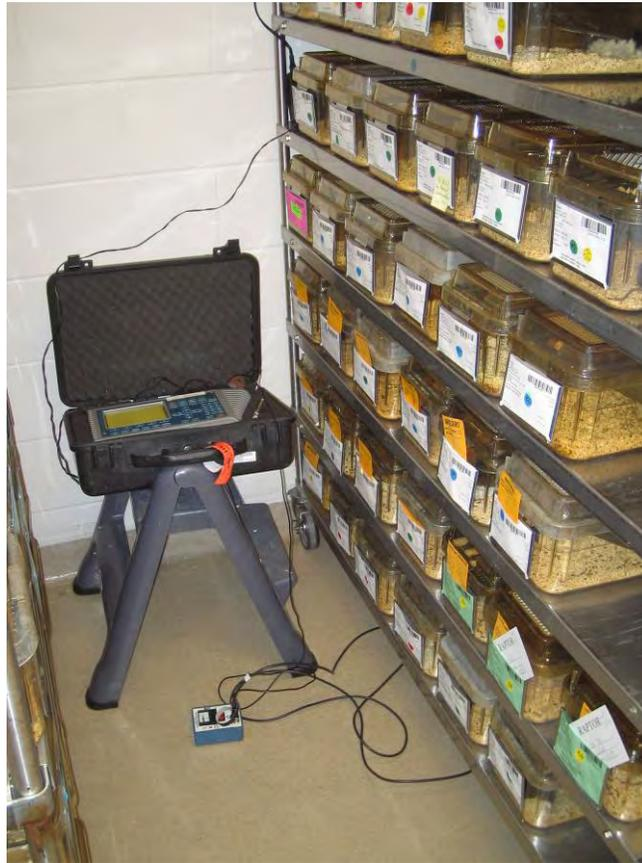
**Figure 108: Vibration Measurement on the Floor of MCB Room 1-128B**
