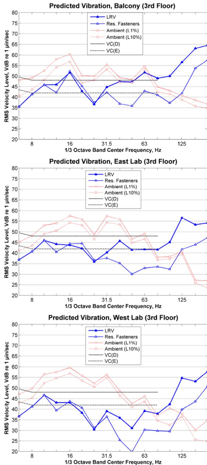
**Figure 150: Predicted Vibration inside MDH/MDA Lab Building, 3<sup>rd</sup> Floor**
