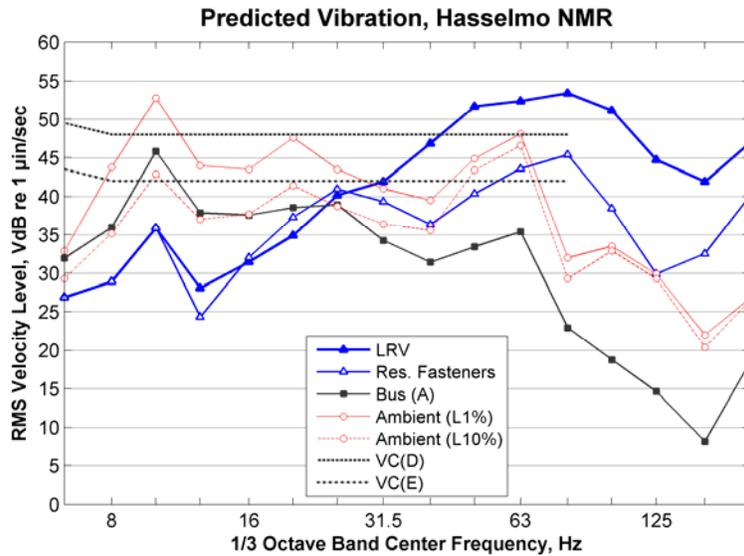
**Figure 51: Predicted Train Vibration inside Hasselmo NMR Lab**
