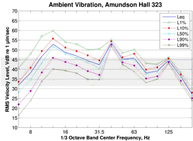
**Figure 135: Ambient Vibration Spectrum inside Room 323 at Amundson Hall**
