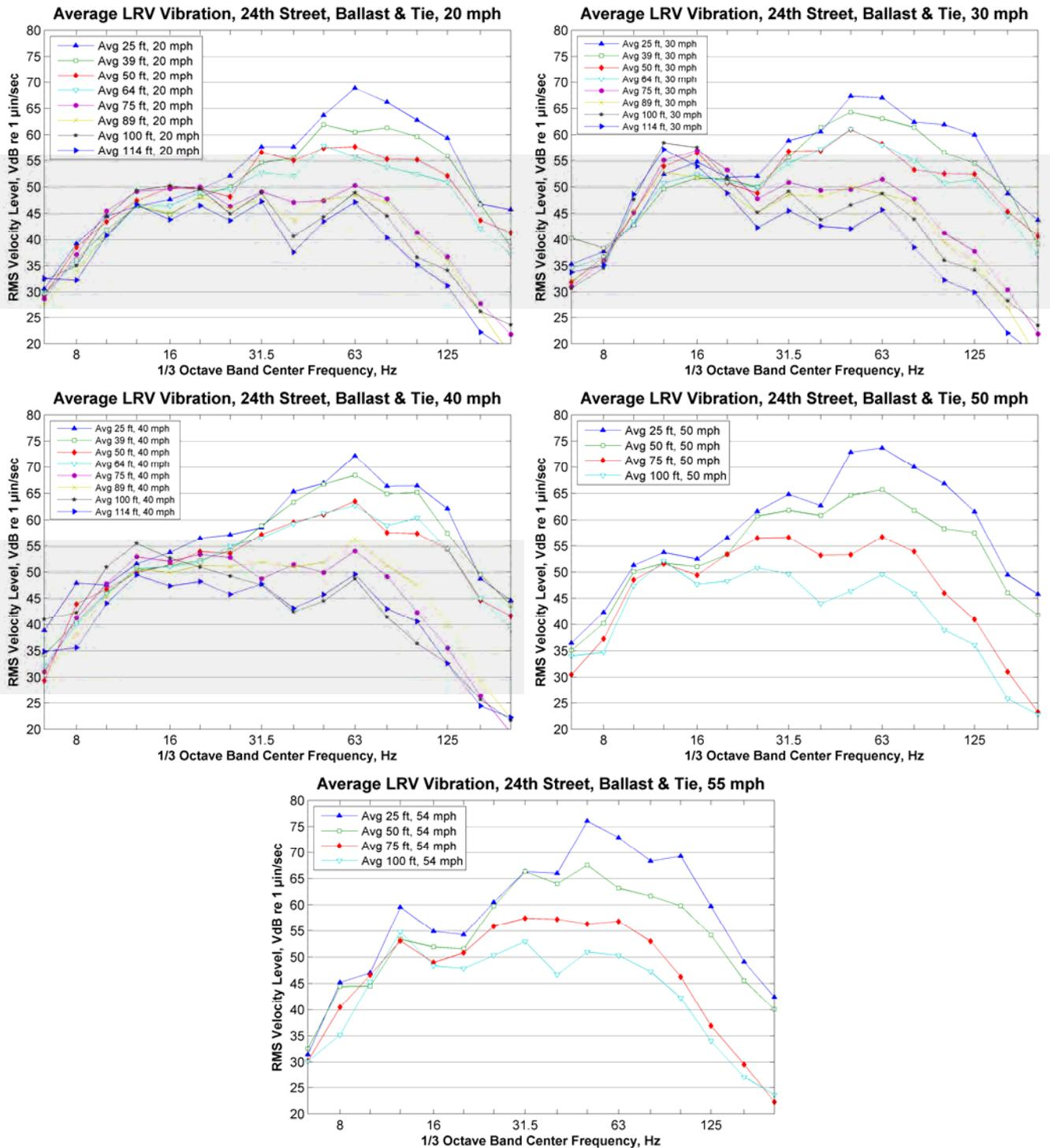
Figure 12: Average Train Vibration Levels, 24<sup>th</sup> Street Ballast and Tie Track
