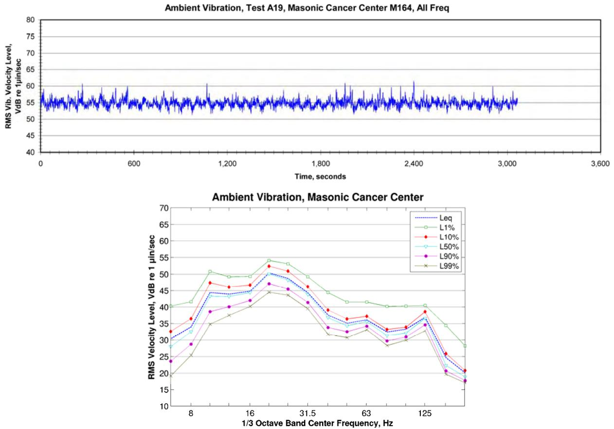
**Figure 144: Ambient Vibration inside the Masonic Cancer Center**
