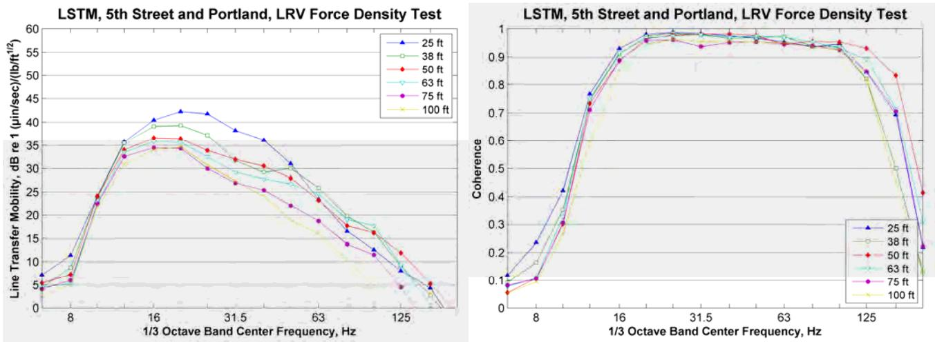
**Figure 23: Line-Source Transfer Mobility, 5<sup>th</sup> St. and Portland Avenue Embedded Track**
