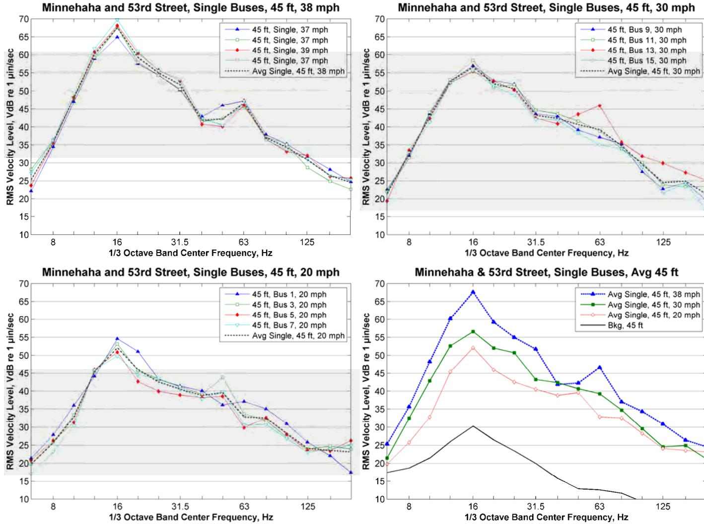
**Figure 204: Single Bus Vibration, Minnehaha and 53<sup>rd</sup> Street, 45 ft from Roadway Centerline**
