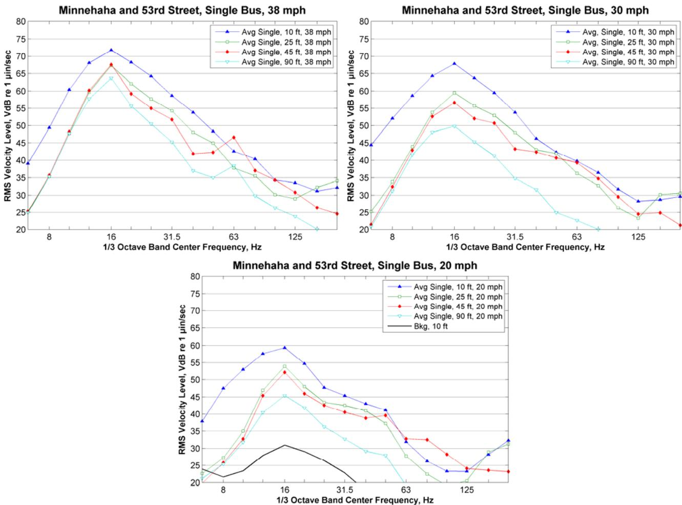
**Figure 30: Average Single Bus Vibration Levels, Minnehaha and 53<sup>rd</sup> Street**
