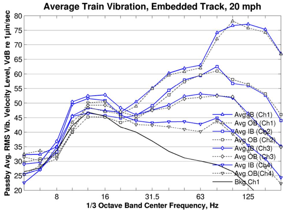
Figure 187: Average Vibration Spectra, 5th Street and 5<sup>th</sup> Avenue Embedded Track
