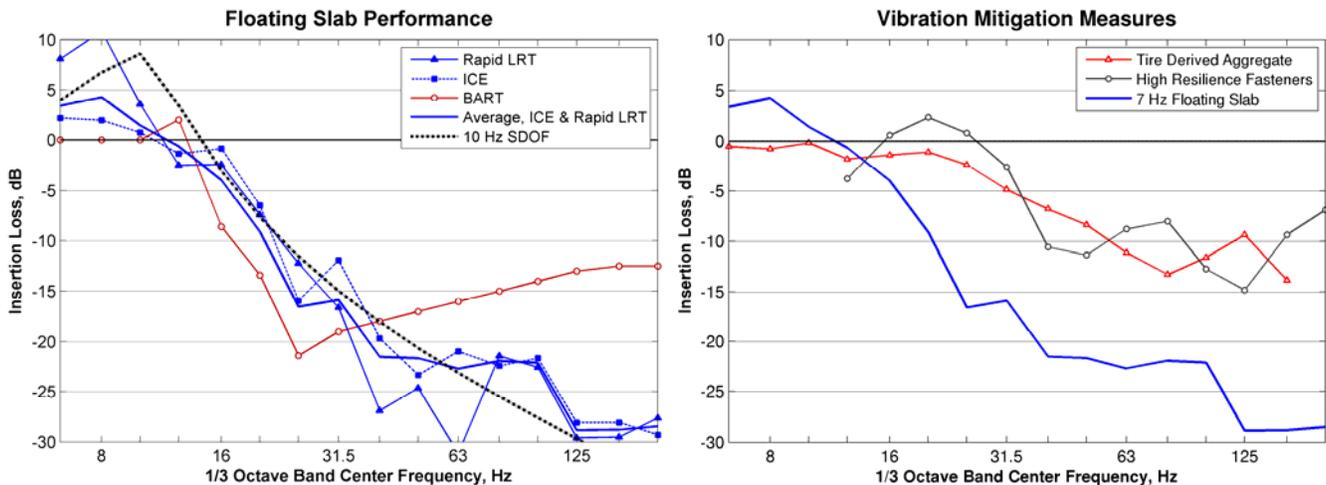
**Figure 6: Performance of Different Vibration Mitigation Measures**
