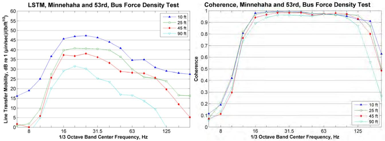
**Figure 32: Line-Source Transfer Mobility, Bus FDL Test, Minnehaha & 53<sup>rd</sup> Street**
