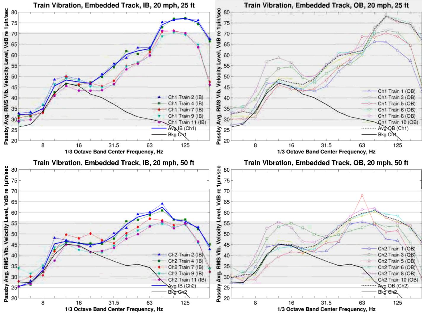
Figure 188: Vibration Spectra, 5<sup>th</sup> Street and 5<sup>th</sup> Avenue Embedded Track, 25 and 50 ft, 20 mph
