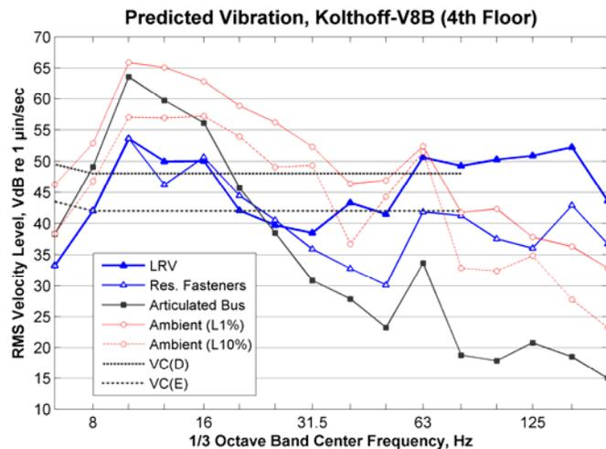
**Figure 75: Predicted Vibration and Mitigation inside 4<sup>th</sup> Floor Lab, Kolthoff Hall**
