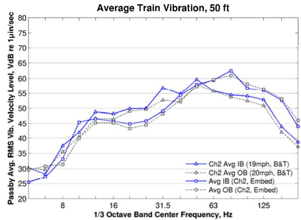
**Figure 20: Comparison of HLRT Vibration Spectra, Tests 1 and 2**
