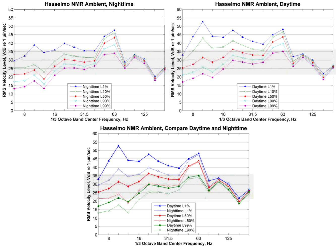
**Figure 49: Daytime and Nighttime Exceedance Levels, Ambient Vibration in Hasselmo NMR Lab (Channel 1)**
