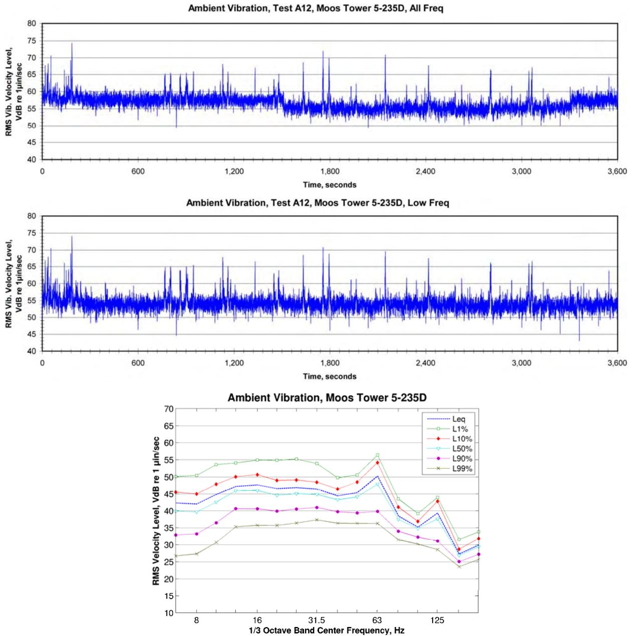
**Figure 117: Ambient Vibration inside Moos Tower Room 5-235D**
