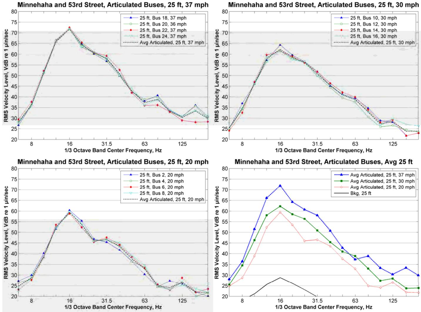
**Figure 203: Articulated Bus Vibration, Minnehaha and 53<sup>rd</sup> Street, 25 ft from Roadway Centerline**
