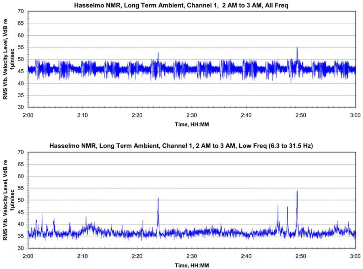
**Figure 46: Ambient Vibration in Hasselmo NMR Lab, Typical Nighttime Hour**
