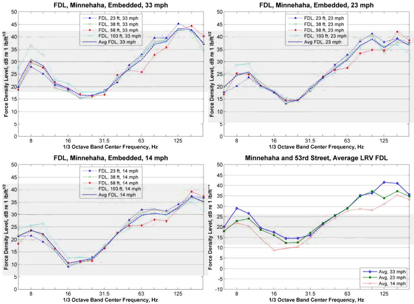
**Figure 29: LRV Force Density Levels, Minnehaha and 53<sup>rd</sup> Avenue, Embedded Track**
