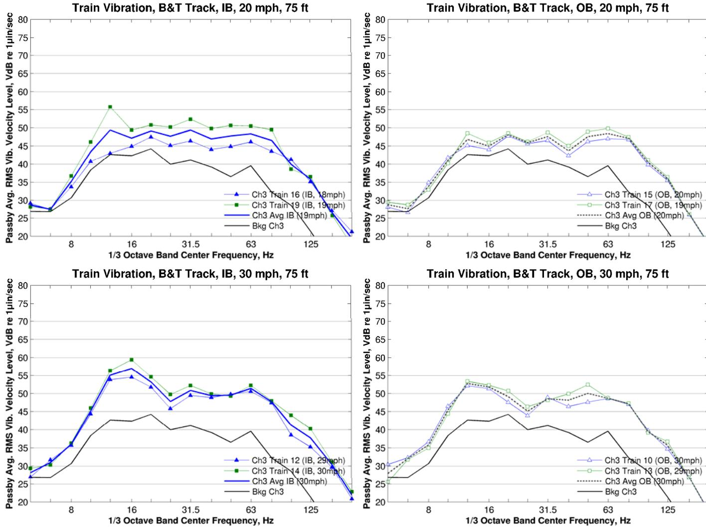
**Figure 183: Vibration Spectra, Ballast & Tie Track, 75 ft, 20 and 30 mph**
