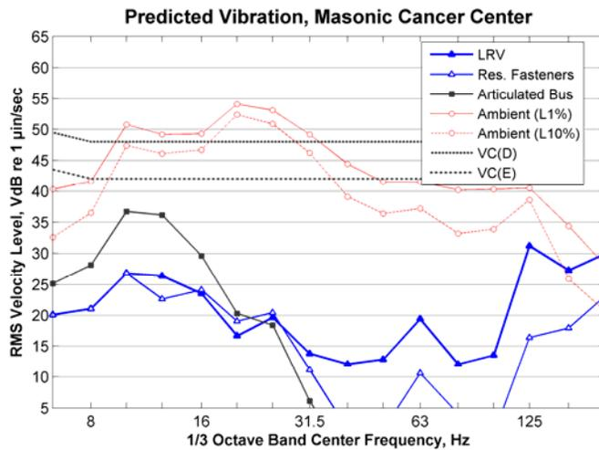
**Figure 145: Predicted Vibration inside Room M164 at the Masonic Cancer Center**
