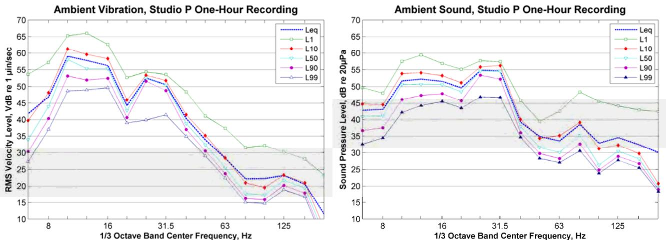
**Figure 172: Statistics of Simultaneous Vibration and Sound Measurements inside Studio P**
