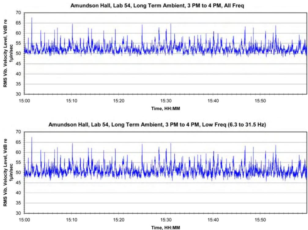
**Figure 127: Ambient Vibration in Amundson Room 54, 3 PM to 4 PM**
