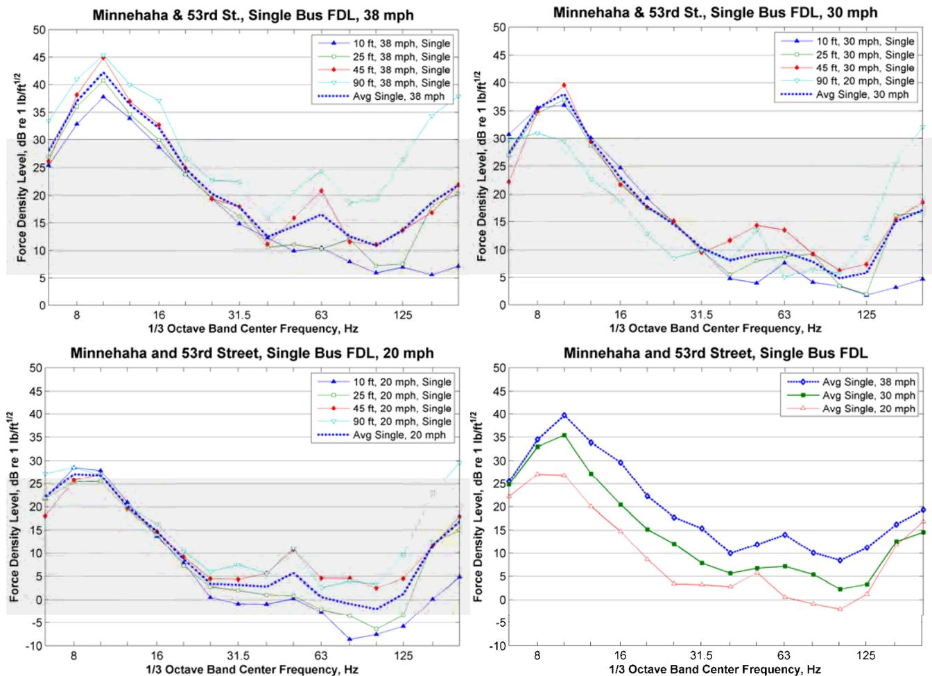
**Figure 33: Single Bus Force Density Levels, Minnehaha and 53<sup>rd</sup> Street**
