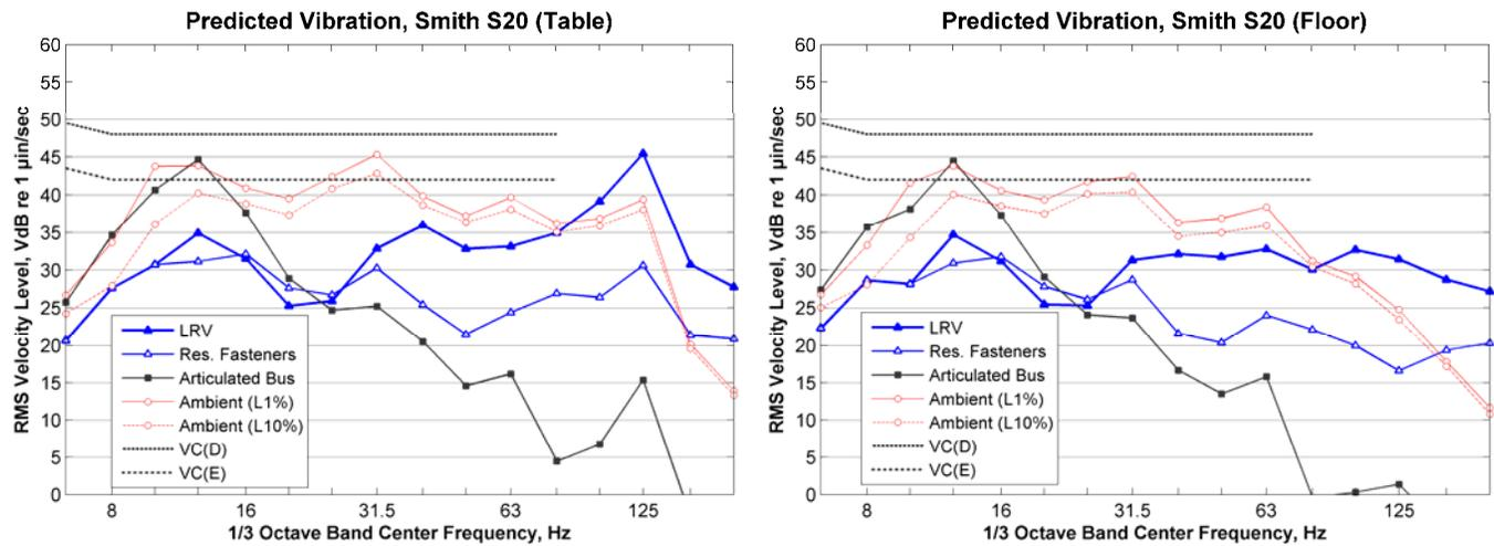
**Figure 79: Predicted Vibration and Mitigation inside Smith S20**
