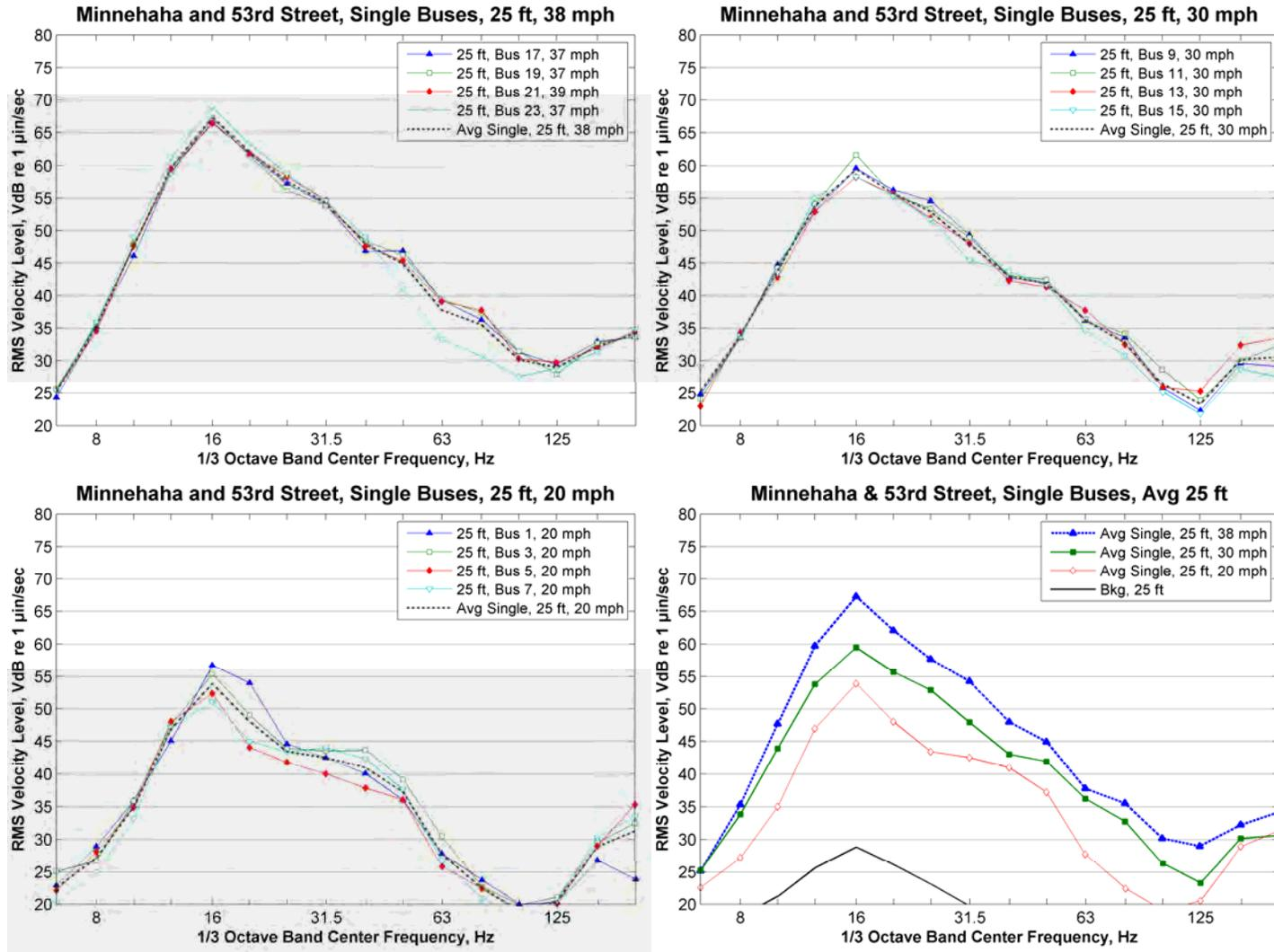
**Figure 202: Single Bus Vibration, Minnehaha and 53<sup>rd</sup> Street, 25 ft from Roadway Centerline**
