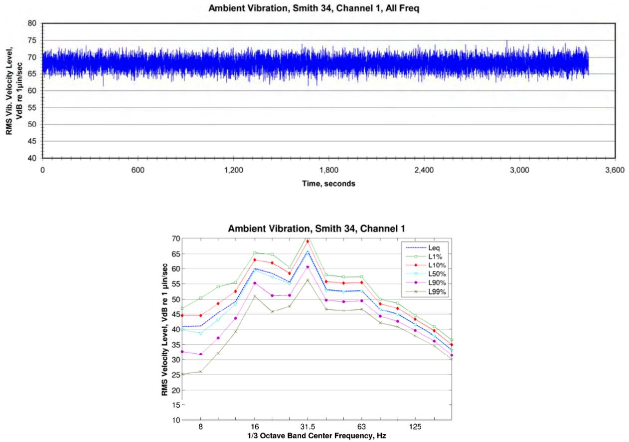
**Figure 85: Ambient Vibration inside Room S34 at Smith Hall**
