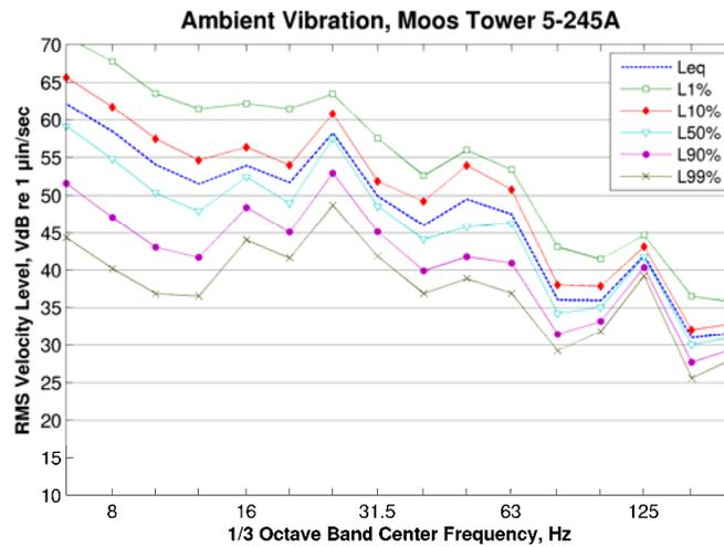
**Figure 106: Ambient Vibration inside Room 5-245A at Moos Tower**
