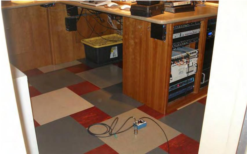
**Figure 151: Indoor Accelerometer at KSTP Television Studio**
