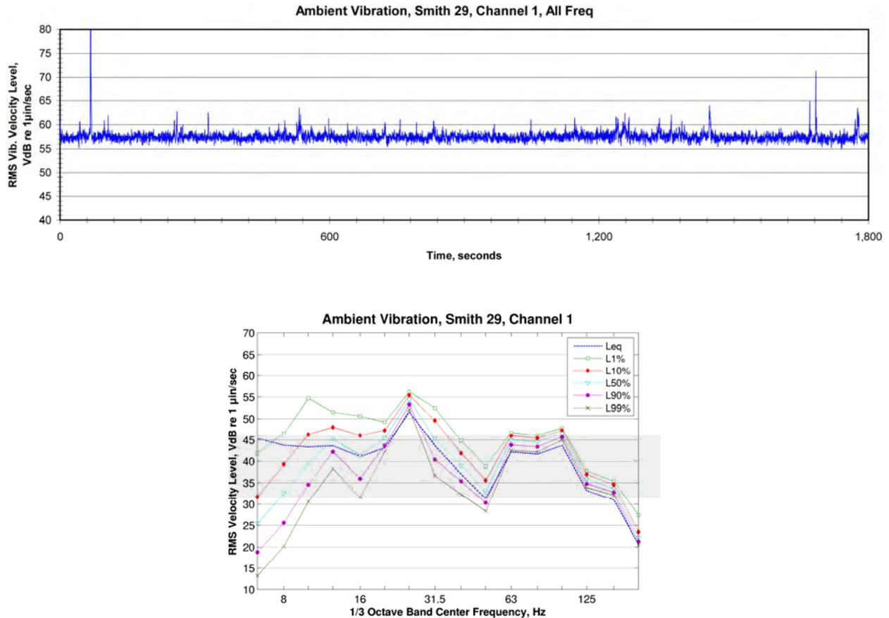
**Figure 83: Ambient Vibration inside Room S29 at Smith Hall**
