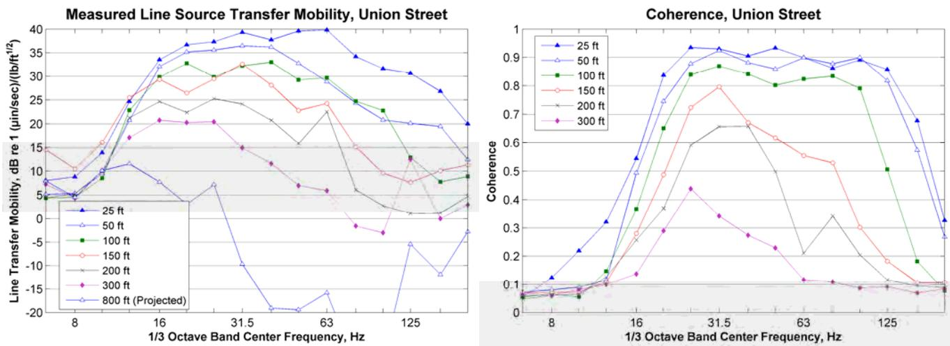
**Figure 61: Measured Line Source Transfer Mobility, Union Street**
