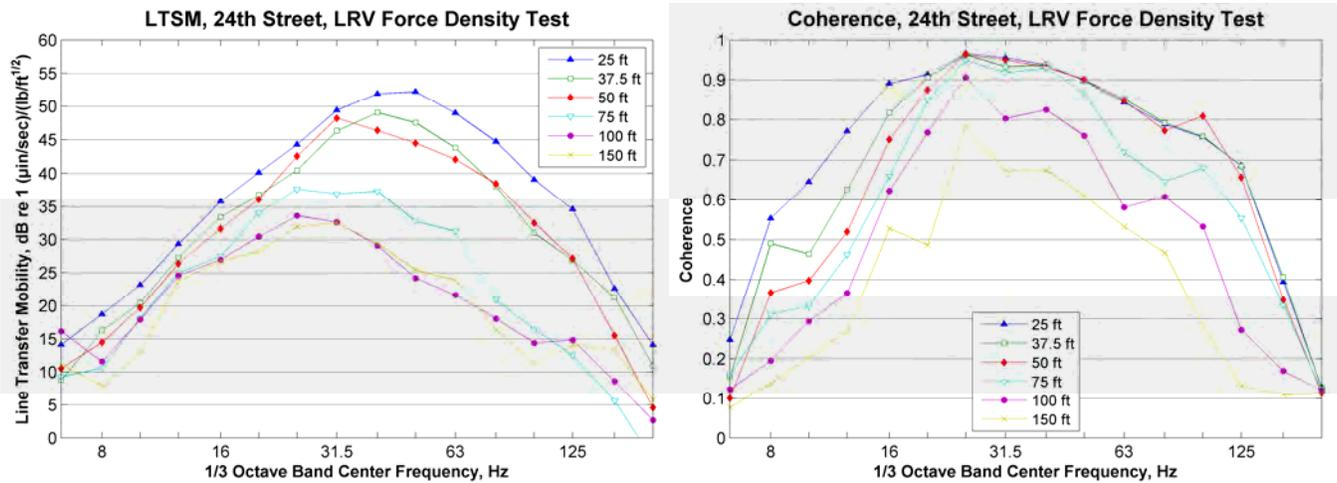
**Figure 11: Measured Line Source Transfer Mobility, 24th Street FDL Test Site**
