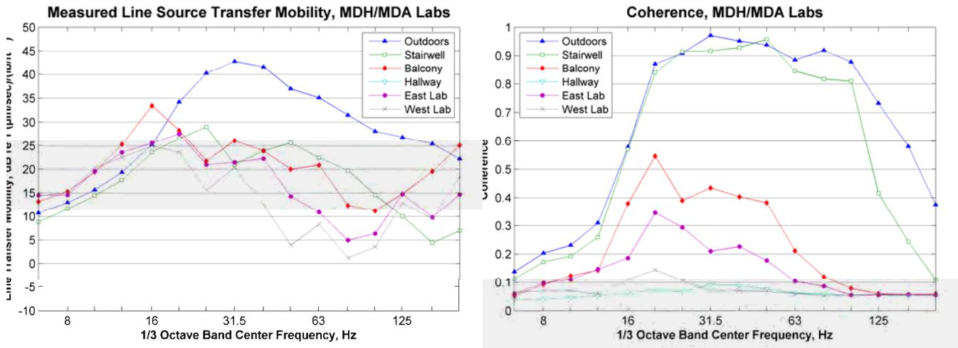
**Figure 149: Measured Line Source Transfer Mobility, MDH/MDA Lab Building**
