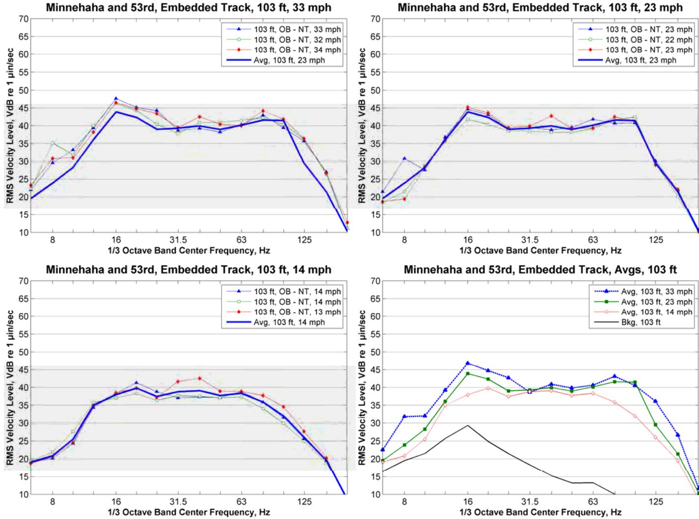
Figure 199: Train Vibration, Minnehaha and 53<sup>rd</sup> Street, 103 ft from Track Centerline
