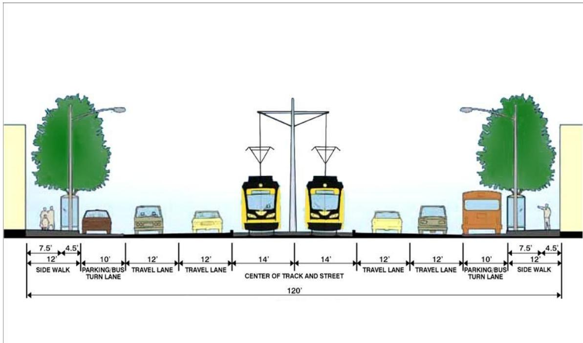
**FIGURE 2-10 WASHINGTON AVENUE TRANSIT/PEDESTRIAN MALL TYPICAL CROSS SECTION**
