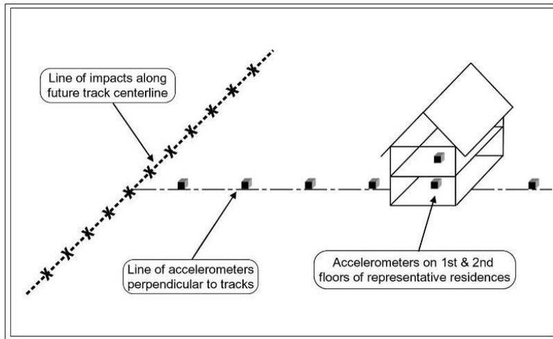
Notes: The impacts were generated with device that drops a 45 lb weight from a height of 4 feet onto a load cell. The vibration signals were measured with seismic accelerometers; signals from the load cell and accelerometers were digitally recorded.
