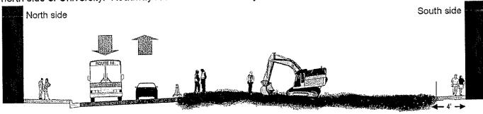
Stage 2: Work shifts to north two-thirds of University. One lane of traffic maintained in each direction on the newly restored road on the south side of University. Pavement restored within 150 days.
