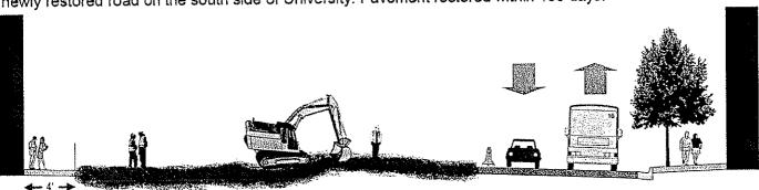
**Stage 3:** Two lanes of traffic restored in each direction. Work continues on guideway, track and stations in the middle of University through November 2011. In 2012, crews return to complete station and tracks and install overhead wires and communication systems.
