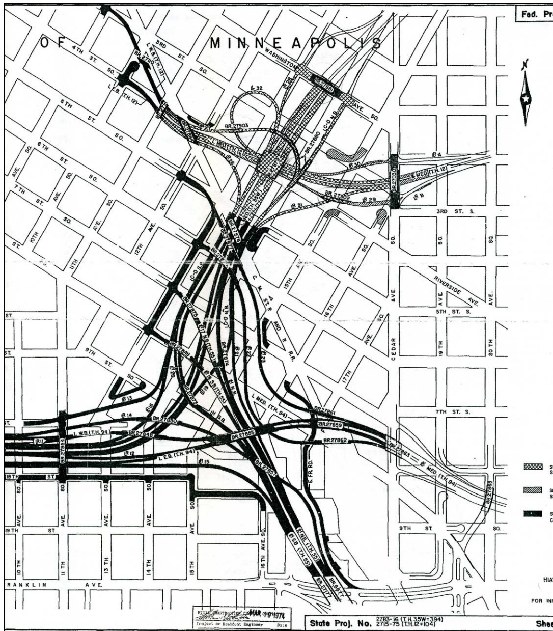
Plans for the Hiawatha Interchange, 1970, showing the connecting roads and bridges. The connection to the Washington Avenue Bridge is on the upper right. Source: MnDOT, Microfilm Roll 438
