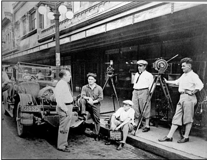
Portable generator mounted on car to provide power on location, 1927. This was one of the innovations devised by the company staff.
