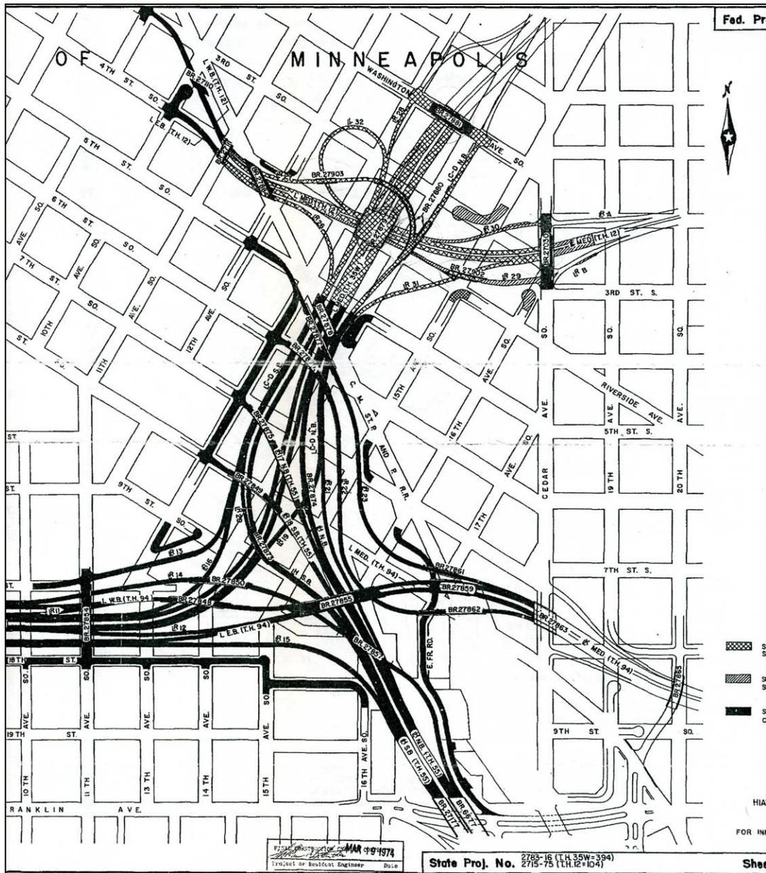
Plans for the Hiawatha Interchange, 1970, showing the connecting roads and bridges. The connection to the Washington Avenue Bridge is on the upper right.
