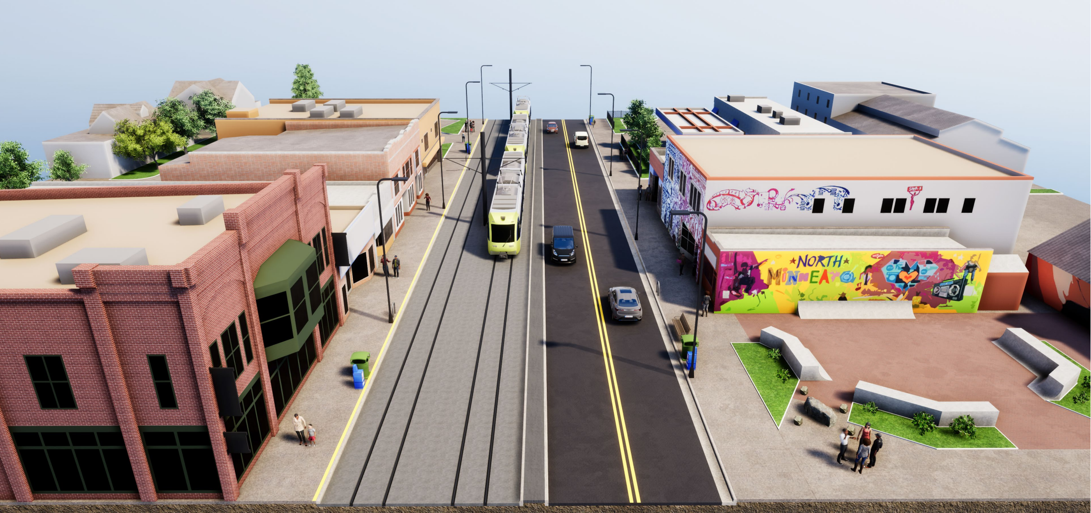
This visualization represents how a side running LRT could fit along West Broadway Avenue.
