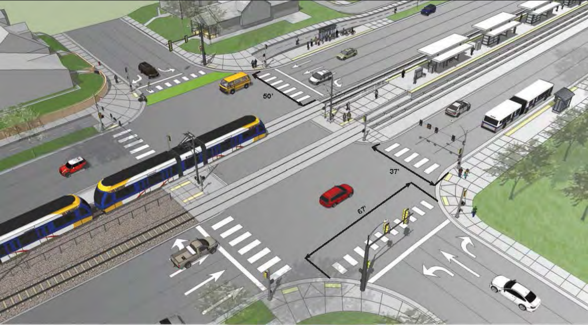
Figure 3.4-2. Conceptual Intersection Pedestrian Safety Improvements
