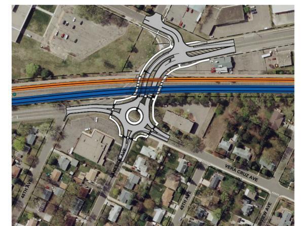
The West Broadway Crossing includes a roundabout to allow full access to the neighborhood to the east. A gate is proposed at the roundabout to prevent traffic from driving around barriers.
