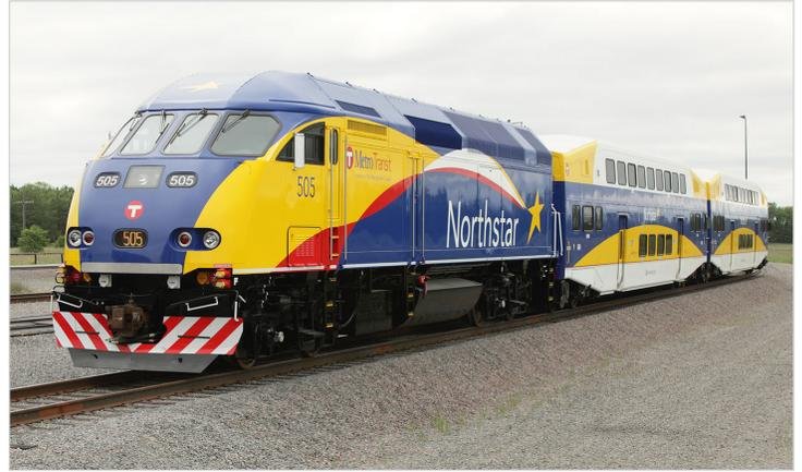
Northstar commuter rail trains, like the one shown on the right above, are pulled by large diesel-electric locomotives and operate over longer distances with fewer stops. Commuter rail trains share track with freight rail service.
