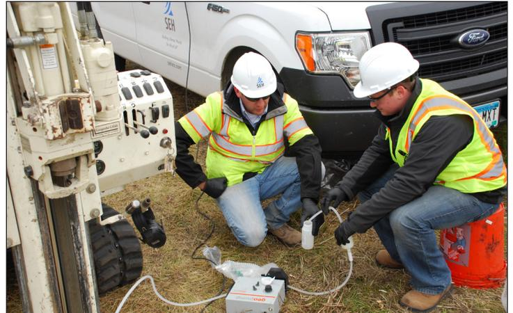
*Environmental technicians are testing soil along the Blue Line Extension route for possible contamination.*
