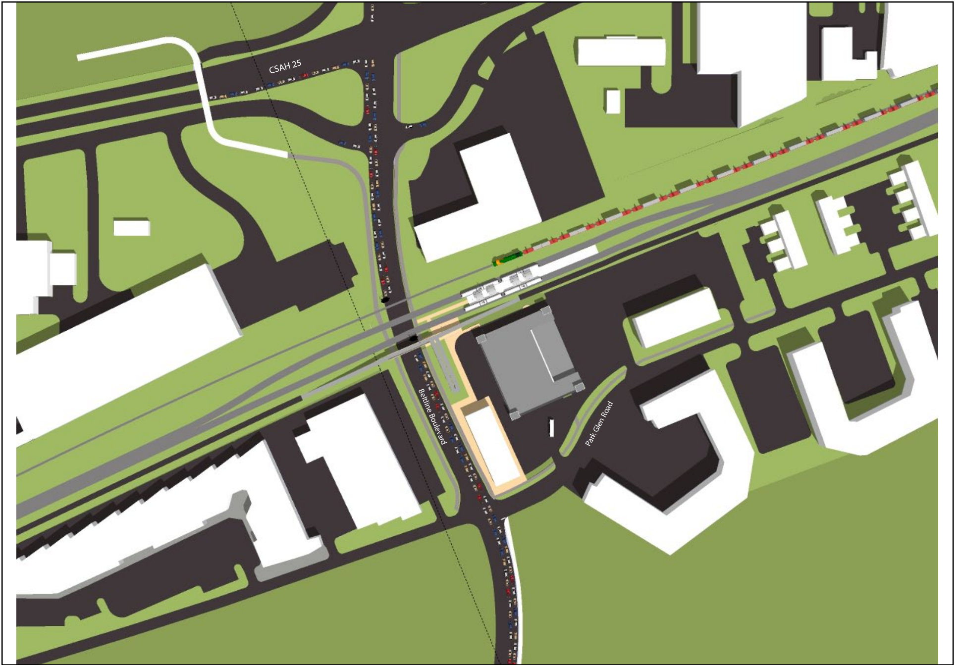
1D Beltline Station- Grade Separated Trail, LRT and Freight Rail at grade
