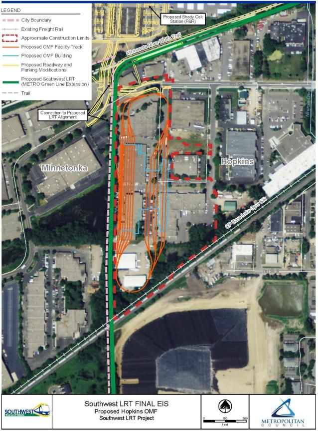
west side of the facility to accommodate total of 36 vehicles (adequate land exists for the expansion). Heavy maintenance of the Project's LRVs, which will include wheel truing and major body repair and painting, will occur at the Franklin Street OMF, which is outside of the project vicinity and will not need to be expanded to accommodate the Project's LRV fleet.
