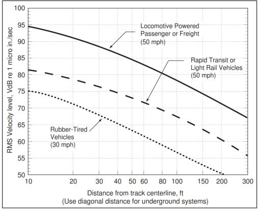
Figure 1. FTA Generalized Ground Surface Vibration Curve
