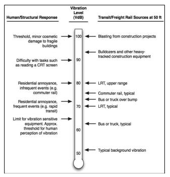
Ground-borne noise (GBN) is also assessed. GBN is a form of low-frequency noise that radiates from building walls and ceilings due to vibration caused by LRT or freight rail operation. Because airborne noise typically masks GBN for above ground (at-grade or elevated) transit systems, GBN is only assessed for operations in tunnels (where airborne noise is not a factor) or near locations such as recording studios that are well insulated from airborne noise.
