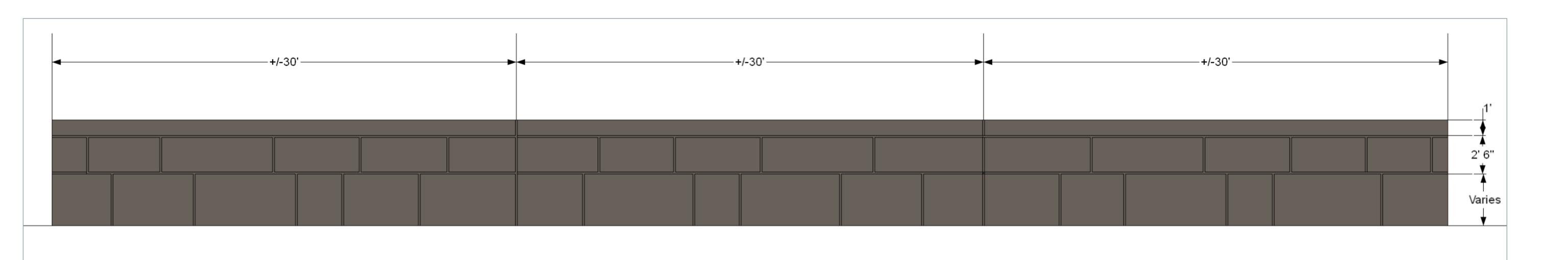
Detail of the proposed wall surface. Repeating 30-foot-long segments create the appearance of cut stone.
