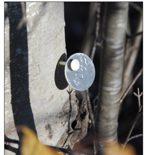
Upper left: A certified tree inspector hired by the project office measures the diameter of a tree in the Kenilworth Corridor. Lower left: Map of the survey area. Right: Trees over six inches in diameter are tagged and mapped by survey crews.
