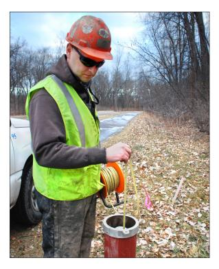
Left: As part of the water resources evaluation and ongoing ground water monitoring program, a technician inserts a ground water level indicator into one of the dozen piezometers placed in the Kenilworth Corridor.
