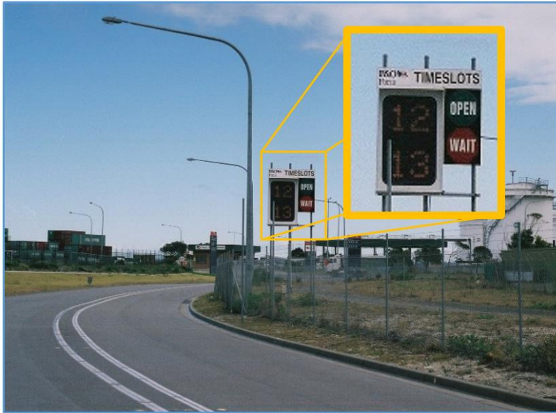
Figure 4-38. Truck Queuing System
