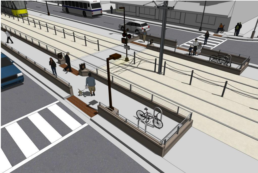
Figure 5-1 "Z-type" Pedestrian Crossing at Unsignalized Intersection
