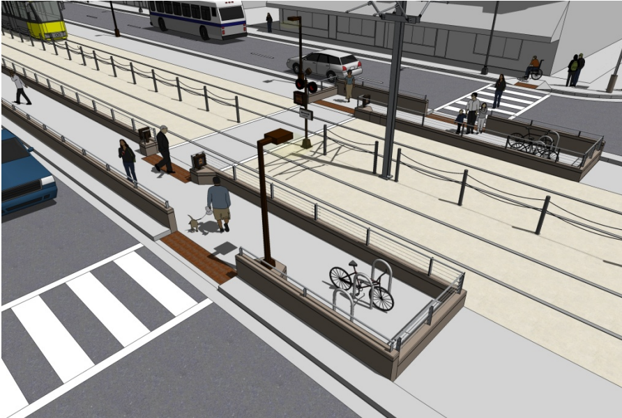
Figure 5-5 "Z-type" Pedestrian Crossing at Unsignalized Intersection
