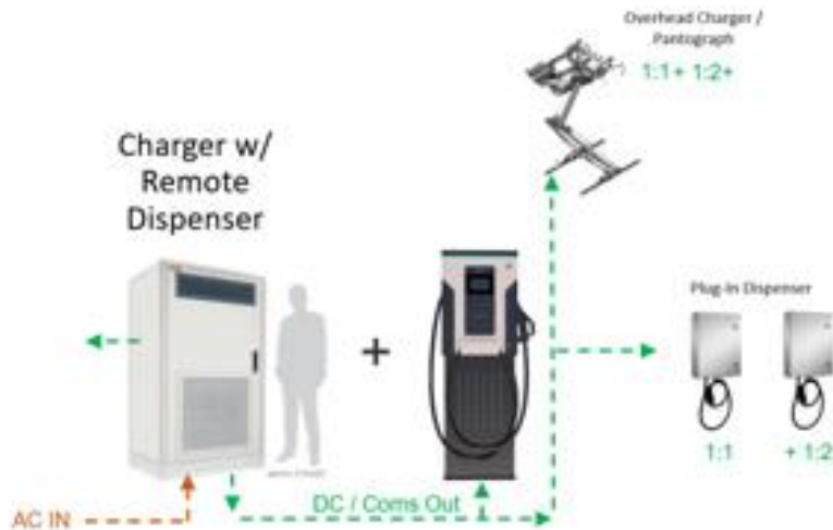
Figure 49: - Containerized 'Big Box' Charger
