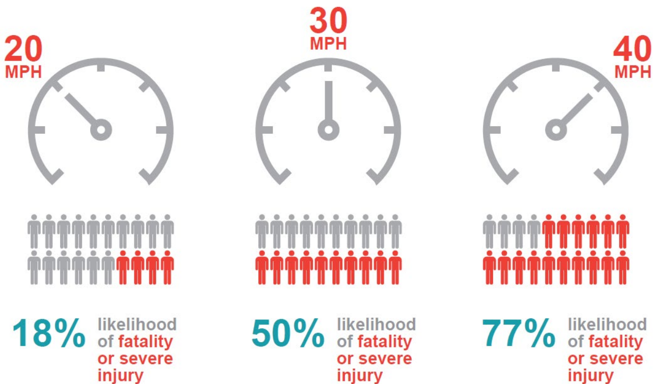
Figure 2: Impact Speed and a Pedestrian's Risk of Severe Injury or Death, Source: https://aaaafoundation.org/impact-speed-pedestrians-risk-severe-injury-death/
