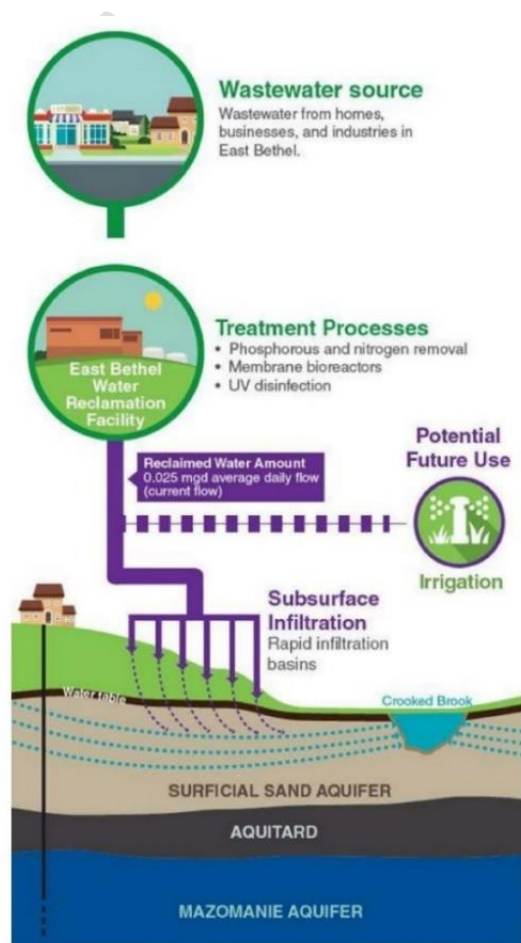
Figure 5: East Bethel water reclamation system
