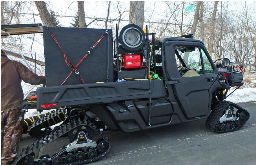
UTV equipped with tracks and CCTB equipment
