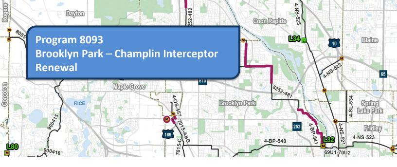
This Program provides for the rehabilitation concrete gravity interceptor in the Cities of Champlin, Brooklyn Park and Osseo. The interceptor will be rehabilitated using Cured-In-Place-Pipe (CIPP) technology.
