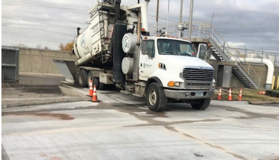
Vector truck discharging into a waste receiving facility
