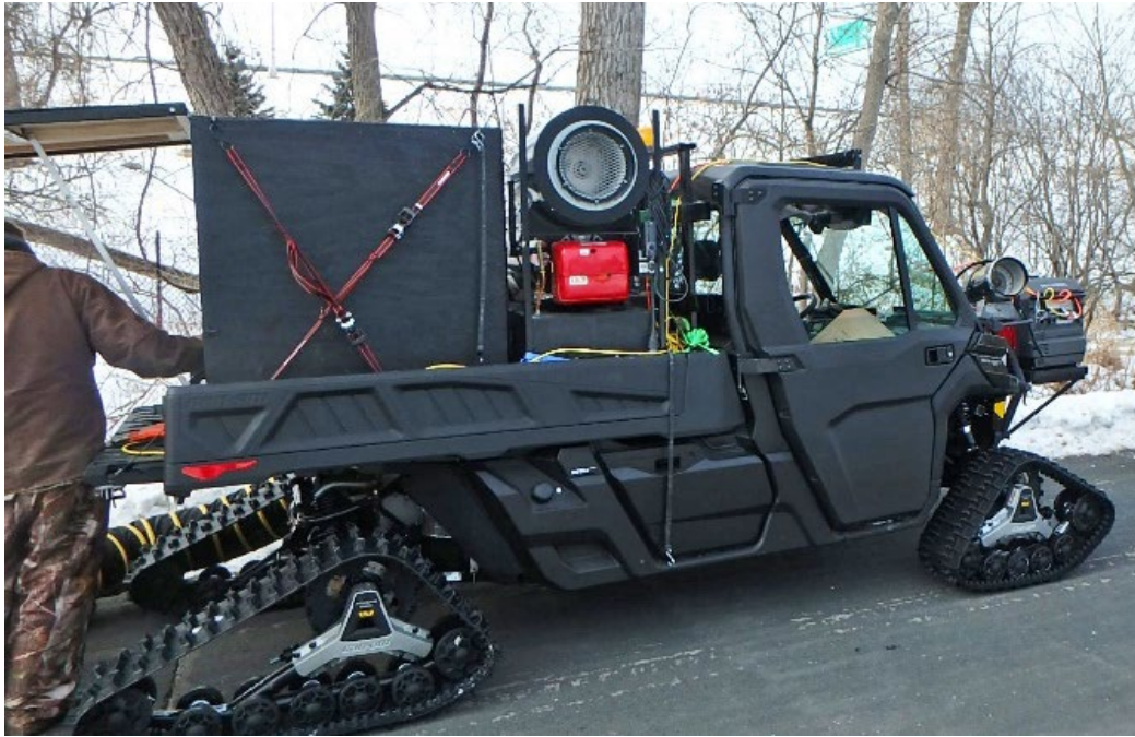
UTV equipped with tracks and CCTB equipment
