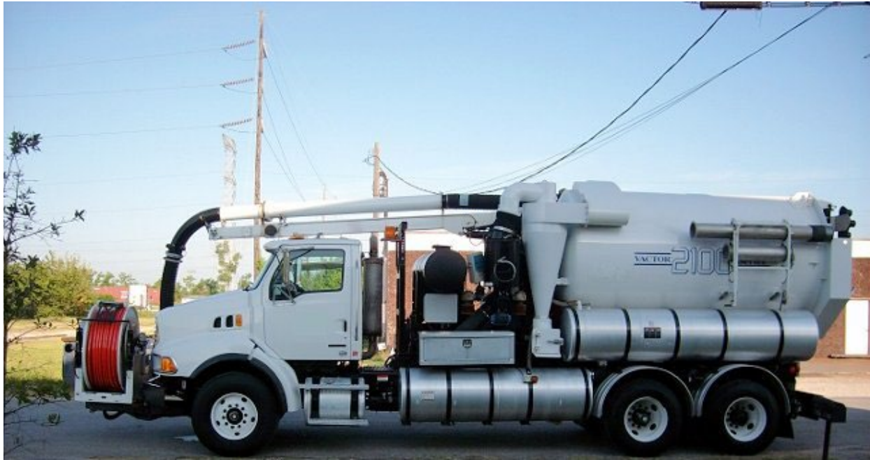
Vactor truck used to clean debris from interceptors
