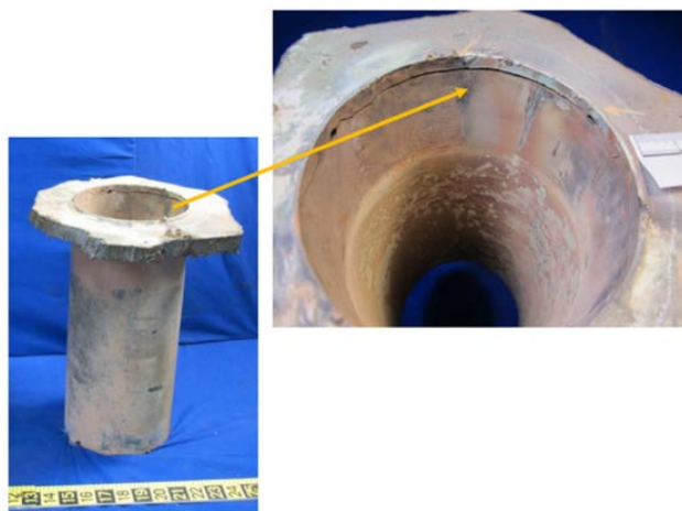
Photo 3. Cracking in the primary heat exchanger tubes at the tube sheet will cause the tubes to fall out of the tube sheet.
