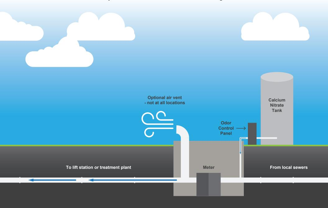
Chemical Odor Control system located below grade at MCES meter station (location dependent) **Optional air vent** - not at all locations Odor **Control Panel** Calcium **Nitrate** Tank To lift station or treatment plant Meter From local sewers
