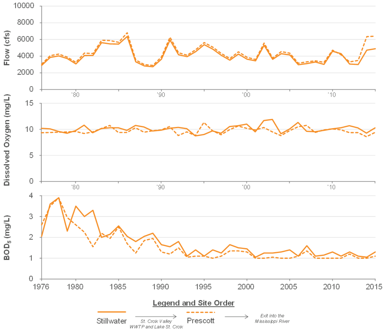
Figure 58. Annual Patterns of Median St. Croix River Flows and Concentrations of Dissolved Oxygen and BOD 5 , 1976-2015
