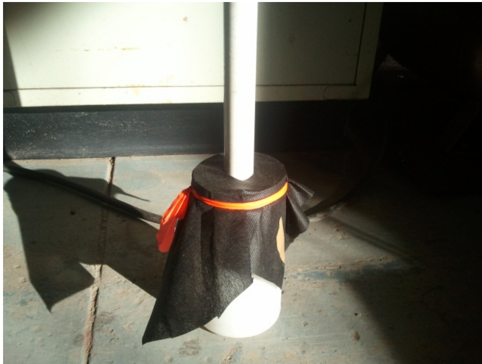
Figure 25. Illustration of the Nalgene bottle sampler arrangement set up for sampling stormwater and any infiltrated stormwater perched on the clay layer within the Hamline-Midway rain garden site. A similar bottle arrangement without the vertical access tube was used for sampling water on the surface of the basins at the Hamline-Midway and Sheep Pasture sites.
