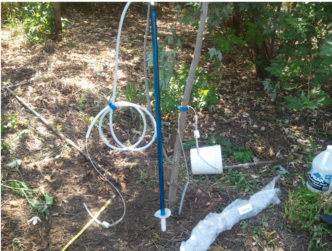
Figure 24. Decagon's SPE20 sampler (1 cm shaft) pore water sampler with a porous PE-nylon-membrane, which is especially suitable for heavy metals.
