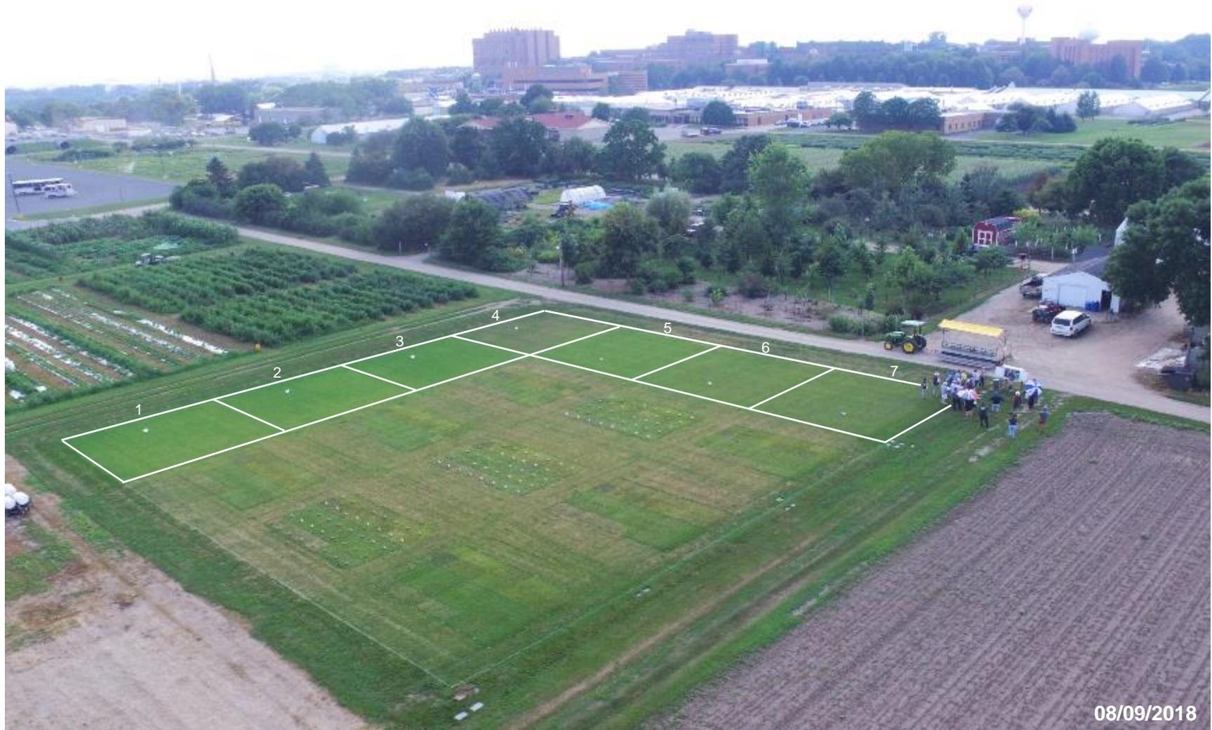
Figure 1. The project location at the turfgrass research farm on the UMN St. Paul campus. The irrigation treatments were a regular time-based irrigated control (1), the Hunter Hydrowise smart controller (2), the Rain Bird ESP-ME smart controller + rain sensor (3), a non-irrigated plot (4), the Toro Evolution smart controller (5), a manually-irrigated plot (6), and the Hunter Soil-Clik soil moisture sensor (7).
