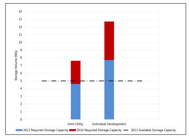
Figure 6.2 Required storage capacity for joint and individual development
