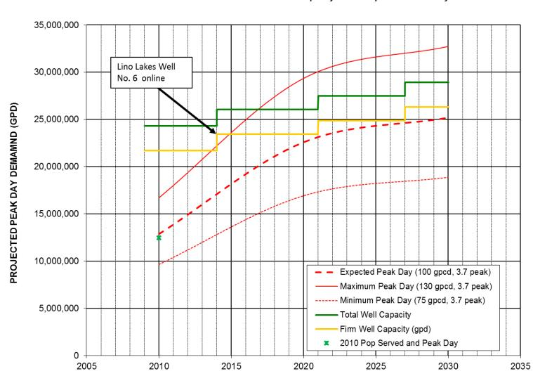
Figure A5 TRIGGER CHART WELL CAPACITY BY YEAR Ten State Standards 3.2.1.1: Firm well capacity should equal Maximum Day Demand
