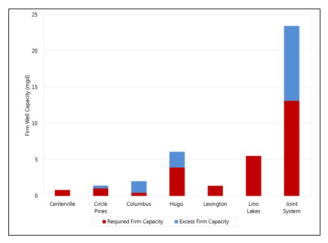
Figure 5.3 Required and excess firm well capacity for 2013 systems
