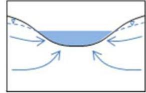
To facilitate the discussion of monitoring programs, a generalized hydrologic setting for a gaining stream is presented. The gaining stream is assumed to:
