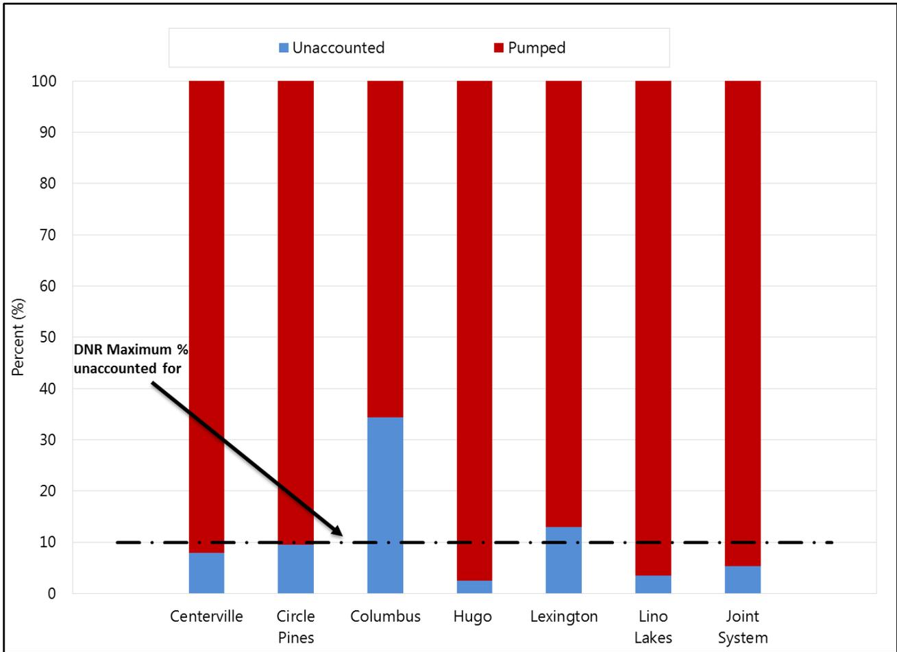
**Figure 5.1 Average percent of water pumped and water unaccounted for by city from 2009-2013**
