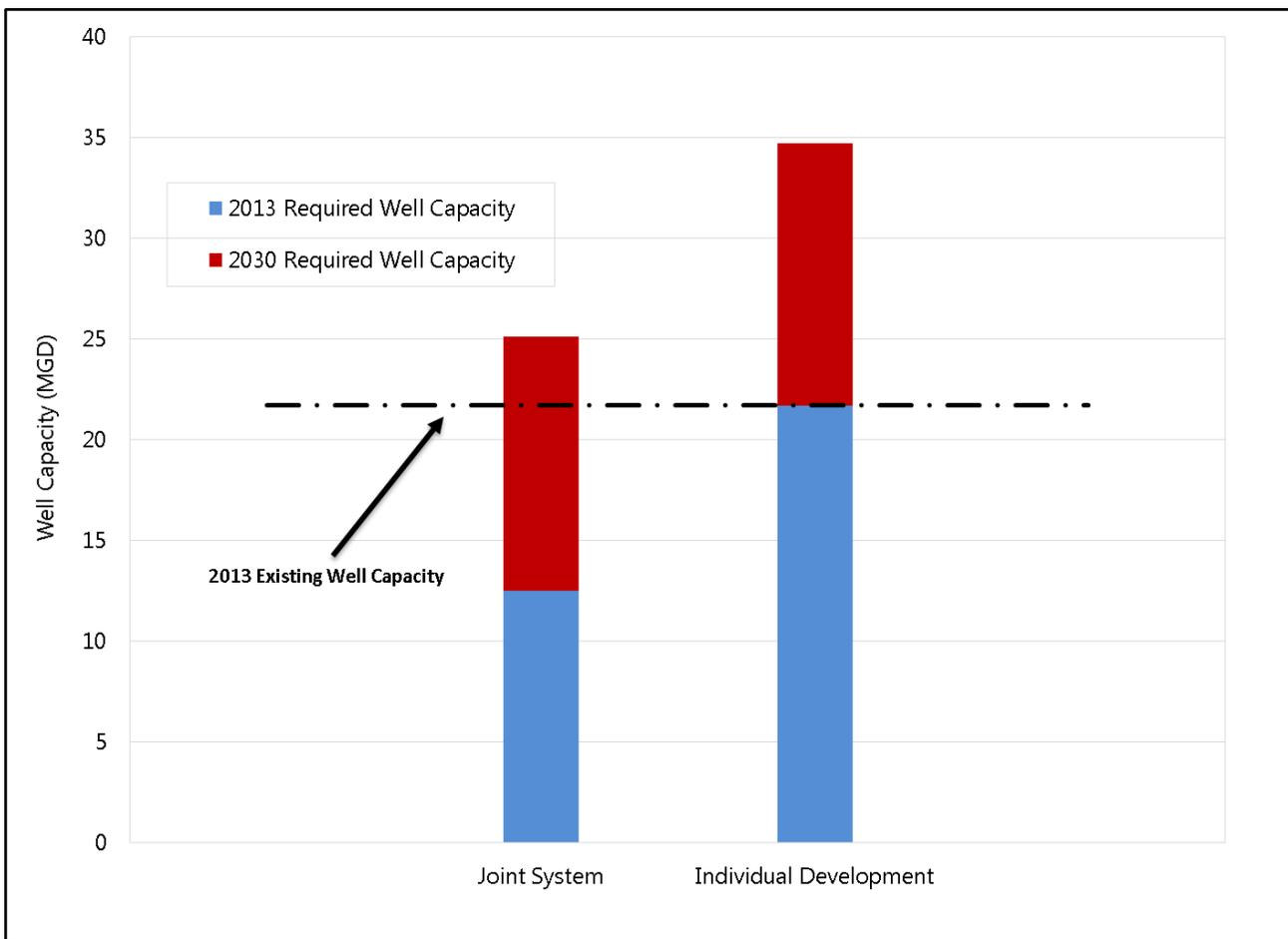
Figure 5.5 Existing and future well capacity requirements for joint and individual development
