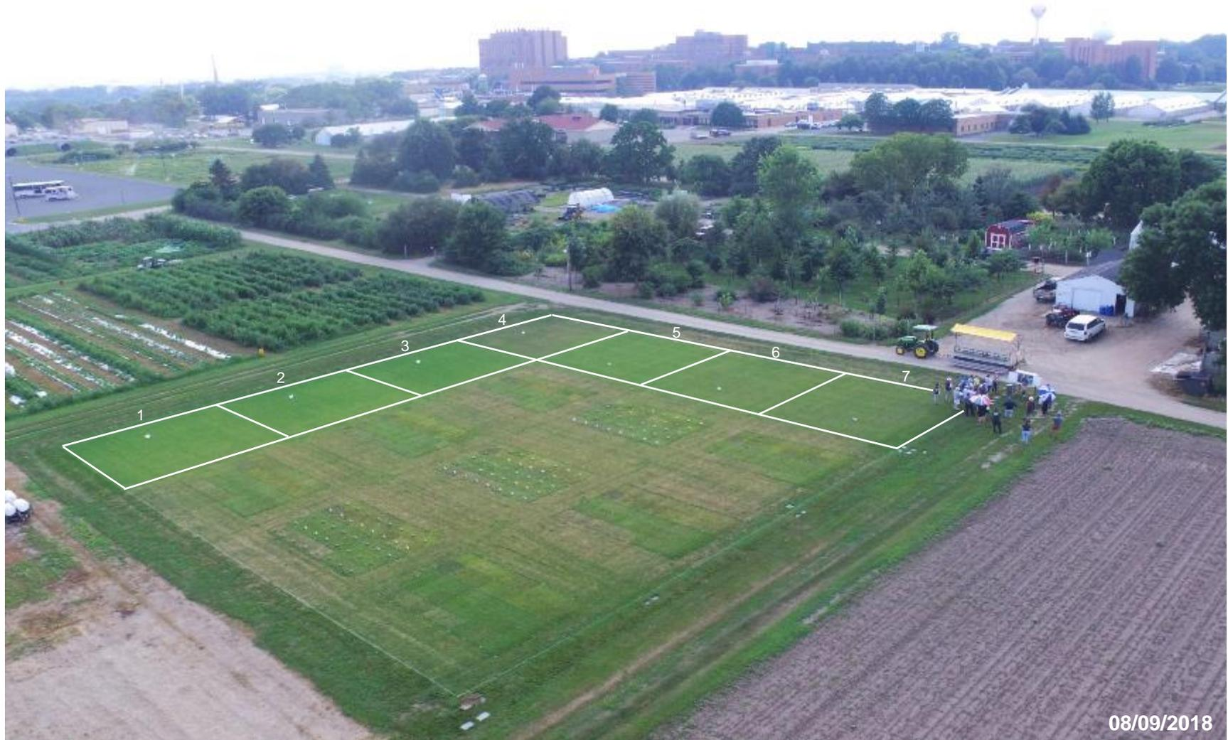
Figure 1. The project location at the turfgrass research farm on the UMN St. Paul campus. The irrigation treatments were a regular time-based Controller A (1), Smart Controller B (2), Smart Controller C + Rain Sensor (3), a non-irrigated plot (4), Smart Controller D (5), a manually-irrigated plot (6), and Soil Moisture Sensor + Controller F (7).
