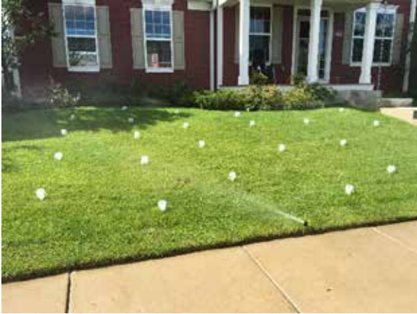
Figure 32: Catch can test used to measure rotor and fixed spray uniformity
