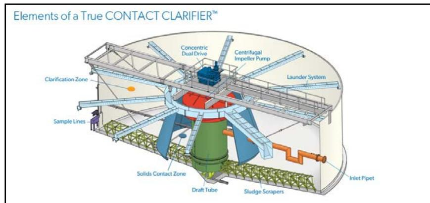
the solids collected at the bottom of the clarifier is recirculated and serves as a seed for coagulation/precipitation process with the raw water in the contact zone.
