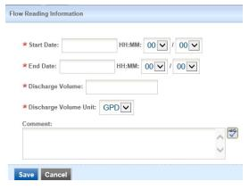
Enter "Start Date" and "End Date" and times. These dates need to match the start and end dates from the monitoring event. Next enter the "Discharge Volume." The discharge volume is the volume of discharge through the monitoring point during the monitoring event. This value is NOT the volume of the sample collected. The volume reported should be in gallons. Add any comments, if applicable, and click the "Save" button.
