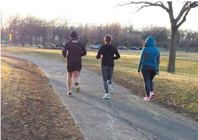
An 8' trail width accommodates three pedestrians traveling side-by-side in the same direction. Pedestrians may adjust their position off-trail when passing.
