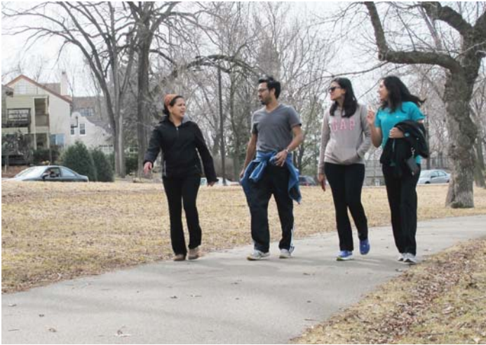
A 10' trail width accommodates four pedestrians traveling side-by-side in the same direction. Pedestrians may adjust their position off-trail when passing.
