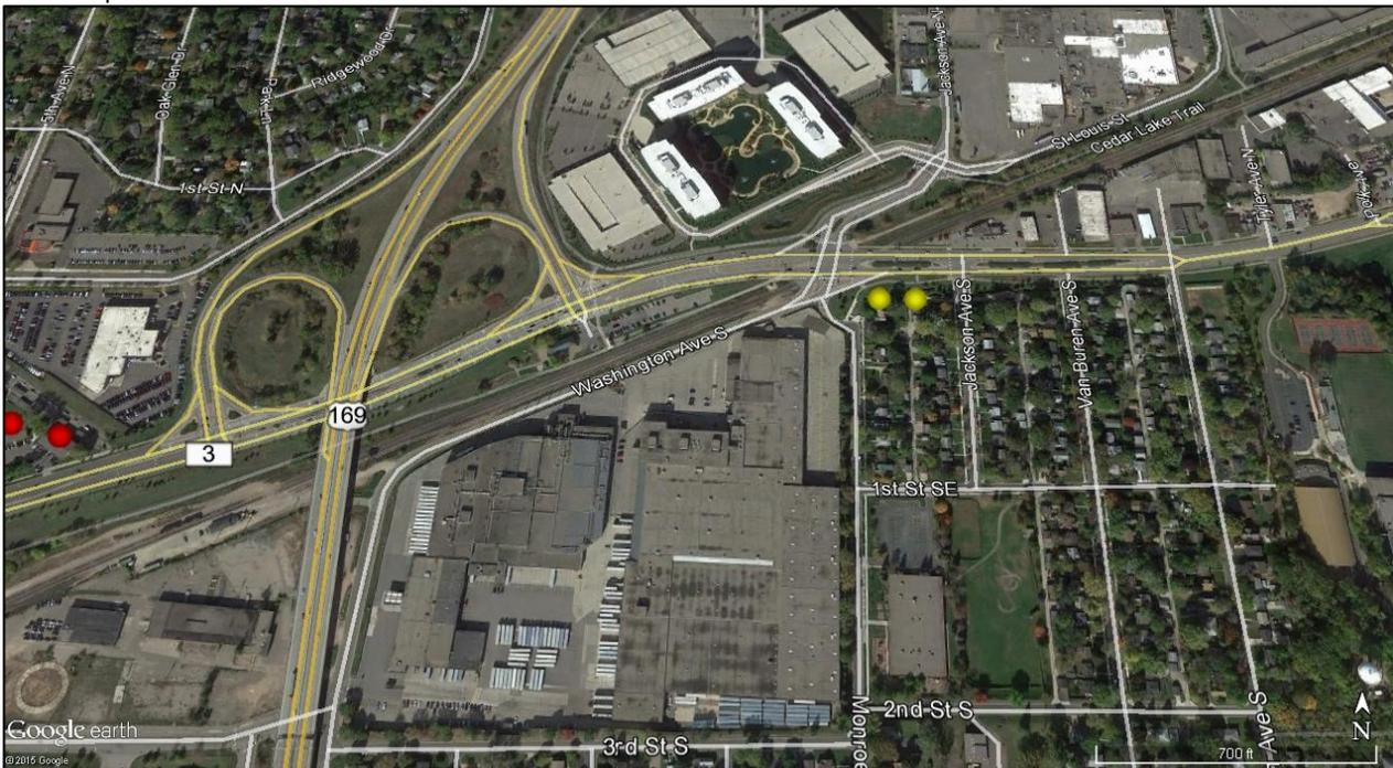
\* Red dots indicate severe noise impacts and yellow dots indicate moderate noise impacts
