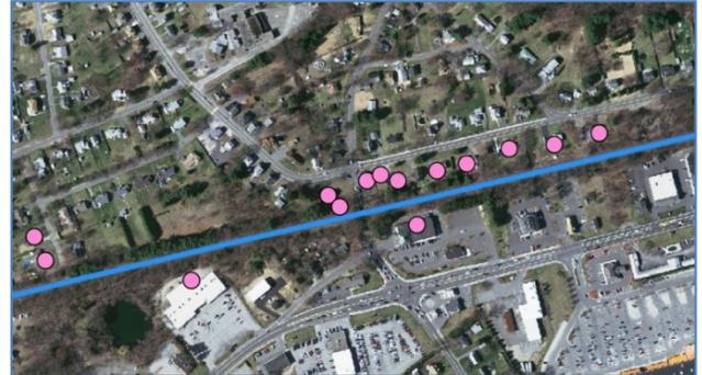
The output of a vibration or GBN impact assessment includes locations with vibration or GBN impact (purple). This information is used to determine the location and extent of any potential vibration mitigation.
