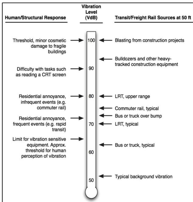
Ground-borne noise (GBN) is also assessed. GBN is a form of low-frequency noise that radiates from building walls and ceilings due to vibration caused by
