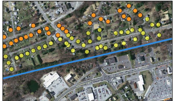
The output of a noise impact assessment includes locations with Severe Impact (yellow) and Moderate Impact (orange). This information is used to determine the location and extent of any potential noise mitigation.
