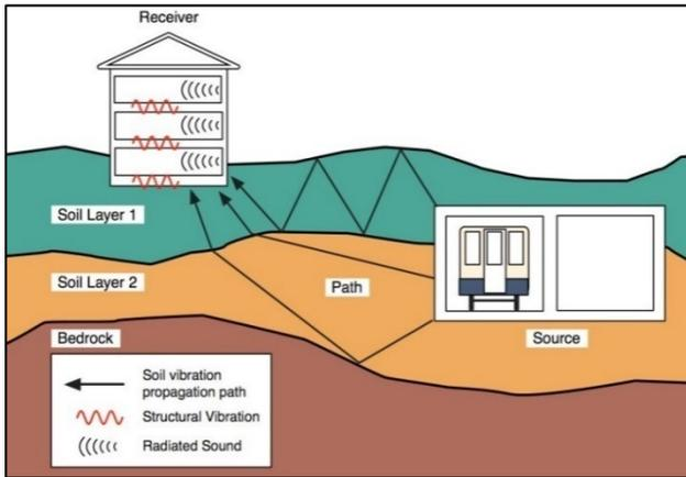
Vibration and GBN impact assessments are based on applicable FTA and Federal Railroad Administration (FRA) models, and are assessed using the source-path-receiver framework. Some of the key components of a vibration impact assessment include:
