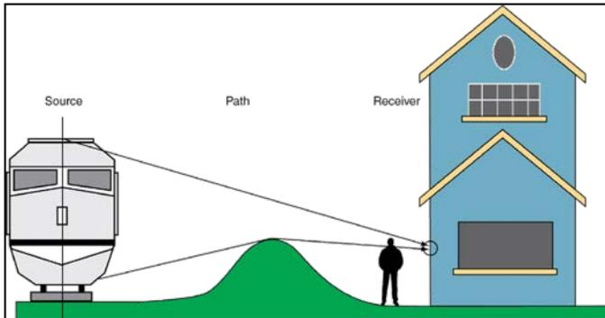
Noise impact assessments are based on applicable FTA and Federal Railroad Administration (FRA) models, and are assessed using the source-path-receiver framework. Some of the key components of a noise impact assessment include:
