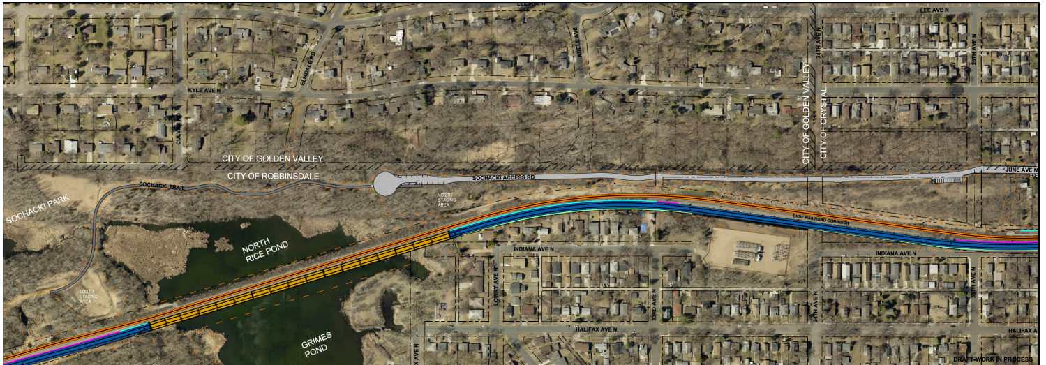
Plan sheet showing where the light rail track (blue) will go and where sidewalk and access road (gray) improvements will be made in Sochacki park
