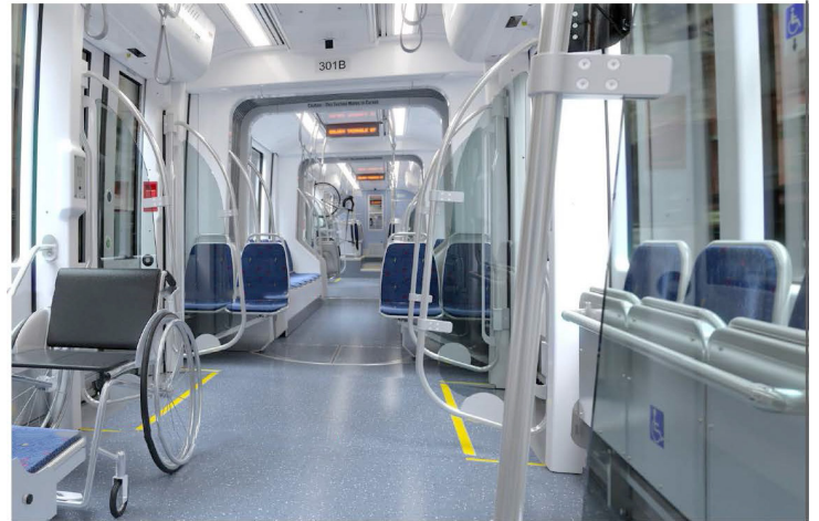
Light rail vehicle design includes space for passengers in wheelchairs and companion seating.
