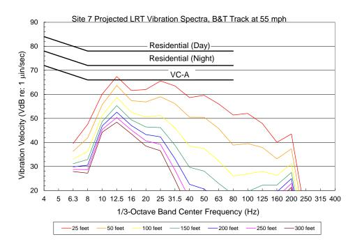
Figure E-7. Site 7 Projected LRT Vibration Spectra on B&T Track at 55 mph Source: Harris Miller Miller & Hanson Inc., 2012
