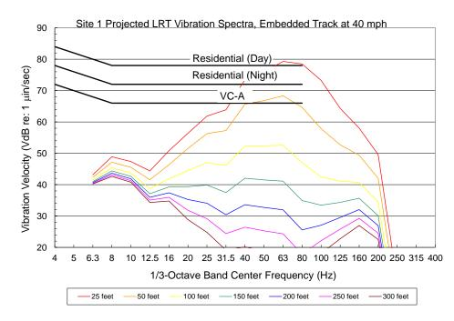
Figure E-9. Site 1 Projected LRT Vibration Spectra on Embedded Track at 40 mph Source: Harris Miller & Hanson Inc., 2012
