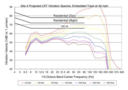
Figure E-12. Site 4 Projected LRT Vibration Spectra on Embedded Track at 40 mph Source: Harris Miller & Hanson Inc., 2012
