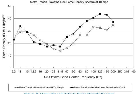
Figure 8. Metro Transit Vehicle Force Density Spectra Source: Harris Miller Miller & Hanson Inc., 2012.
