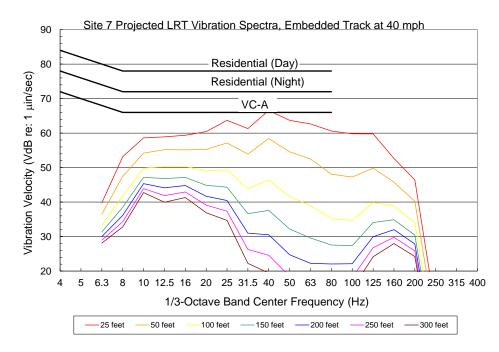
Figure E-15. Site 7 Projected LRT Vibration Spectra on Embedded Track at 40 mph Source: Harris Miller Miller & Hanson Inc., 2012
