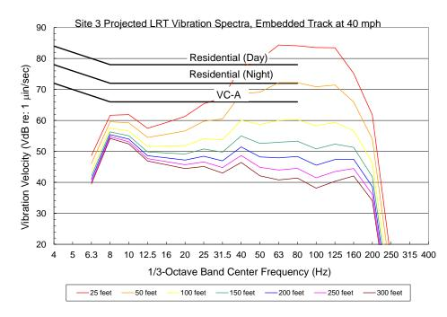
Figure E-11. Site 3 Projected LRT Vibration Spectra on Embedded Track at 40 mph Source: Harris Miller Miller & Hanson Inc., 2012
