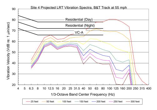
Figure E-4. Site 4 Projected LRT Vibration Spectra on B&T Track at 55 mph Source: Harris Miller Miller & Hanson Inc., 2012
