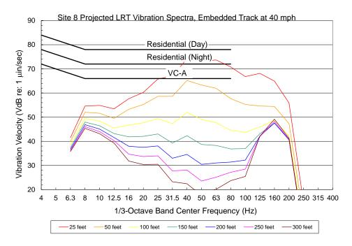
Figure E-16. Site 8 Projected LRT Vibration Spectra on Embedded Track at 40 mph Source: Harris Miller Miller & Hanson Inc., 2012
