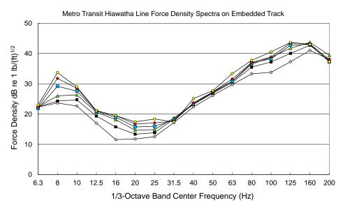
Figure D-2. Metro Transit Reference LRV Force Density Levels on Embedded Track Source: ATS Consulting, 2008
