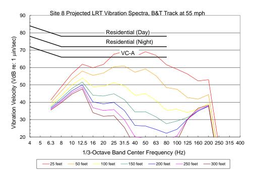
Figure E-8. Site 8 Projected LRT Vibration Spectra on B&T Track at 55 mph Source: Harris Miller Miller & Hanson Inc., 2012
