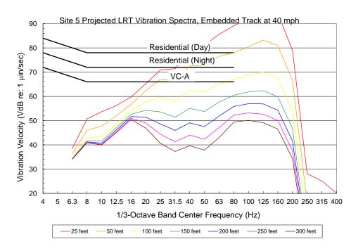
Figure E-13. Site 5 Projected LRT Vibration Spectra on Embedded Track at 40 mph Source: Harris Miller Miller & Hanson Inc., 2012
