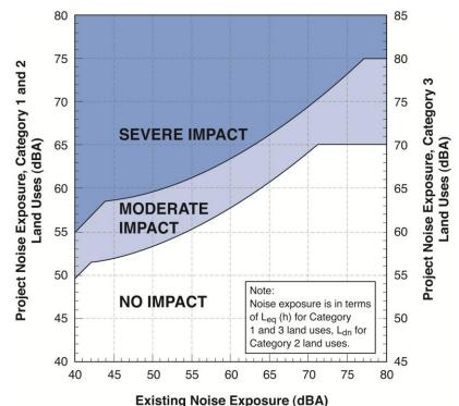
Figure 2. FTA Noise Impact Criteria Comparing Existing Noise to Project Noise Source: Federal Transit Administration, 2006.
