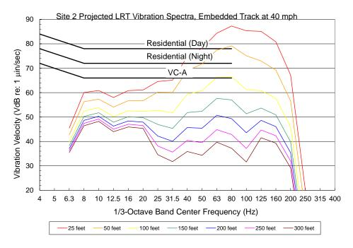
Figure E-10. Site 2 Projected LRT Vibration Spectra on Embedded Track at 40 mph Source: Harris Miller & Hanson Inc., 2012
