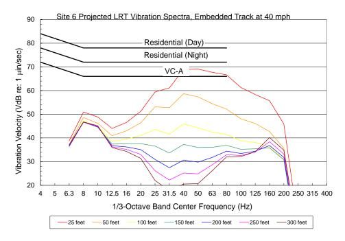
Figure E-14. Site 6 Projected LRT Vibration Spectra on Embedded Track at 40 mph Source: Harris Miller & Hanson Inc., 2012
