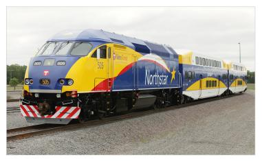
Northstar commuter rail trains, like the one shown on the right above, are pulled by large diesel-electric locomotives and operate over longer distances with fewer stops. Commuter rail trains share track with freight rail service.
