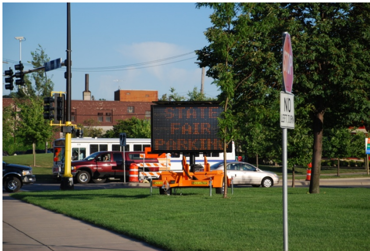
VMS used to alert drivers to State Fair parking off the newly reconstructed University of Minnesota transitway
