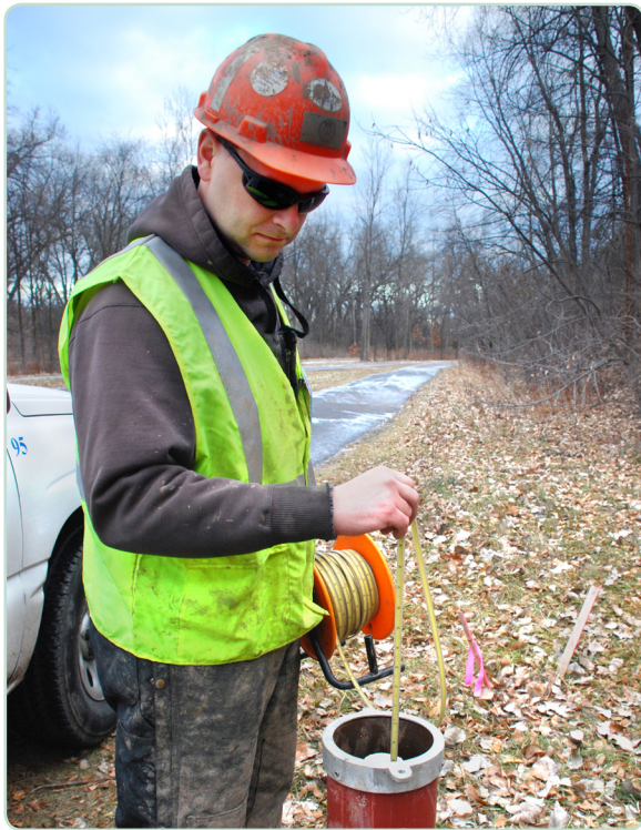
A technician inserts a ground water level indicator at one of several monitoring stations in the Kenilworth area.
