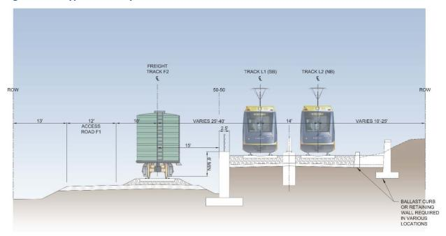
Figure 3-2c. Typical Railway Section – Wall Corridor Protection
