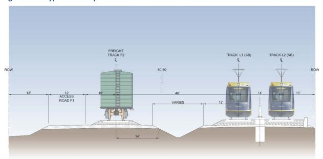
Figure 3-2a. Typical Railway Section – Ditch Corridor Protection
