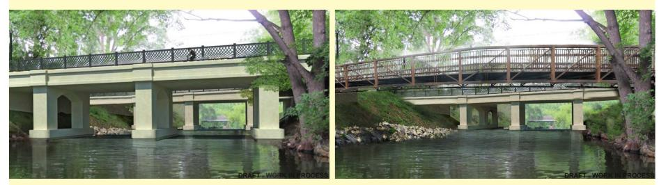
Modified SPO bridge Concrete arched in-channel piers Pedestrian and bicycle bridge Vaulted steel structure, no inchannel piers
