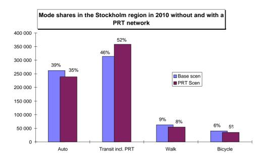
The number of auto trips is calculated to be reduced by 9 % in the peak period, with its dramatic and positive impacts in terms of reduced congestion, air pollution and road traffic accidents. Transit trips – including the new PRT mode – is forecast to expand by almost one third (31%) during all day, and by 41 % in the off-peak period:
