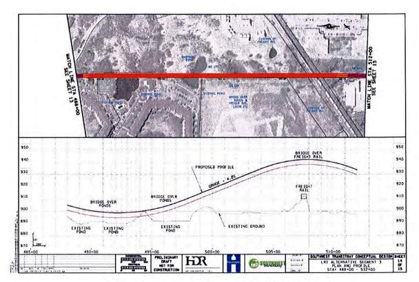
Figure 2 - Elevation of track in SDEIS Appendix F
