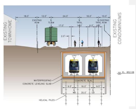
Diagram B – Typical Kenilworth Shallow LRT Tunnel Section per SDEIS
