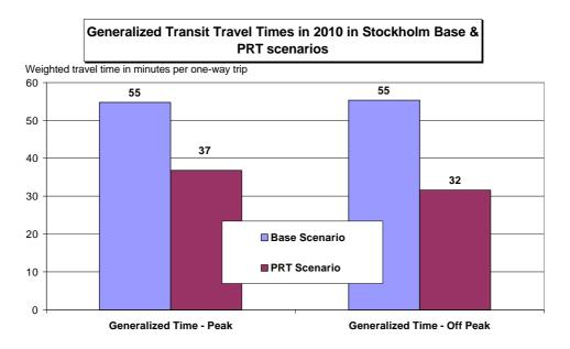
If an *area-wide PRT system* would be introduced in all Stockholm region, a substantial modal shift from the auto mode (-4 % units) would occur; also a slight shift from the walk and bike modes towards the transit modes, including the new area-wide PRT-system.
