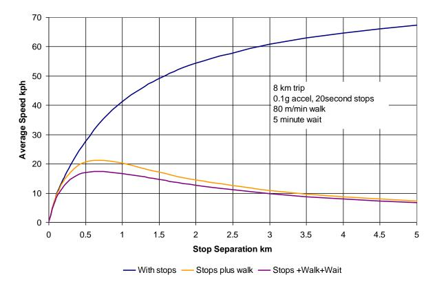
Figure 4 Overall Average Speed for Conventional Transport vs Stop Separation
